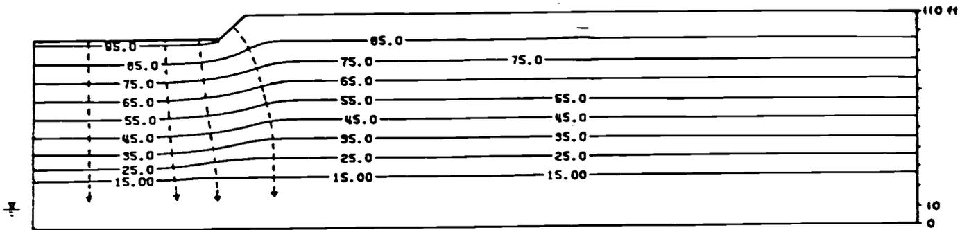
b) Total head distribution after 5 hours of simulation.
