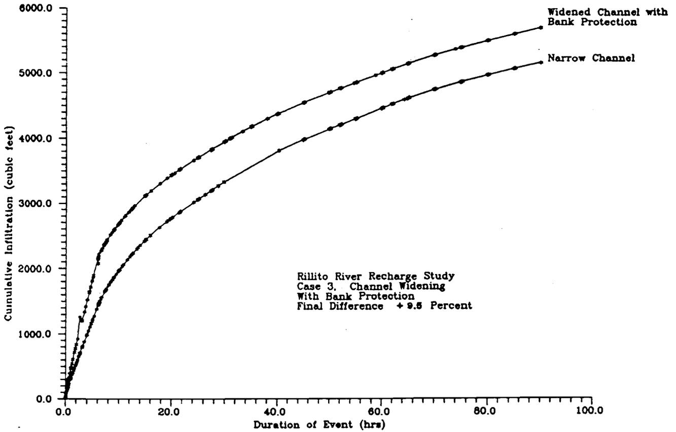
Figure 13. Difference in cumulative infiltration for case 3: channel widening with bank protection.
