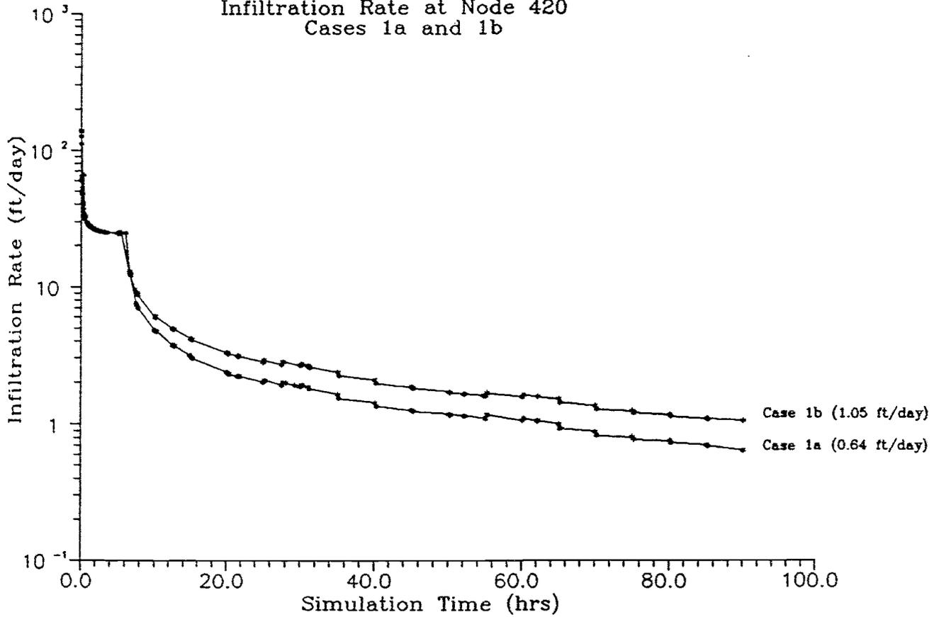
Figure 1. Infiltration rate at node 420 for case 1 (wide channel) before and after bank protection.
