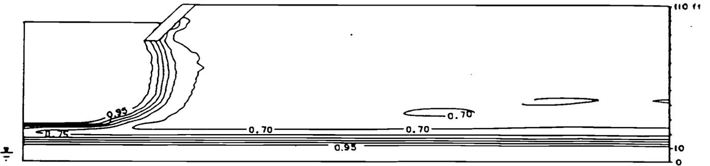
b) Degree of saturation after 5 hours of simulation.
