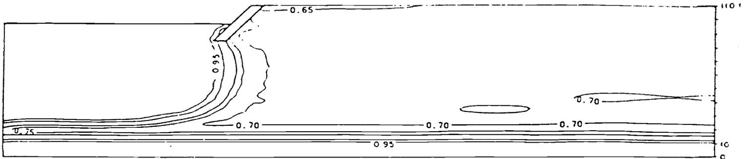
b) Degree of saturation after 5 hours of simulation.
