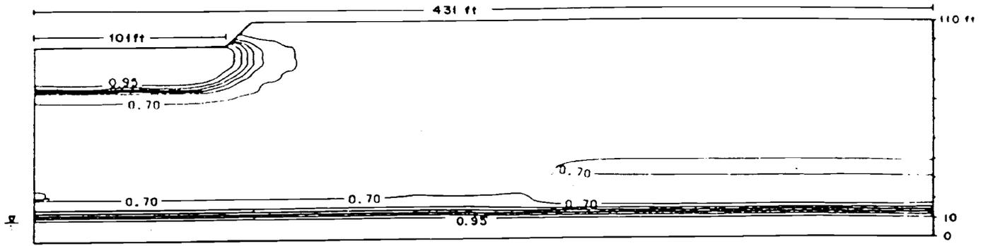
a) Degree of saturation after 1 hour of simulation.
