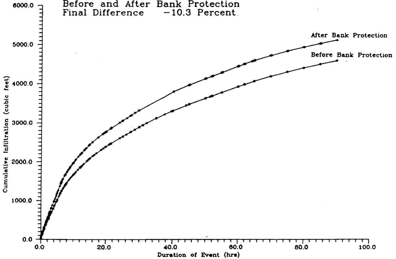
Figure 8. Difference in cumulative infiltration for case 2 (narrow channel) before and after bank protection.
