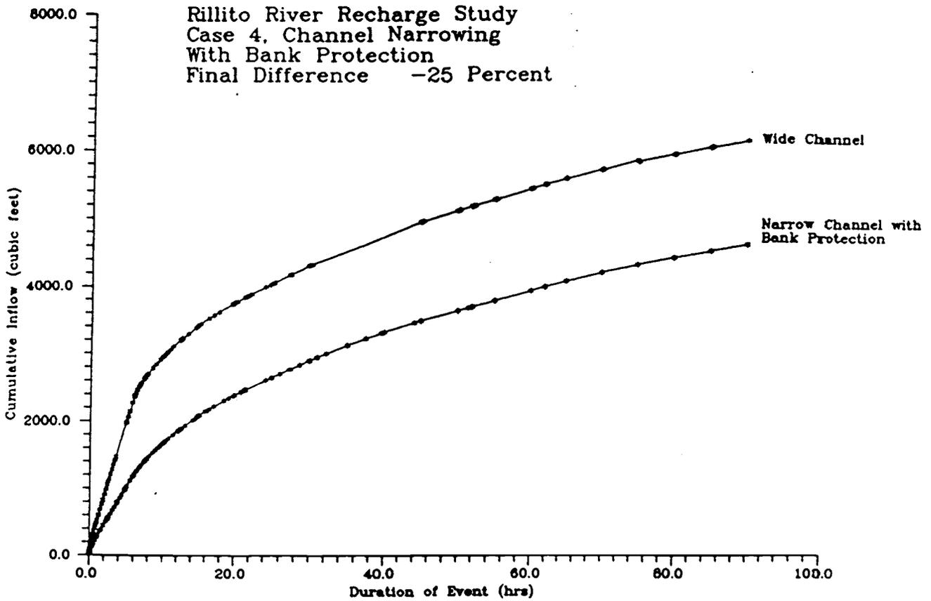
Figure 14. Difference in cumulative infiltration for case 4: channel narrowing with bank protection.
