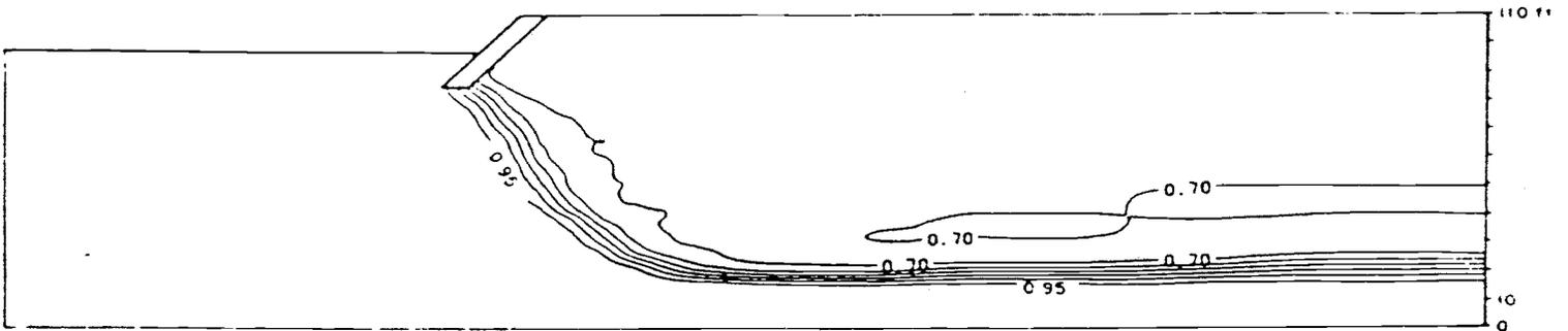
c) Degree of saturation after 10 hours of simulation.
