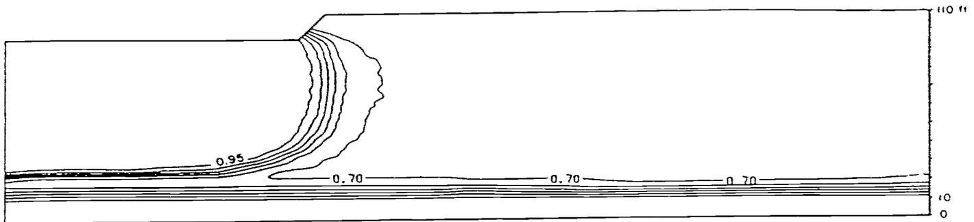
b) Degree of saturation after 5 hours of simulation.
