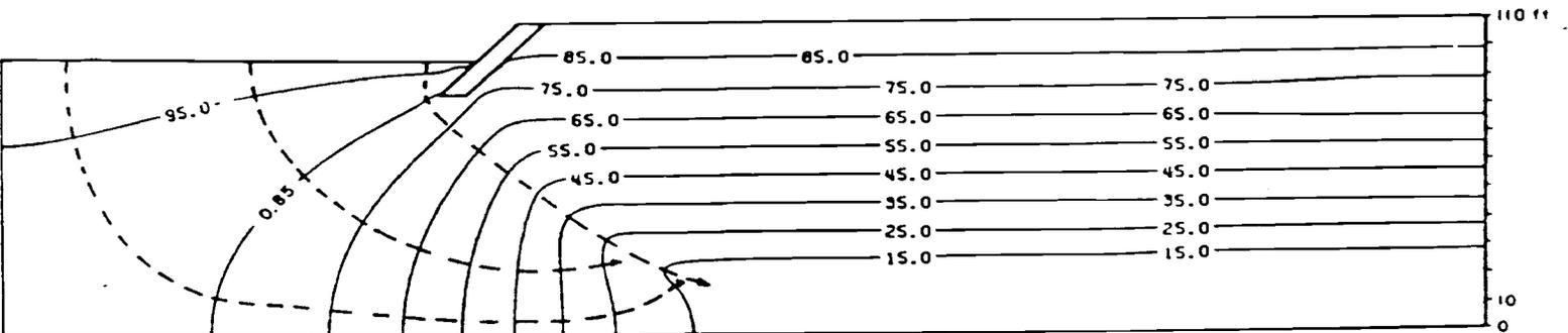
c) Total head distribution after 10 hours of simulation.
