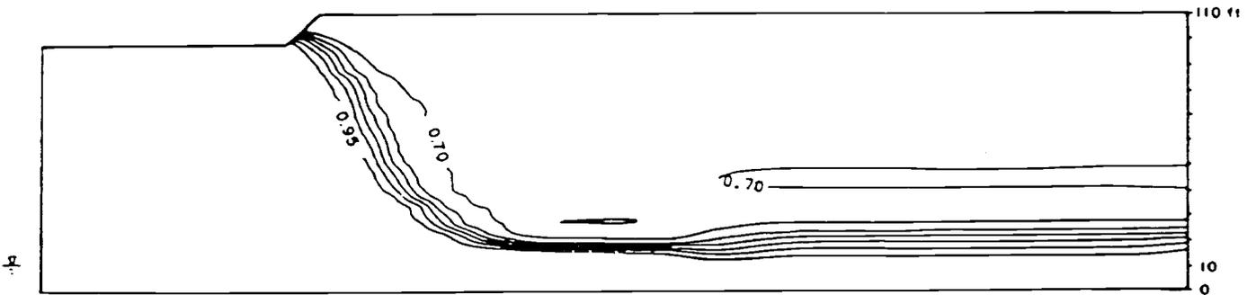
c) Degree of saturation after 10 hours of simulation.
