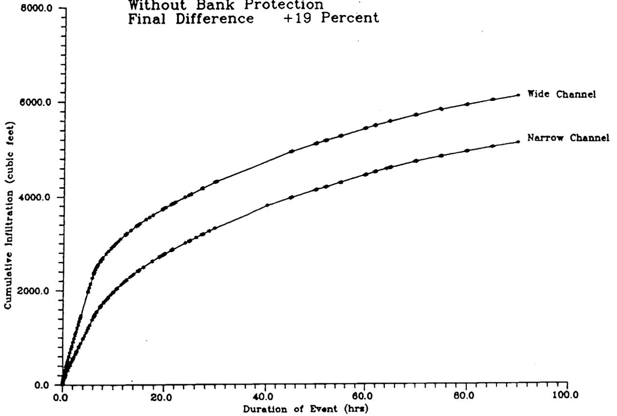
Figure 15. Difference in cumulative infiltration for case 5: channel widening without bank protection.
