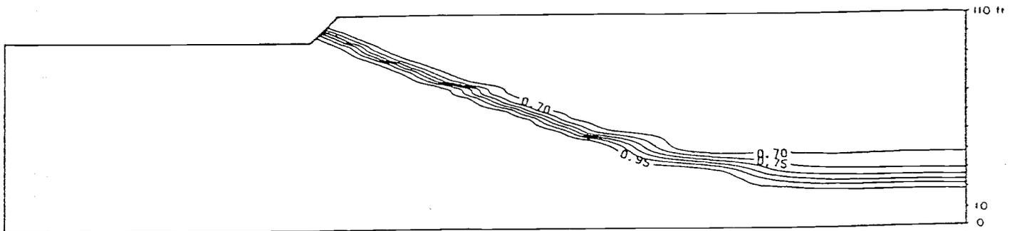
d) Degree of saturation after 25 hours of simulation.
