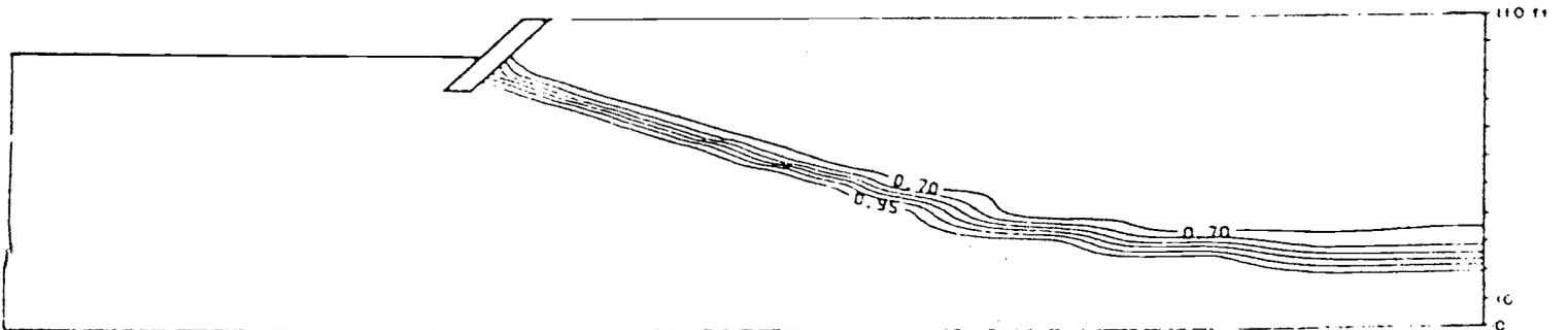
d) Degree of saturation after 25 hours of simulation.
