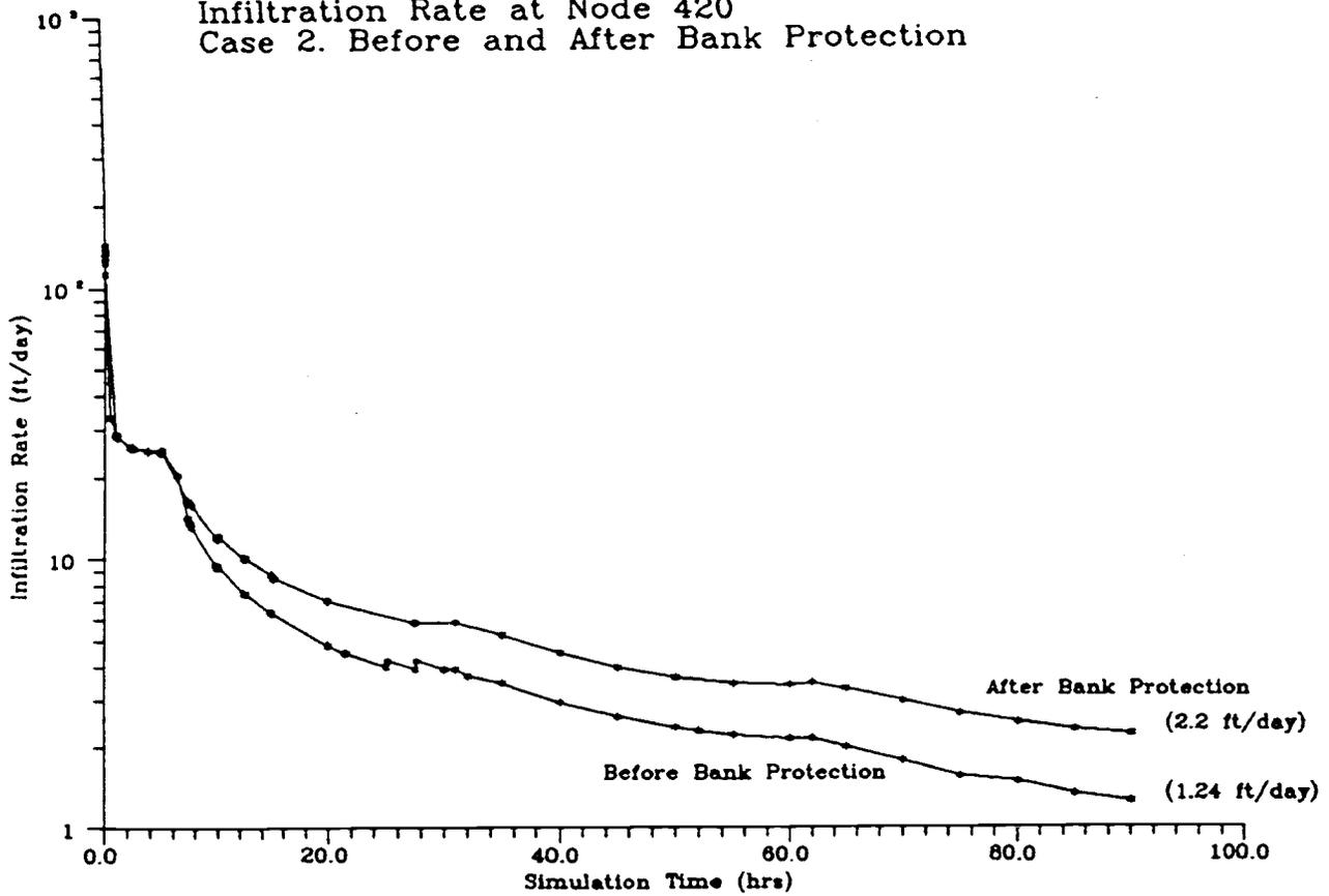
Figure 7. Infiltration rate at node 420 for case 2 (narrow channel) before and after bank protection.
