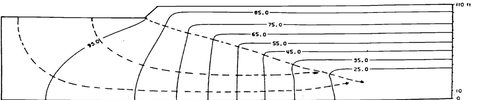
d) Total head distribution after 25 hours of simulation.
