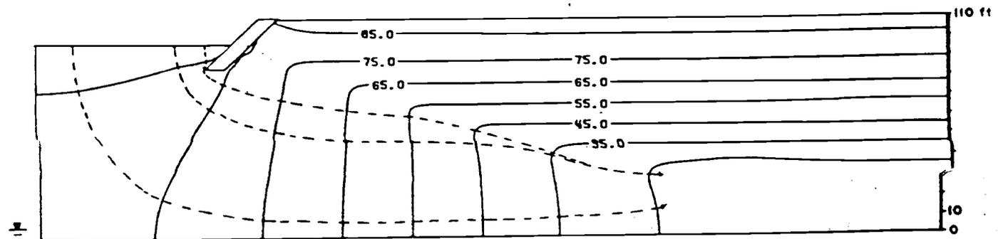
d) Total head distribution after 25 hours of simulation.
