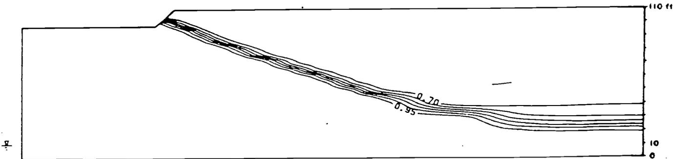
d) Degree of saturation after 25 hours of simulation.
