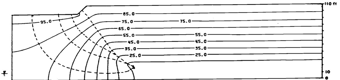
c) Total head distribution after 10 hours of simulation.
