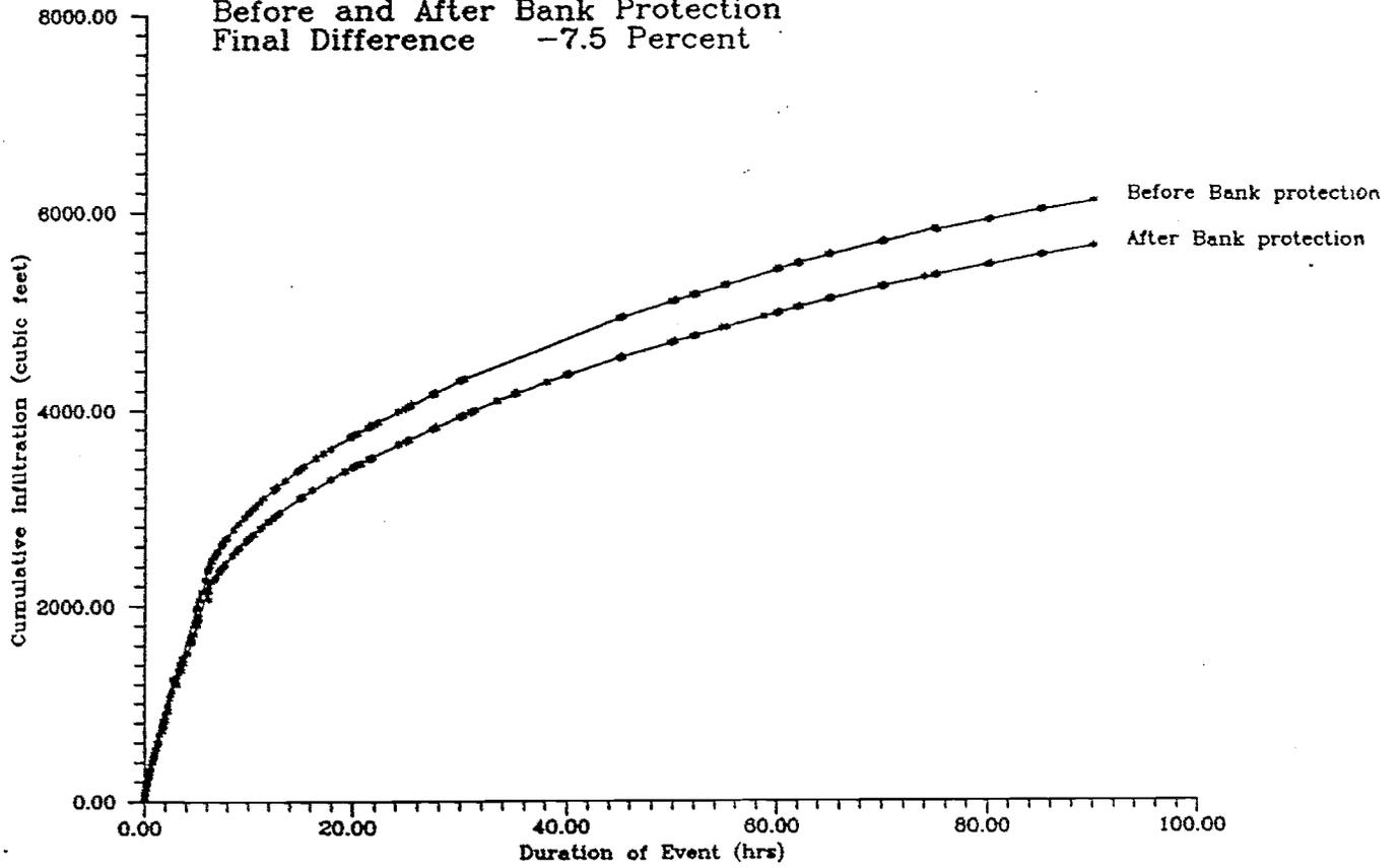
Figure 2. Difference in cumulative infiltration for case 1 (wide channel) before and after bank protection.
