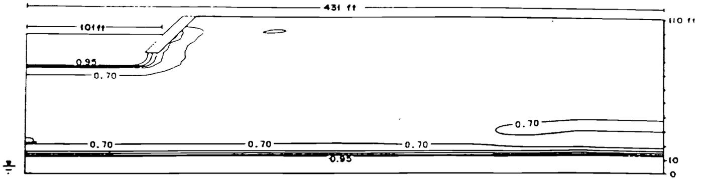
a) Degree of saturation after 1 hour of simulation.
