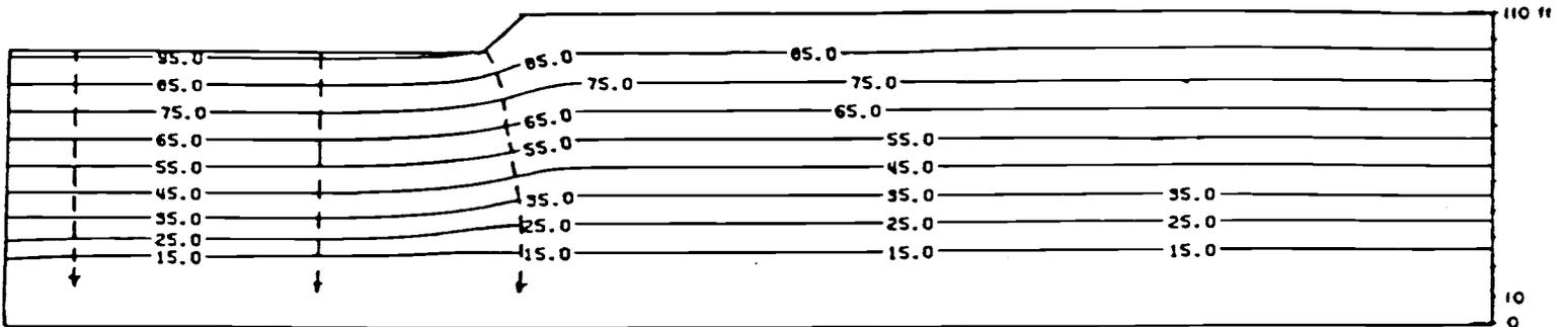
b) Total head distribution after 5 hours of simulation.
