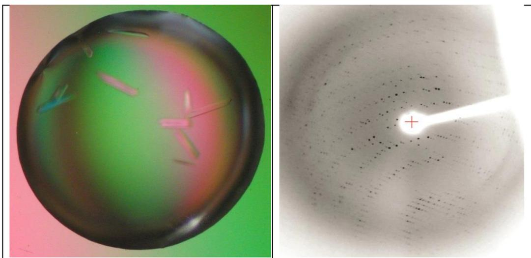
Figure 4.10: (left) Crystals of Mk0566 and (right) the diffraction pattern obtained from the crystals after being shot by the x-ray beam.
