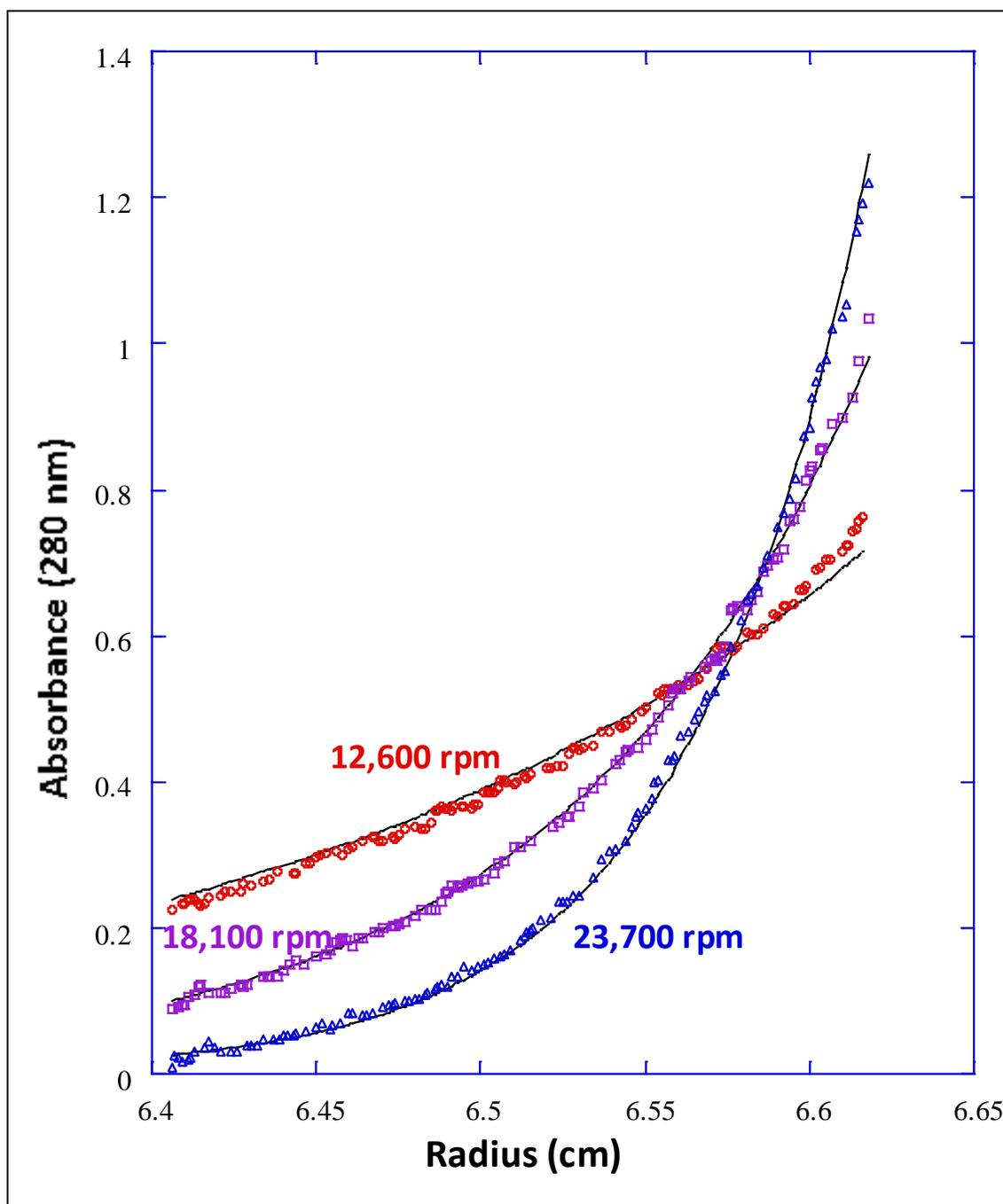
Figure 4.9: Sedimentation equilibrium of Mk0566 using analytical ultracentrifugation. Molecular weight obtained by global fitting was 39,471 g/mol and the enzyme was in monomeric form in absence of DNA. Figure courtesy of Dr. Chad K. Park, Analytical Biophysics Core Facility.
