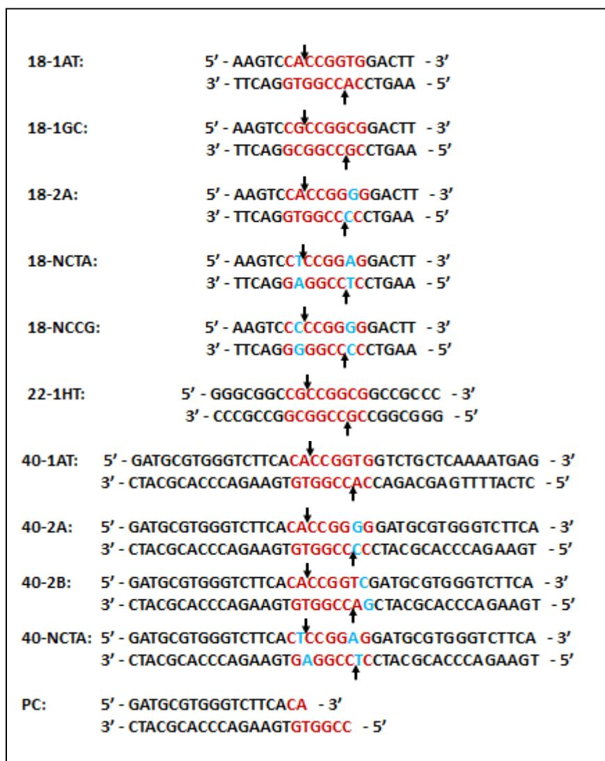
Table 2.8: DNA constructs used in determining dissociation constants, cleavage rate constants and crystal structure. Recognition sequences are shown in red, whereas the variations in secondary site sequences are shown in cyan. Arrows indicate the cleavage sites.
