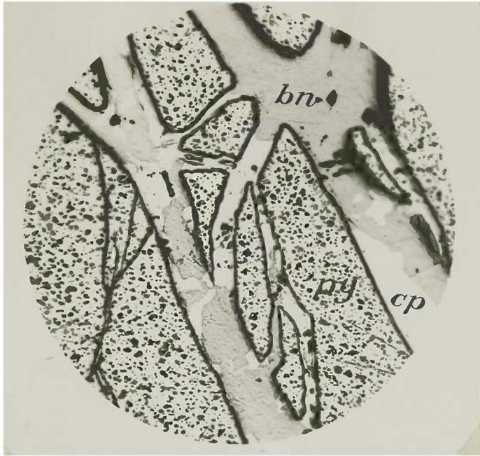
Pyrite (py) fractured and filled by veins of chalcopyrite (cp), and these in turn replaced by bornite (bn).
