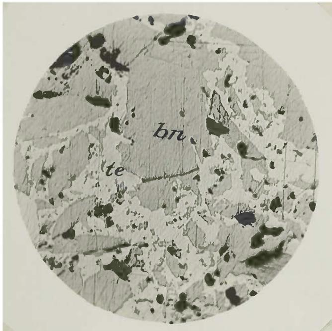
Tetrahedrite (te) and bornite (bn) intergrown and suggesting contemporaneous deposition.
