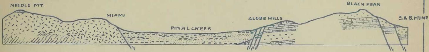
DIAGRAMMATIC SECTION SHOWING GRABEN STRUCTURE OF PINAL VALLEY
