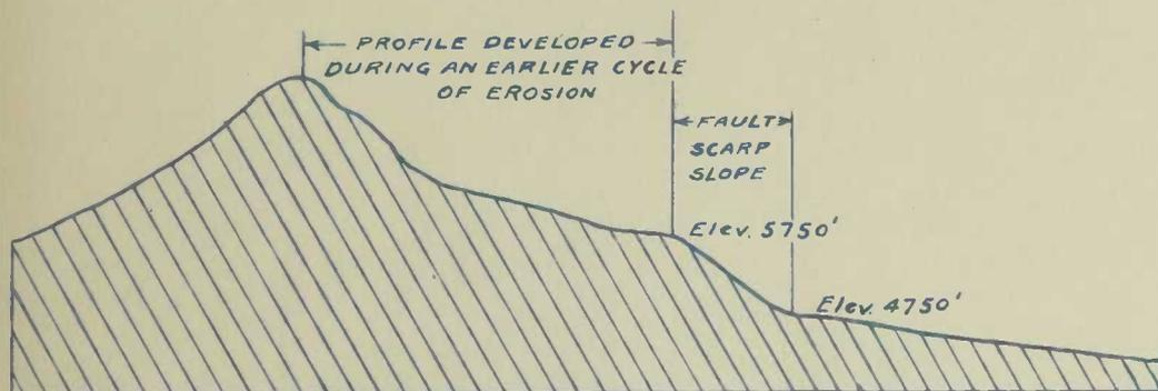
SECTION UP ICEHOUSE CANYON SHOWING LOW GRADIENT OF STREAM BED ABOVE FAULT SCARP
