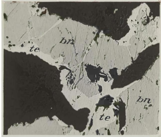
Bornite (bn) veined and replaced by tetrahedrite (te). Black is calcite gangue with pits.
