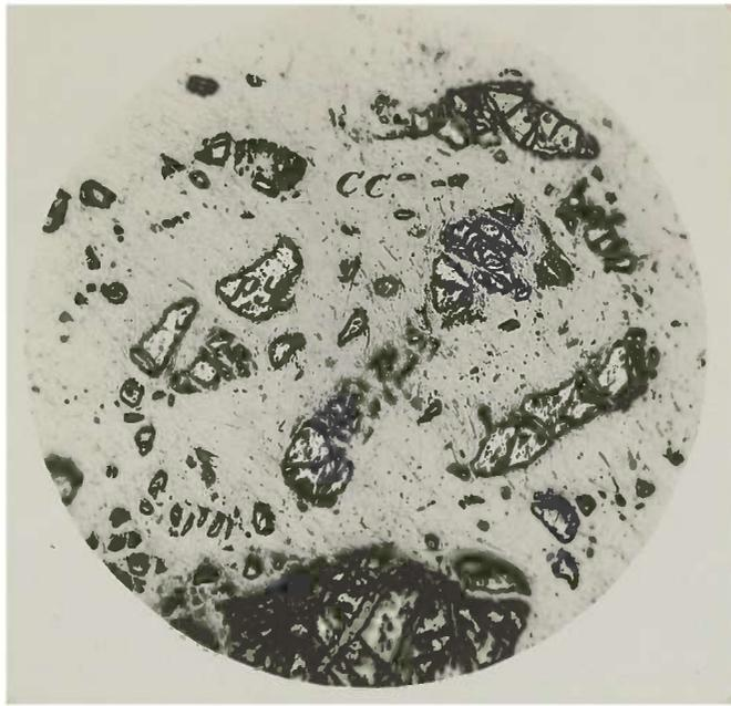
Pyrite (py) almost entirely replaced by chalcocite (cc). Note bomb structure.
