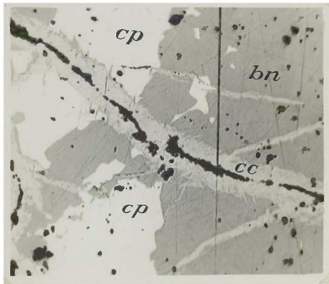
Chalcopyrite (cp) replaced by secondary bornite (bn). Chalcocite (cc) veins replacing chalcopyrite and rimmed with bornite. Replaces bornite direct. Black gangue.
