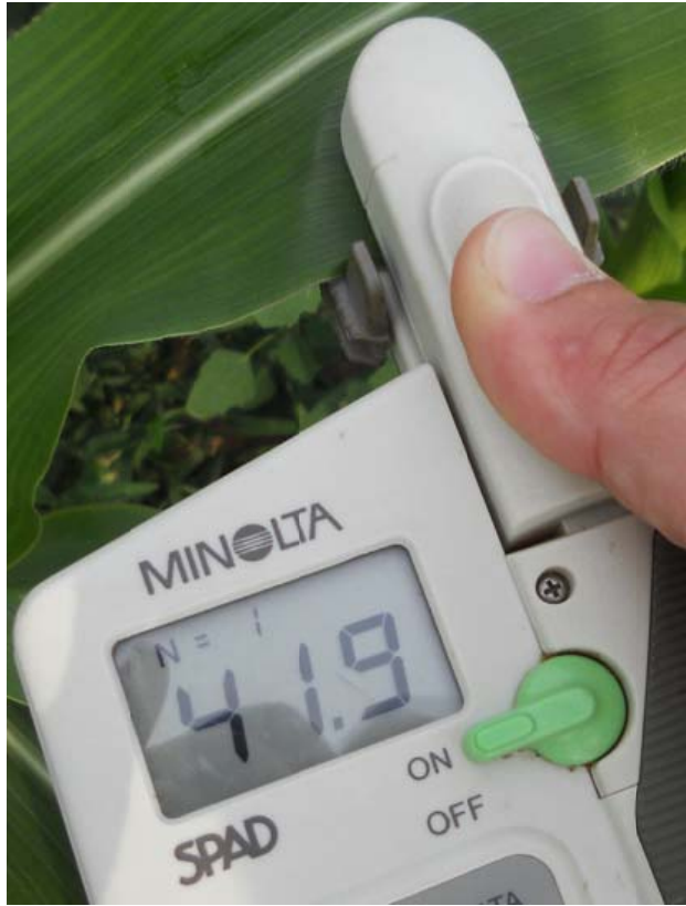
Fig. 3. Placement of SPAD meter, between the midrib and the edge of the leaf, for corn chlorophyll measurements.
