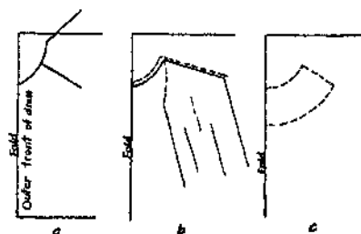
Figure 11.—Cutting a fitted facing: a and b, dress placed on material, b, cutting the neck and shoulder seam line; c, the facing pattern.
