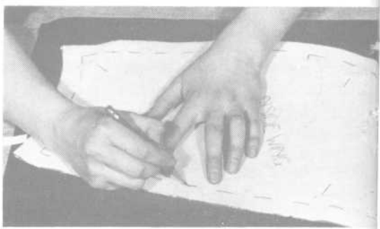
3. Marking seam lines.
