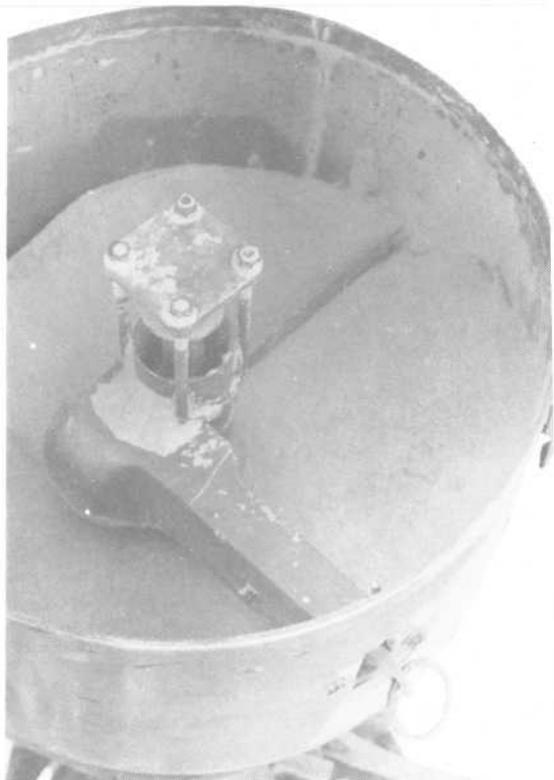
This dust feed mechanism developed by USDA researcher, Frank Irons, improves the uniformity of dust distribution.
