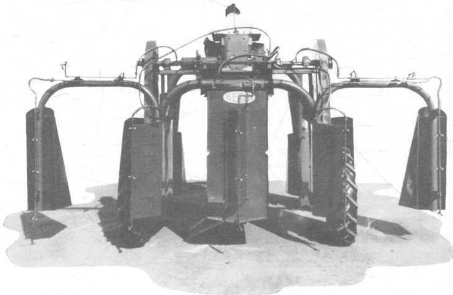
**This high-clearance spray rig is a type used in bottom defoliation. (Rear view shows shields for wheels and spray nozzles.)**
