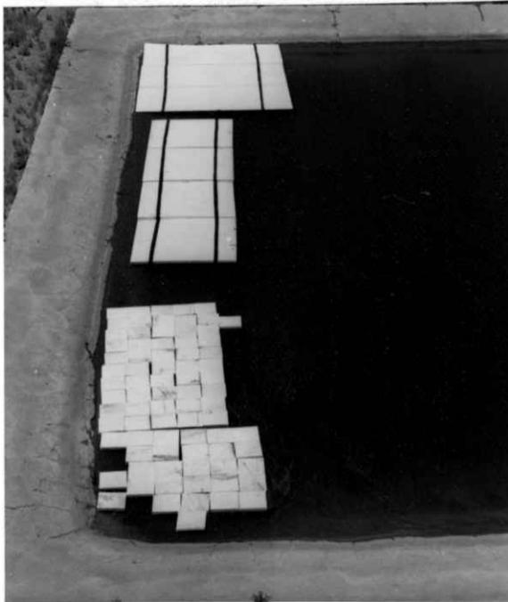
FIGURE 10. WAX IMPREGNATED EXPANDED POLYSTYRENE FLOATING COVER. (Hypalon Squares in Foreground. Rubber Banded Sheets in Background. Tested at Water Resources Research Center Field Laboratory, University of Arizona.)
