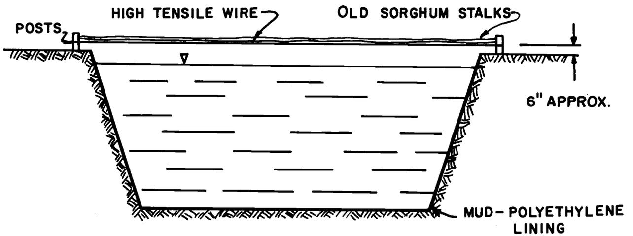
Figure 11. Mud-Polyethylene Tank Covered with Native Materials for Evaporation Control.
