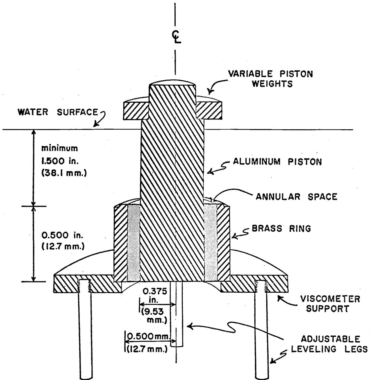
FIGURE 3. FALLING COAXIAL VISCOMETER
