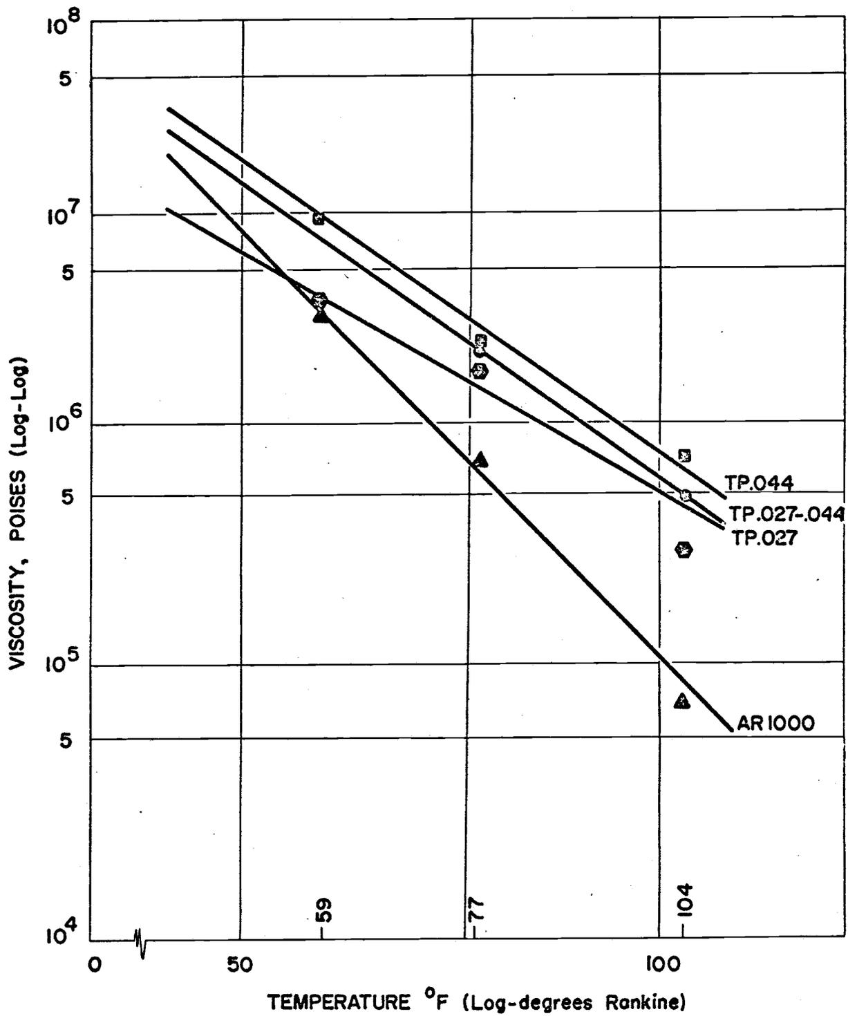
FIGURE 9. VISCOSITY - TEMPERATURE RELATIONSHIP FOR ASPHALT AND ASPHALT-RUBBER MIXTURES
