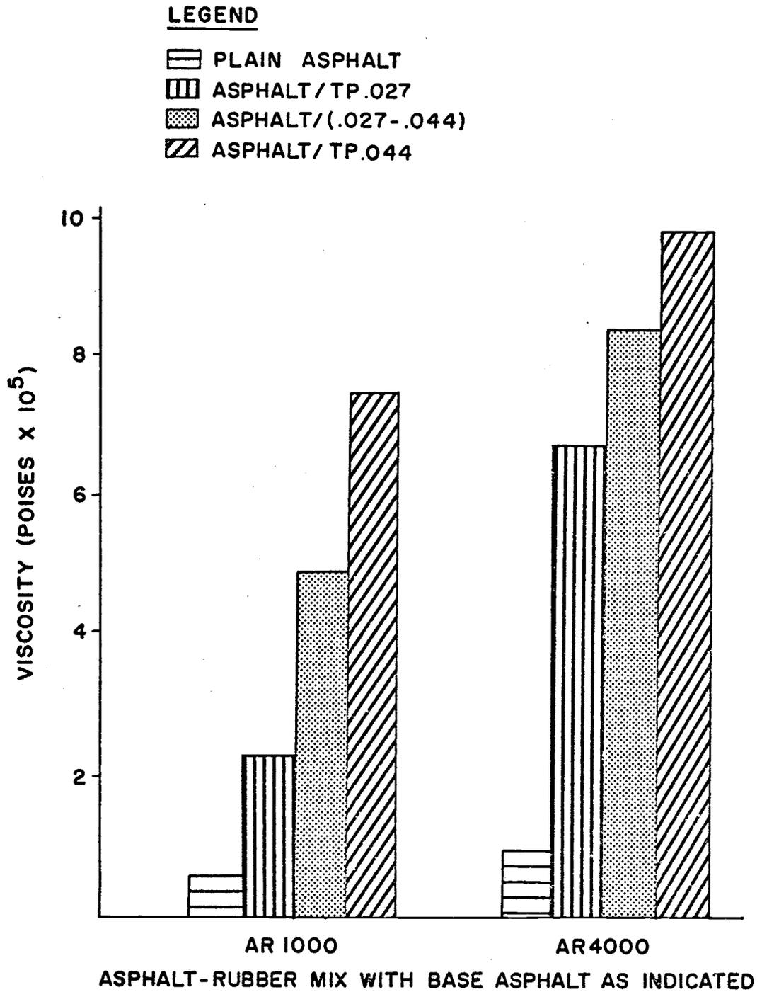
FIGURE 8. VISCOSITY OF ASPHALT AND ASPHALT-RUBBER MIXTURES TESTED AT 104°F (60°C).
