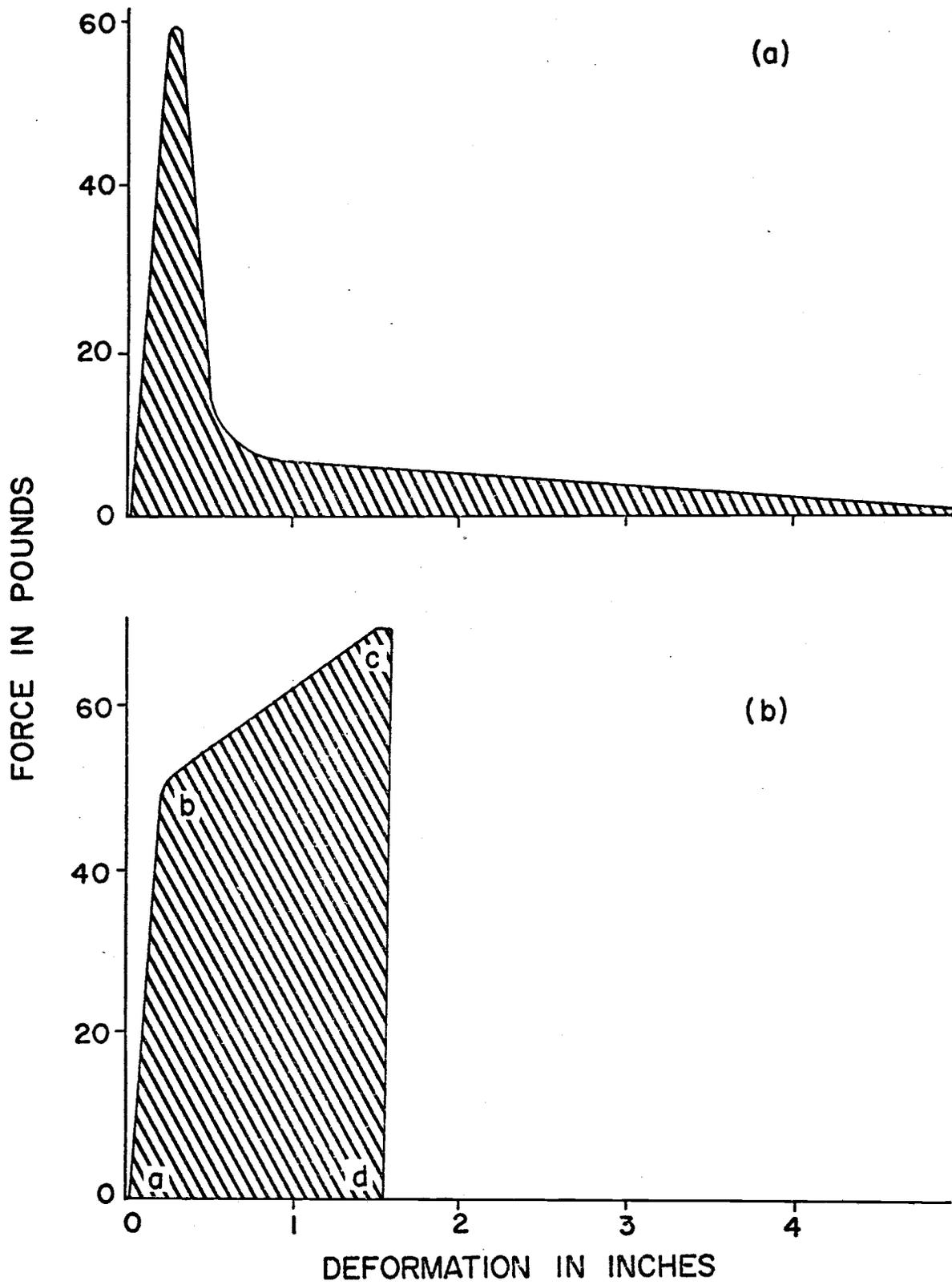
FIGURE 13. TYPICAL FORCE - DEFORMATION CURVES FOR (a) ASPHALT CEMENT AND (b) ASPHALT-RUBBER
