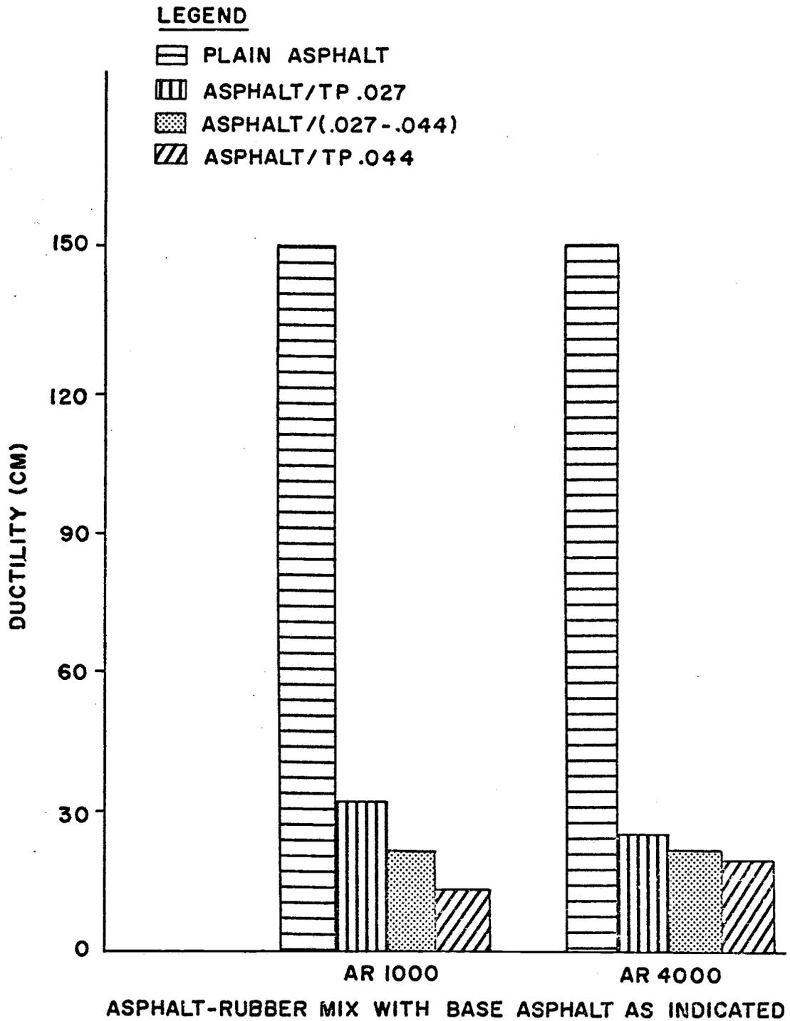
FIGURE 10. DUCTILITY VALUES FOR ASPHALT AND ASPHALT-RUBBER MIXTURES TESTED AT 77°F (25°C).
