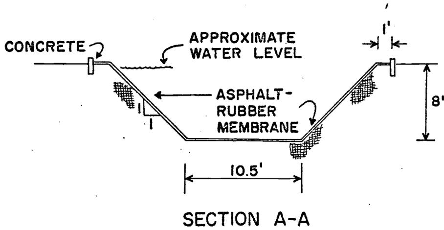
FIGURE 15. RESERVOIR USED FOR ASPHALT-RUBBER LINING INSTALLATION
