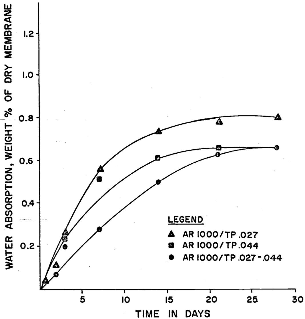
FIGURE 12. WATER ABSORPTION OF THE ASPHALT-RUBBER MEMBRANE WITH TIME
