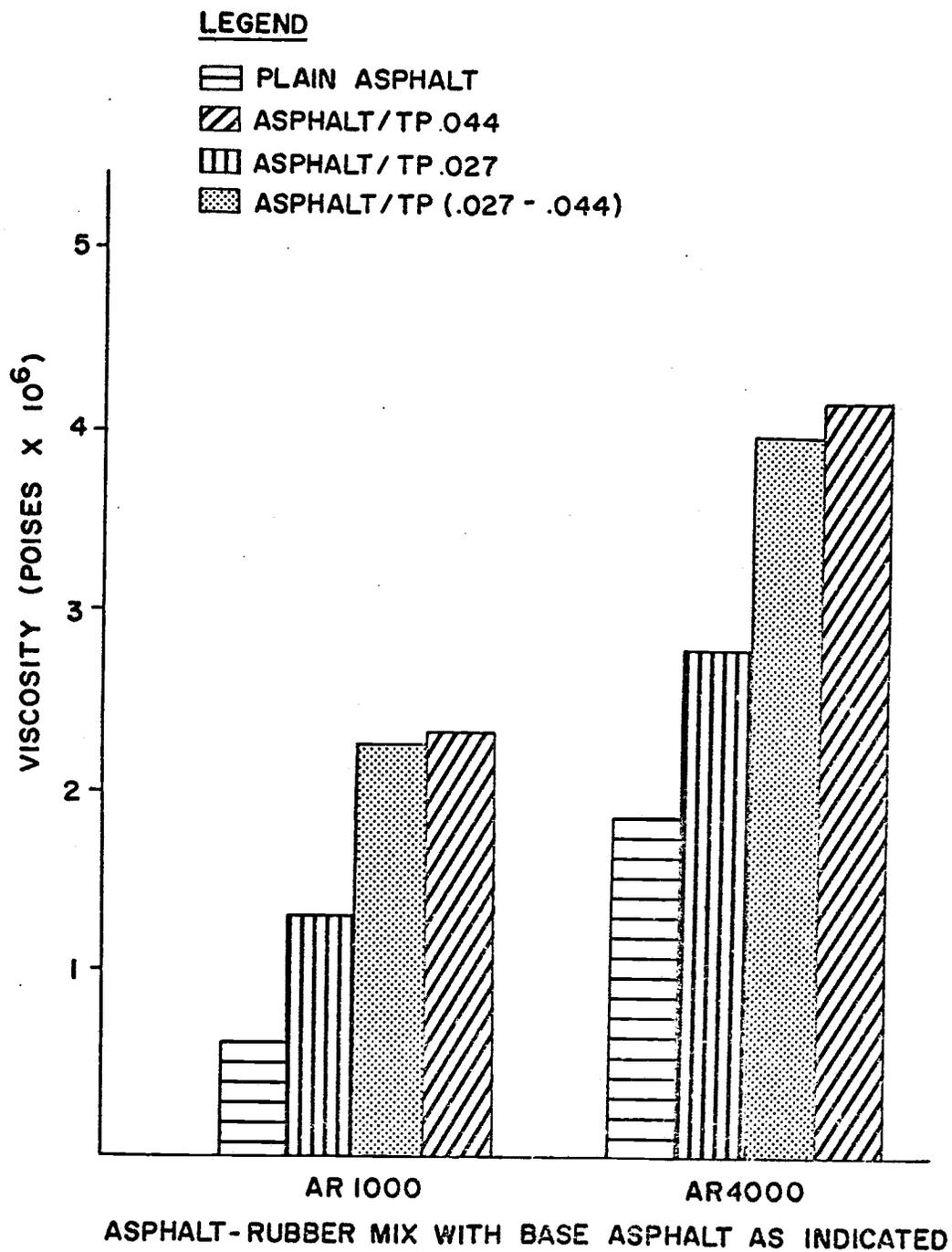
FIGURE 7. VISCOSITY OF ASPHALT AND ASPHALT-RUBBER MIXTURES TESTED AT 77°F (25°C).
