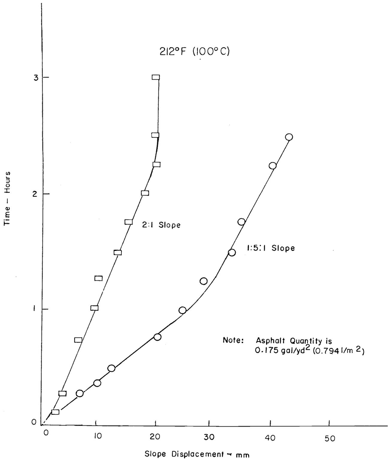
Figure 12. Effect of Temperature and Slope on the Displacement of a 3/8" Cover Aggregate Tested at 212°F (100°C) - Polypropylene Base
