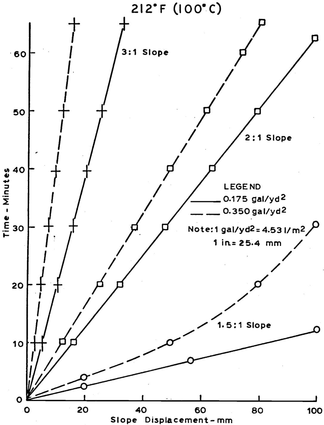
Fig. 10. Effect of Temperature and Slope on the Displacement of a 3/8 in. Cover Aggregate Tested at 212°F (100°C) - Polyethylene Base
