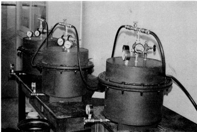
FIGURE 2. SERIES HOOK-UP OF HYDROSTATIC TEST VESSELS
