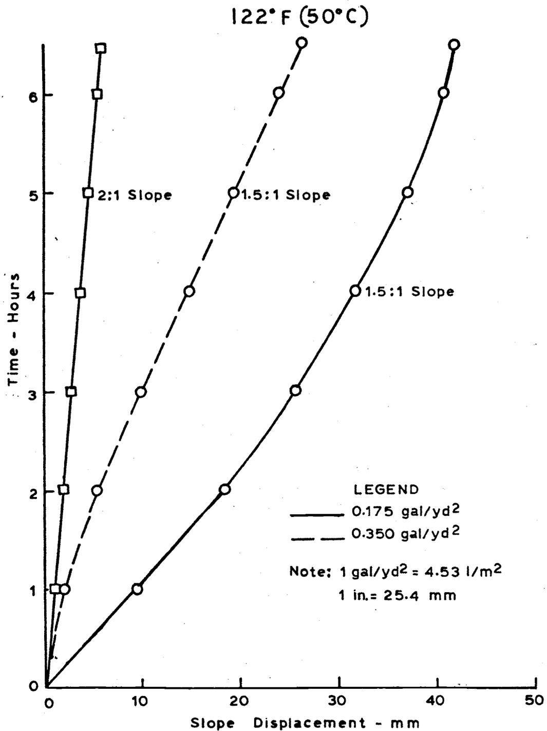
Fig. 8. Effect of Temperature and Slope on the Displacement of a 3/8 in. Cover Aggregate Tested at 122°F (50°C) - Polyethylene Base
