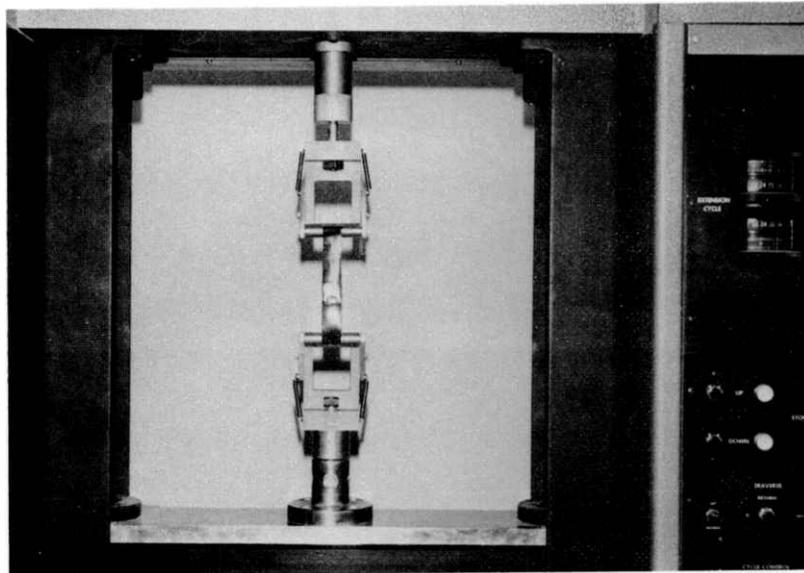
FIGURE 4. TENSILE TESTING GRIPS POSITIONED FOR TESTING OF OVERLAP SPECIMEN
