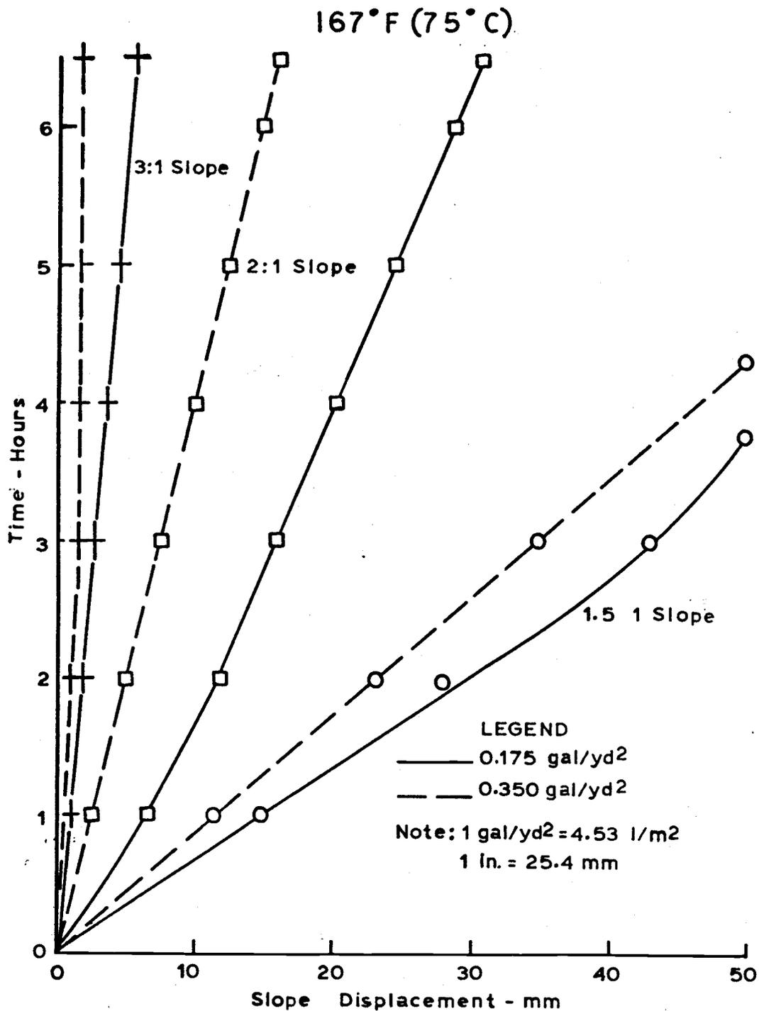
Fig. 9. Effect of Temperature and Slope on the Displacement of a 3/8 in. Cover Aggregate Tested at 167°F (75°C) - Polyethylene Base
