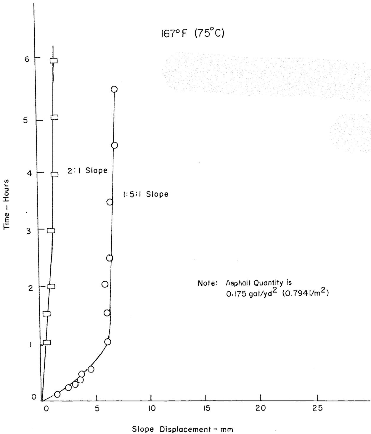
Figure 11. Effect of Temperature and Slope on the Displacement of a 3/8" Cover Aggregate Tested at 167°F (75°C) - Polypropylene Base
