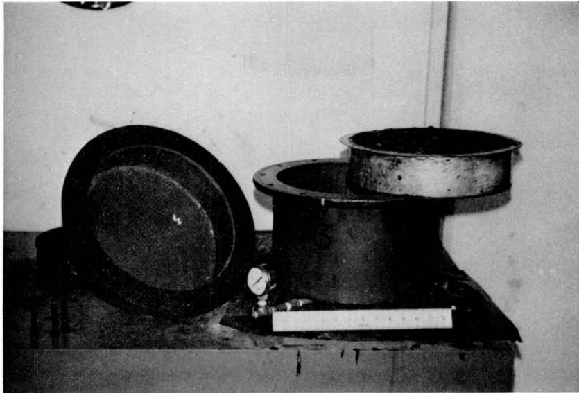
FIGURE 1. HYDROSTATIC TEST VESSEL - UNASSEMBLED
