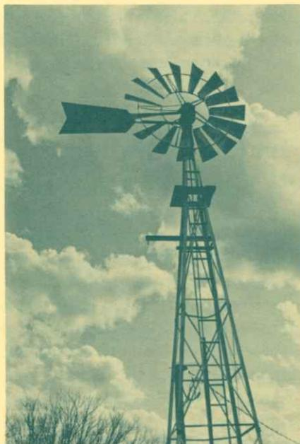
Symbol of the West, the windmill pumps groundwater to the surface.
