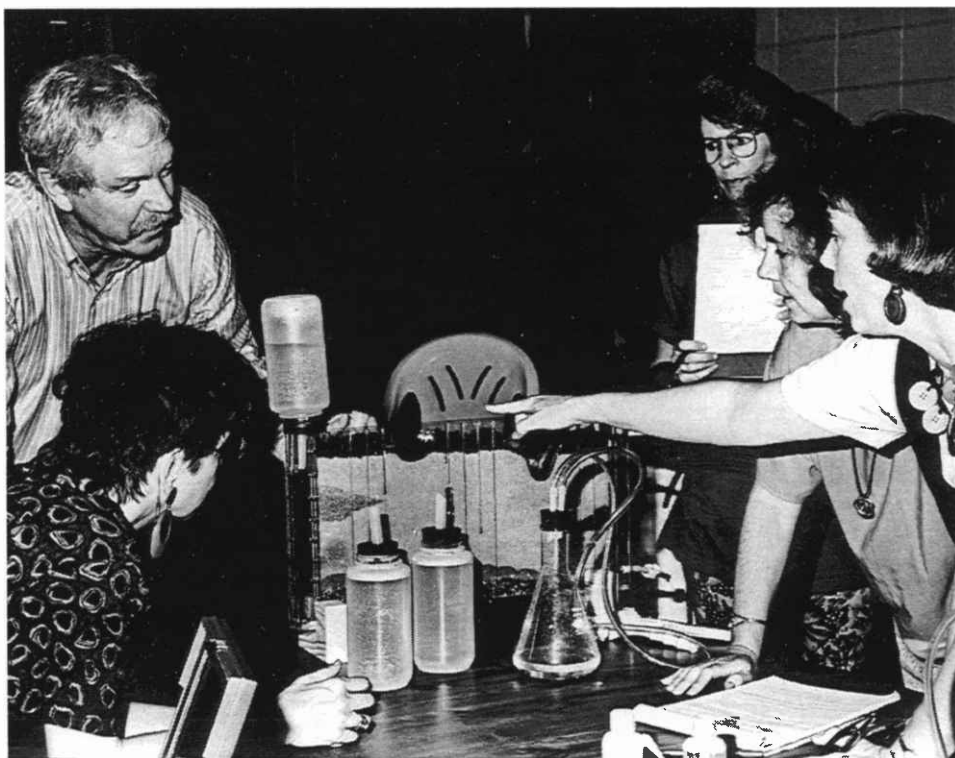
Lawrence Sullivan, Project WET (Water Education for Teachers) director, demonstrates a groundwater flow model to Tucson teachers. The three-dimensional sand tank models represent a vertical cross section of an aquifer. When charged with water, they become mini-aquifers complete with wells that pump water, a lake, a leaky lagoon and an artesian well. Project WET is part of the Water Resources Research Center's outreach program. (Photo: B. Tellman)
