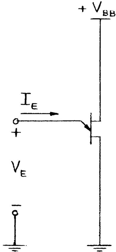
Fig. 1.3 Unijunction Transistor Circuit Arrangement
