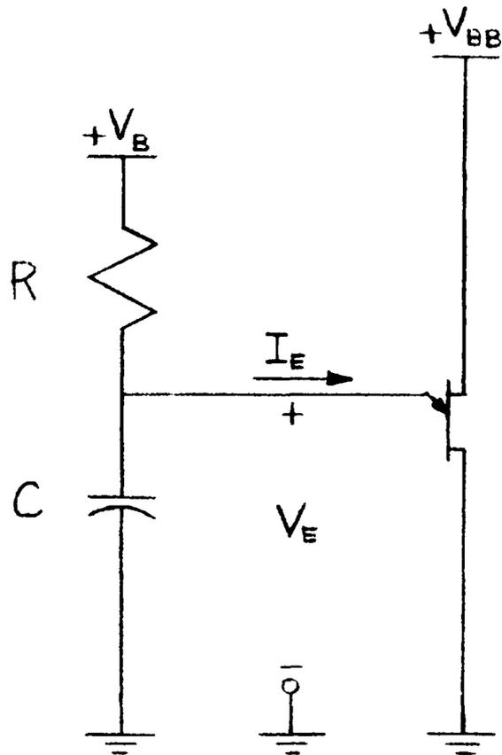
Fig. 1.5 Unijunction Transistor Monostable Oscillator Circuit
