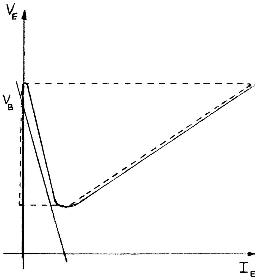
Fig. 1.6 Unijunction Transistor Monostable Oscillator Characteristic Including Load Line and Operating Path
