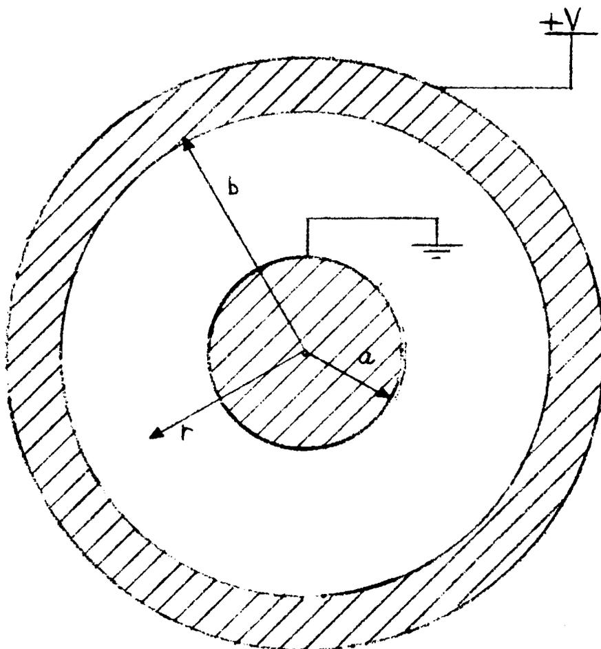
Fig. 2.2 Test Geometry for Resistance Paper
