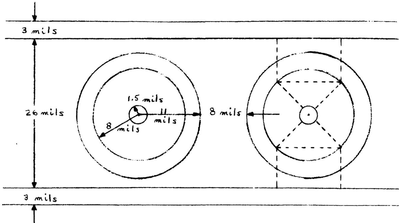
Fig. 3.2 Neuristor Geometry No. 1
