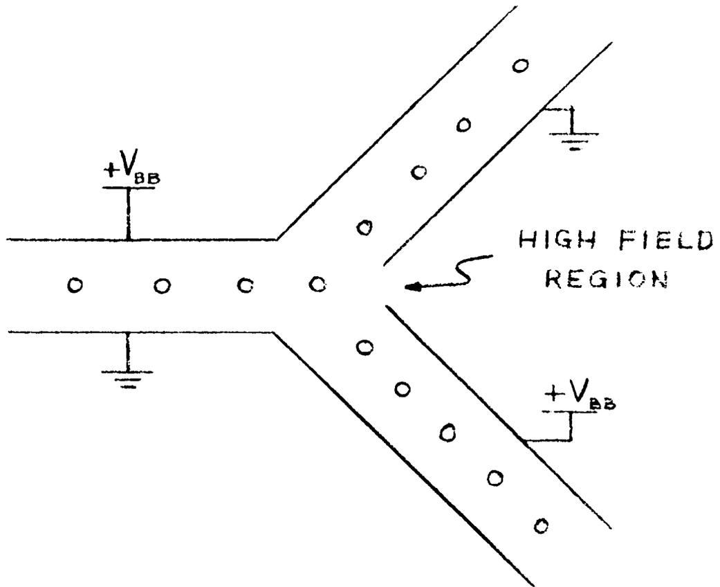
Fig. 1.9 Problem of High Field Region at T Junction in Adaptation of Bar Geometry
