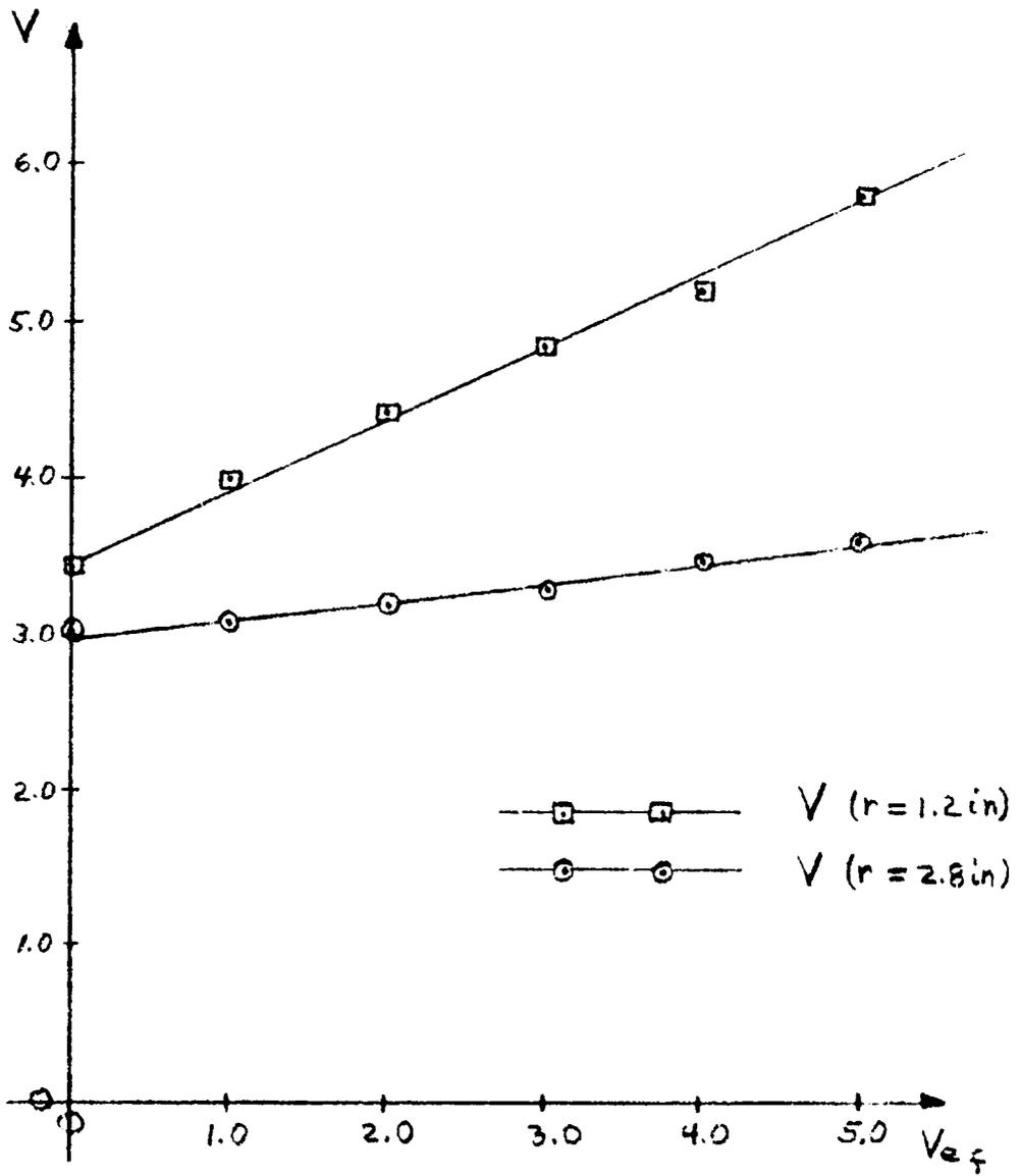
Fig. 2.7 Potential at Two Radii vs. Fired Emitter Potential for Open Channel Geometry
