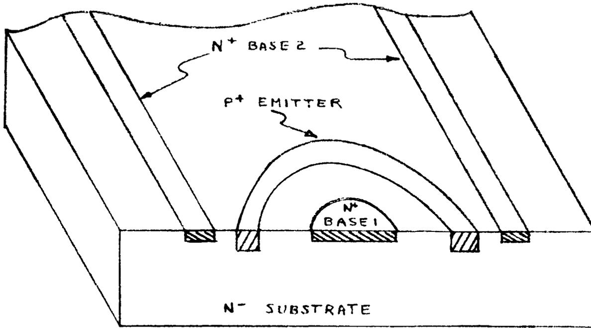
Fig. 3.1 Adapted Cylindrical Unijunction Transistor Geometry
