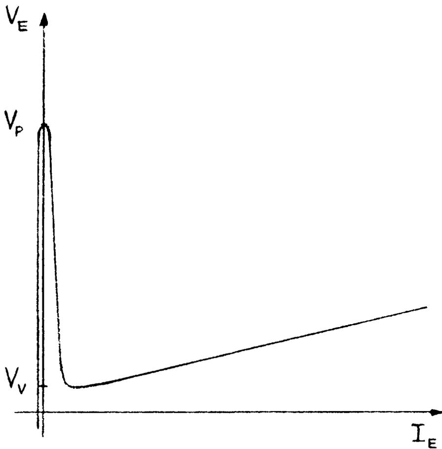
Fig. 1.4 Unijunction Transistor Emitter Characteristics
