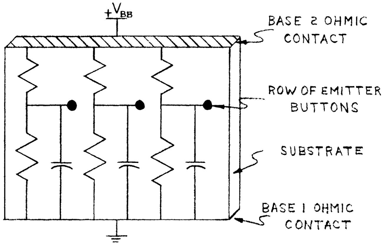
Fig. 1.7 Complete Neuristor Line Including External Lumped Circuitry
