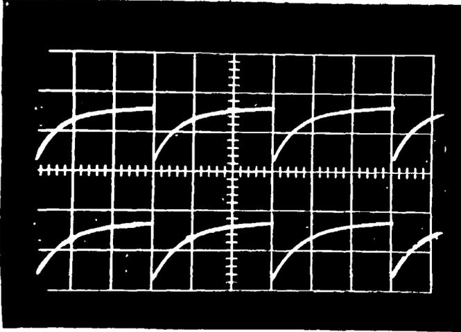
Fig. 4.2 Pulse Propagation on Neuristor Line
