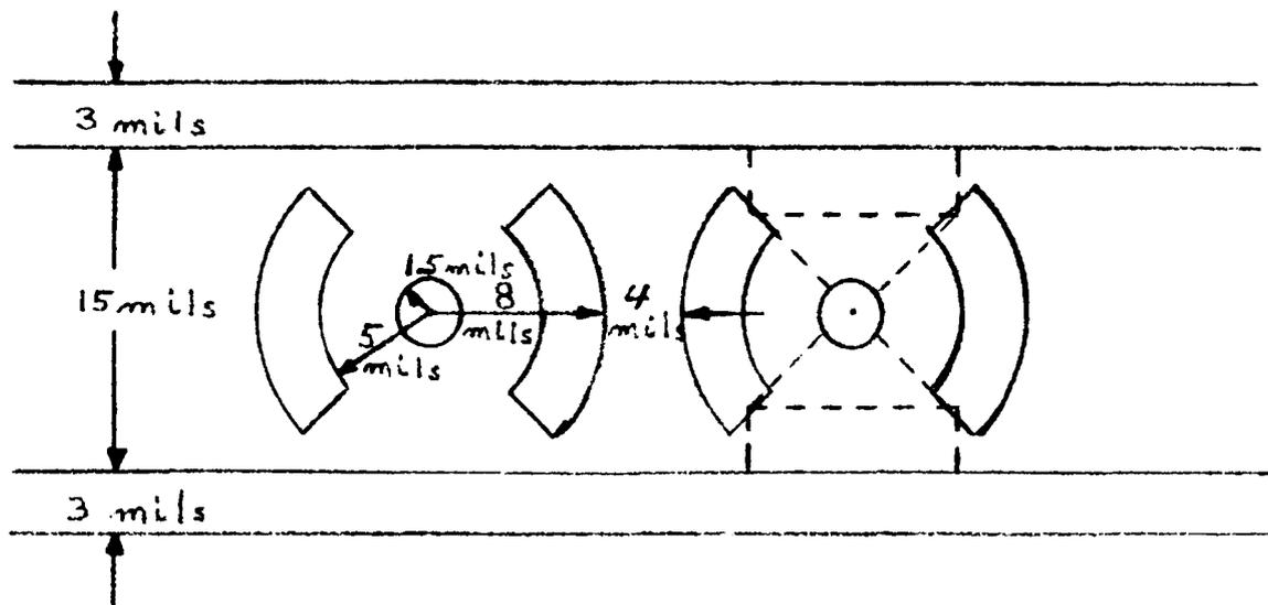
Fig. 3.5 Neuristor Geometry No. 4
