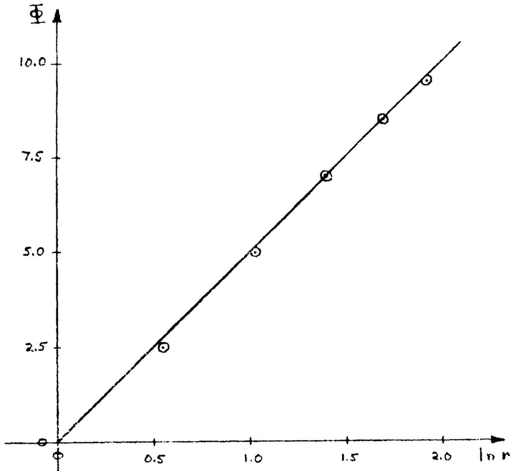
Fig. 2.3 Potential vs. Radius for Geometry of Fig. 2.2
