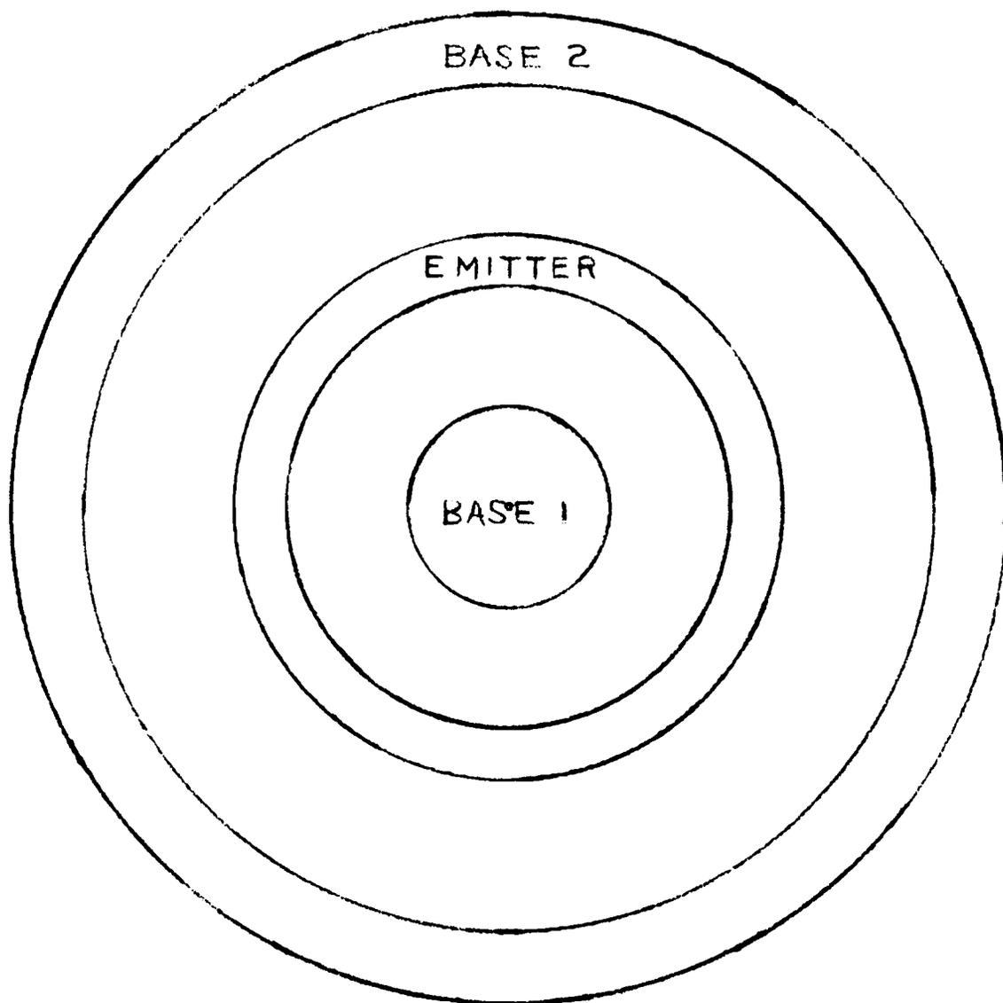
Fig. 1.10 Cylindrical Geometry Configuration of Unijunction Transistor
