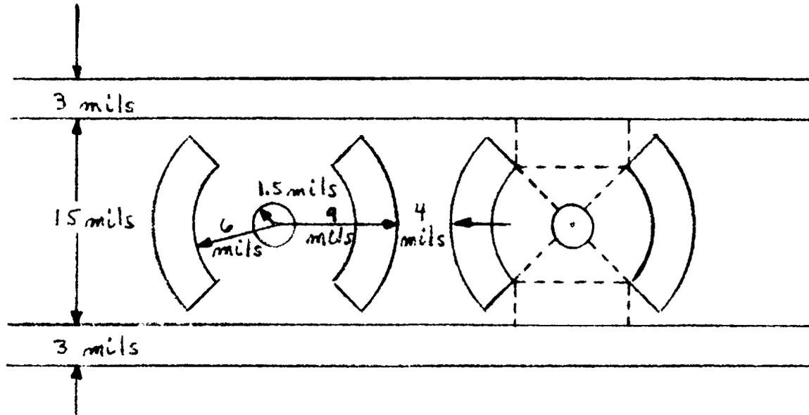
Fig. 3.6 Neuristor Geometry No. 5
