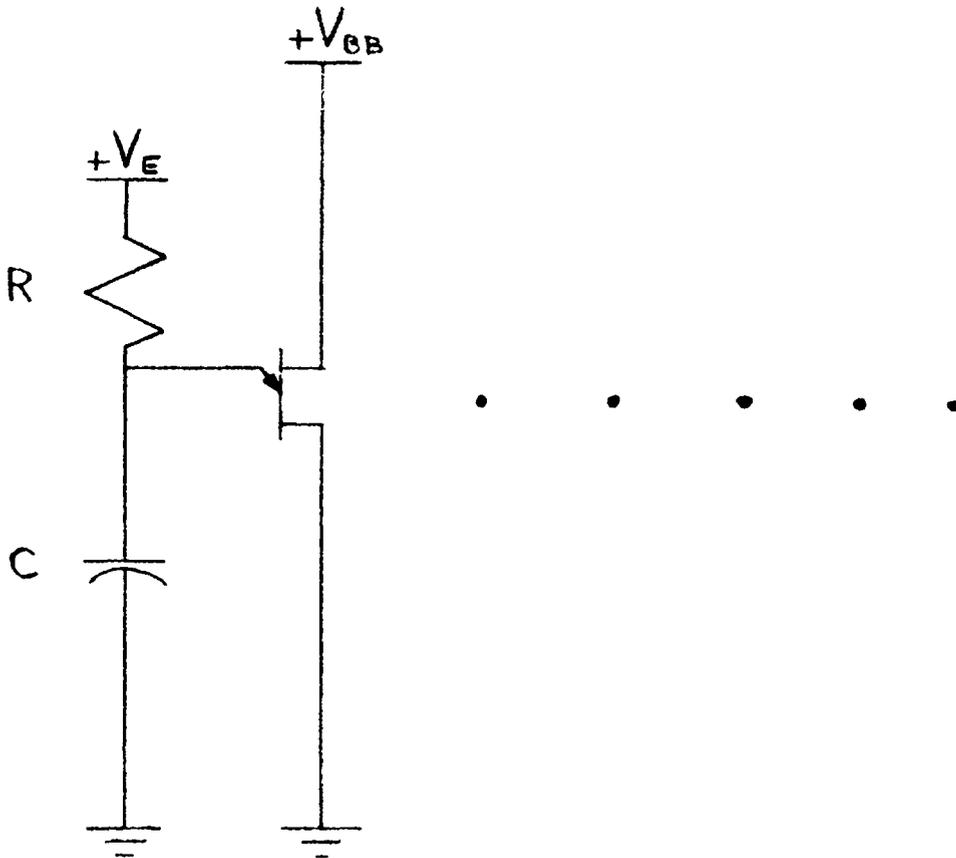
Fig. 4.1 Neuristor Line Circuit Connections
