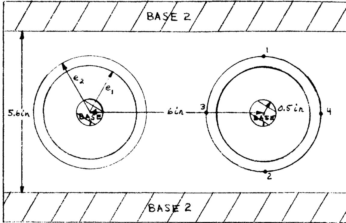
Fig. 2.5 Open Channel Neuristor Geometry
