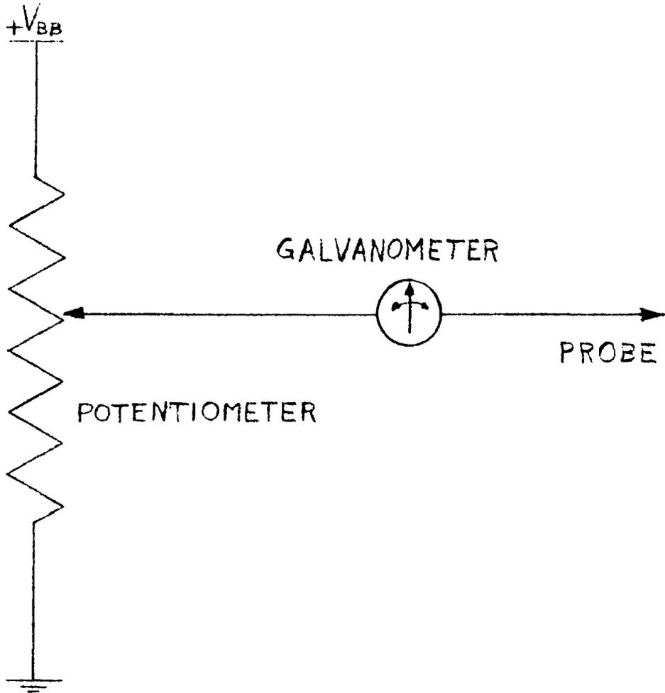
Fig. 2.1 Potential Measuring Equipment
