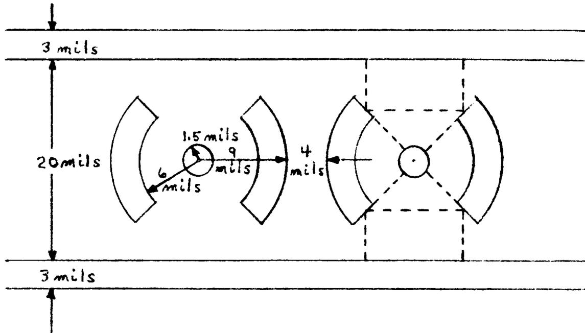
Fig. 3.4 Neuristor Geometry No. 3
