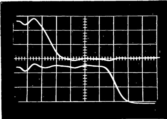
Fig. 4.3 Pulse Fall Time on Neuristor Line
