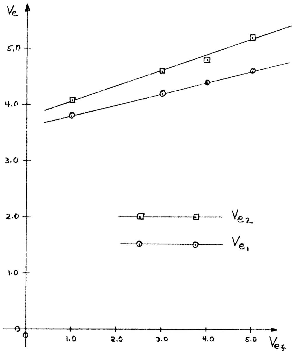
Fig. 2.6 Nearest Neighbor Emitter Potential vs. Fired Emitter Potential for Open Channel Geometry
