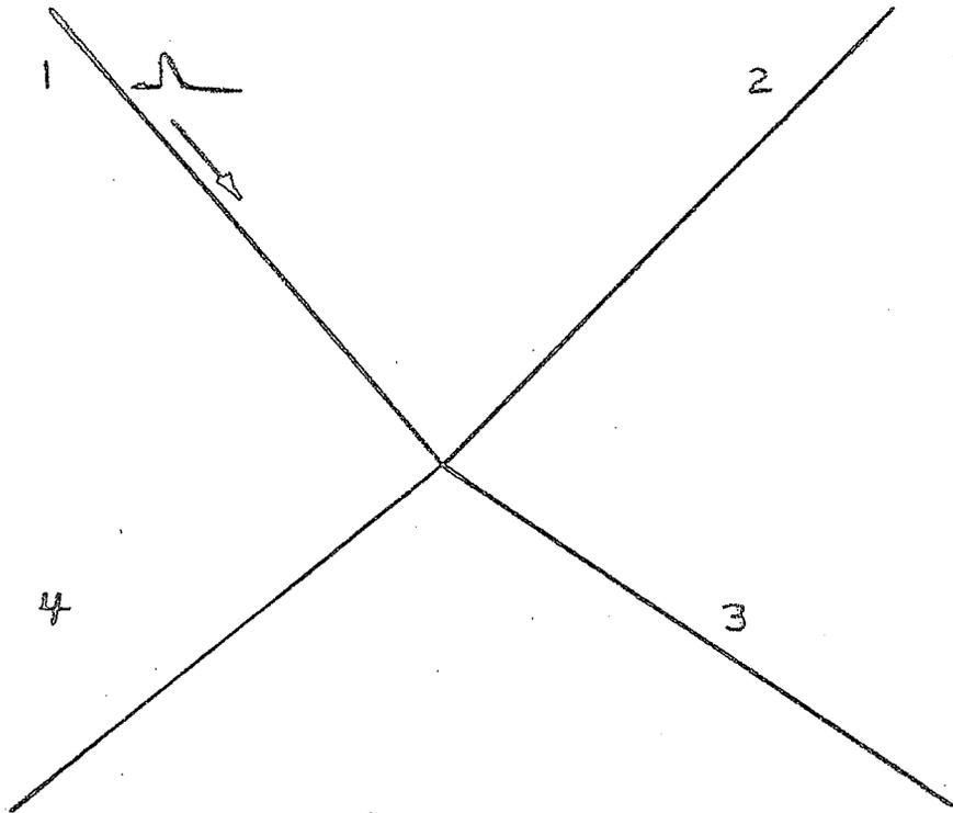
Fig. 1.1 Four Branch Neuristor T Junction
