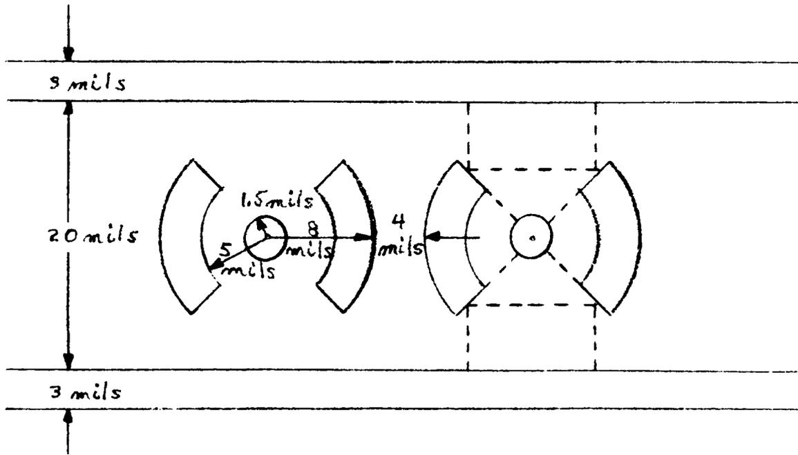
Fig. 3.3 Neuristor Geometry No. 2
