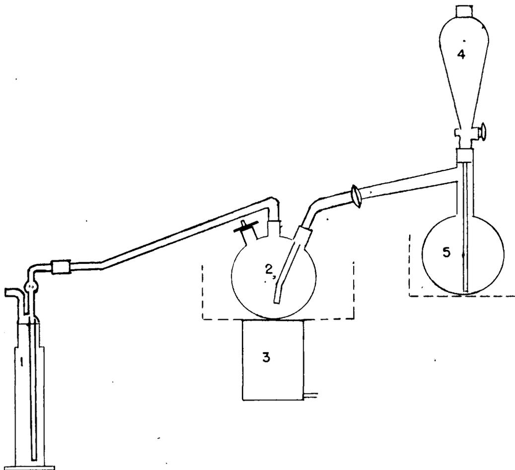
Fig. 1 Diazomethane Esterification Apparatus
