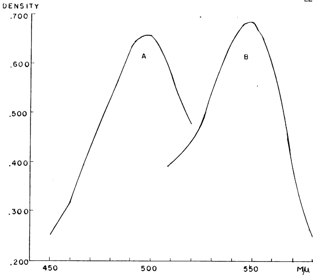
Fig. 6 Comparison of Halphen Reaction Color Products of Refined Cottonseed Oil with and without Sulfur
