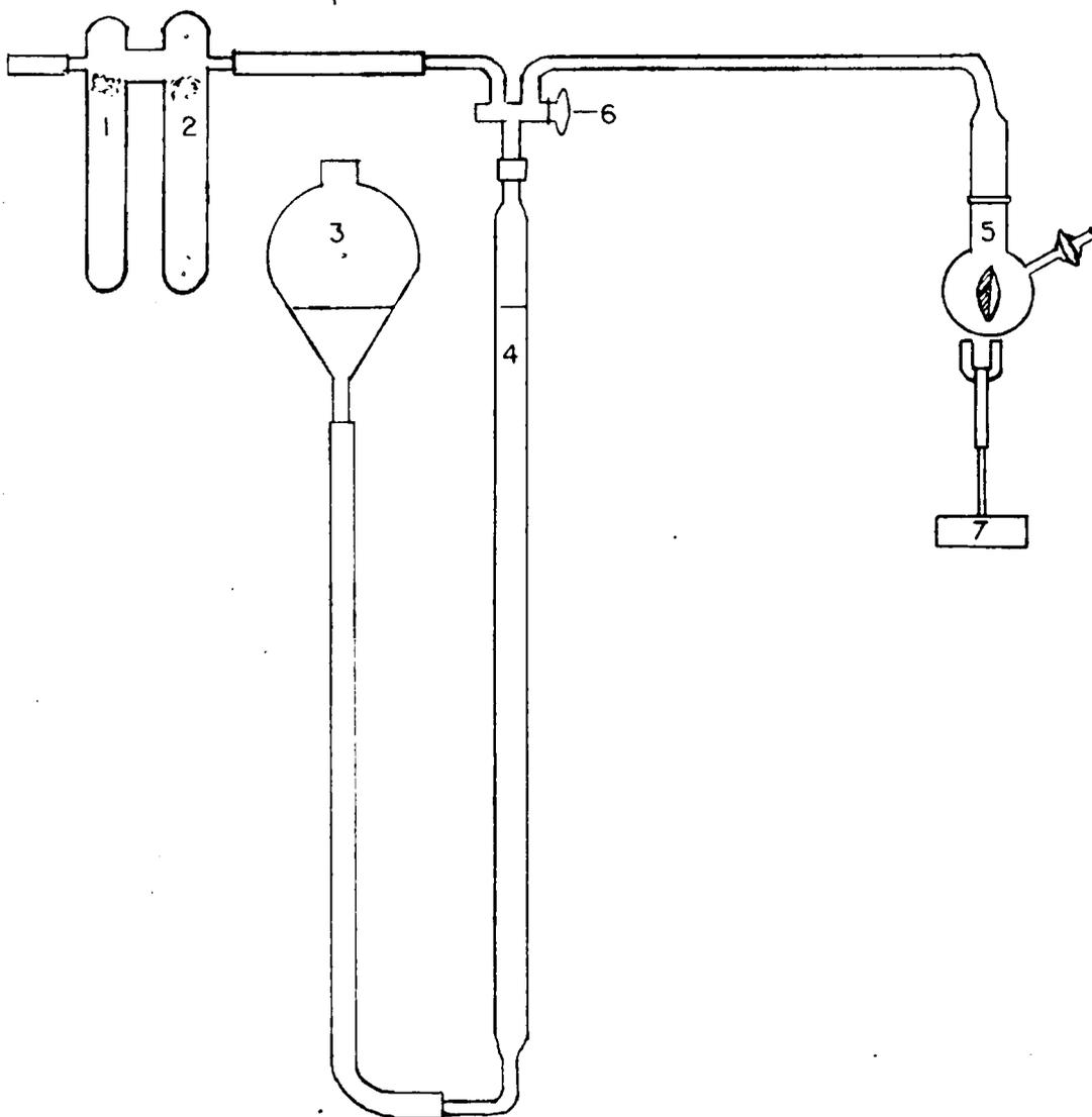
Fig. 12 Micro Hydrogenation Apparatus
