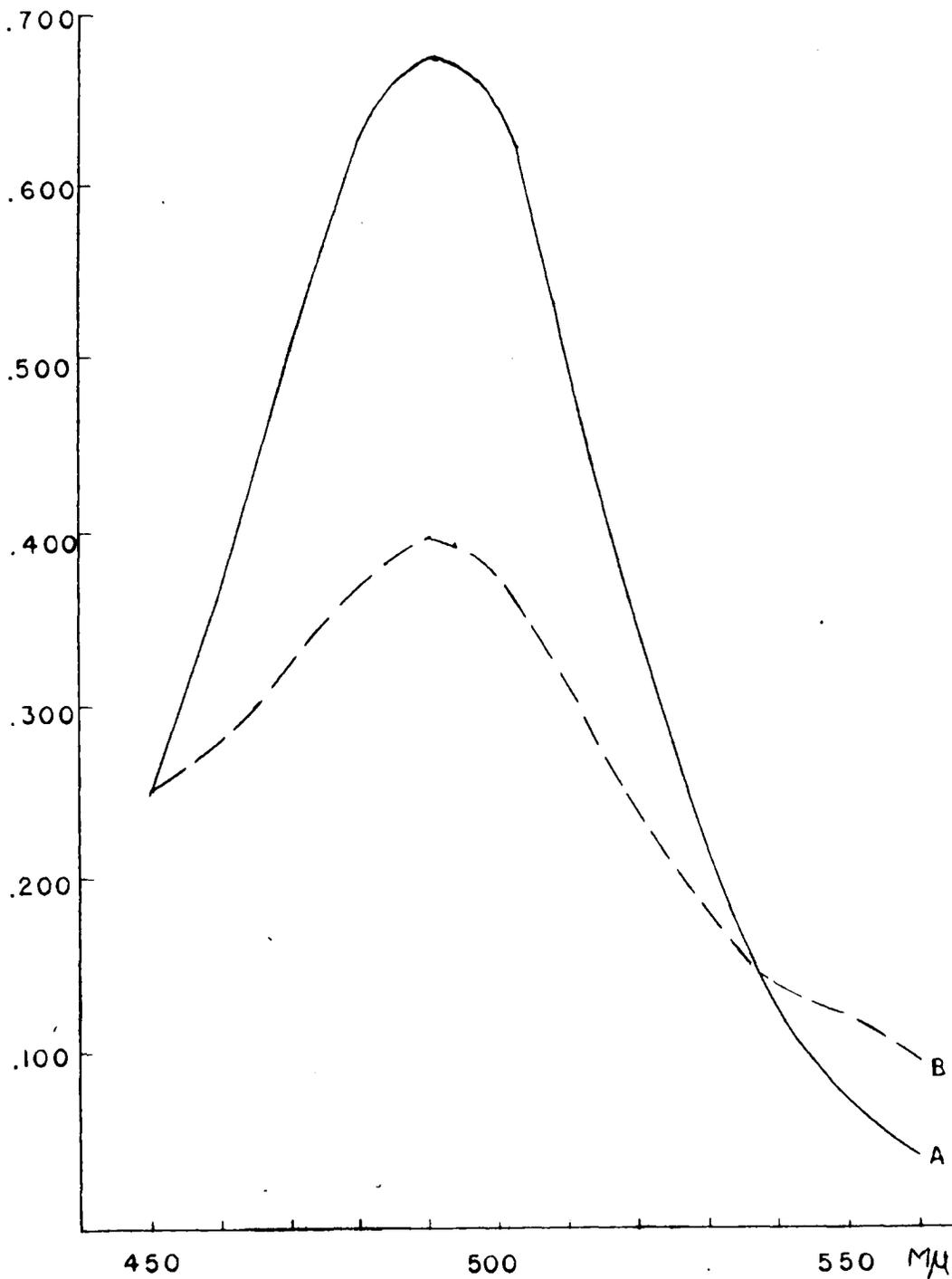
Fig. 5 Comparison of Halphen Reaction Color Products of Sterculia foetida oil in Isoamyl Alcohol
