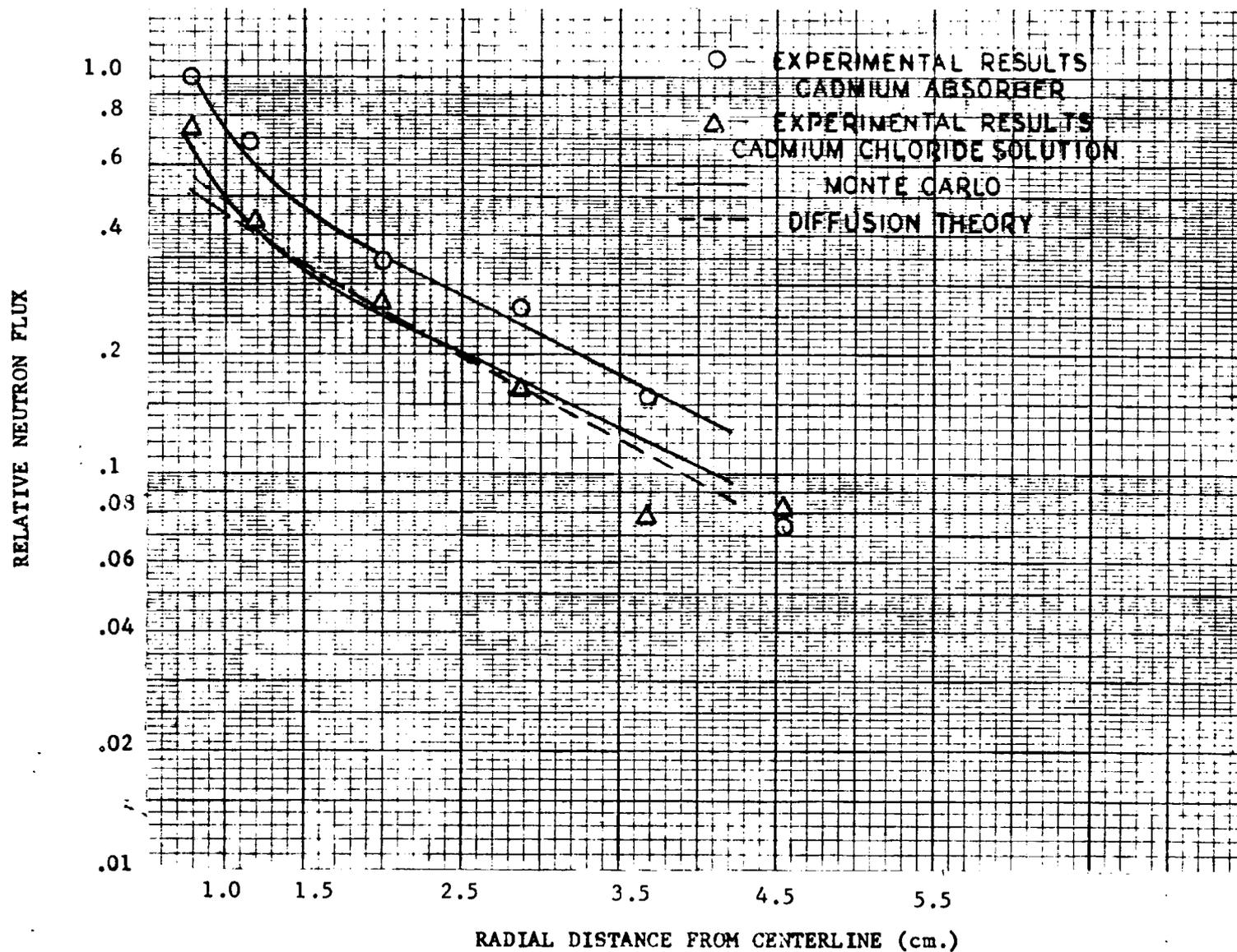
The Monte Carlo calculation predicts the variation of the flux near both absorbers since it closely matches that determined experimentally. The flux curves are normalized on the basis of the number of absorptions occurring in each of the absorbers.
