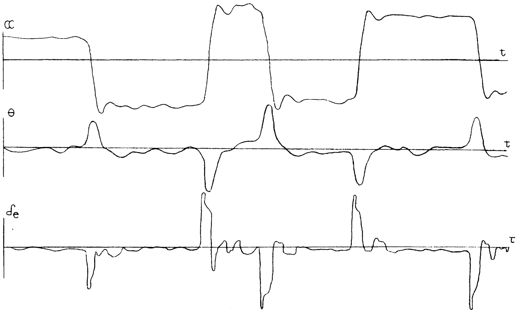
Fig. 5.1. Pilot Response Curves for Small Disturbances
