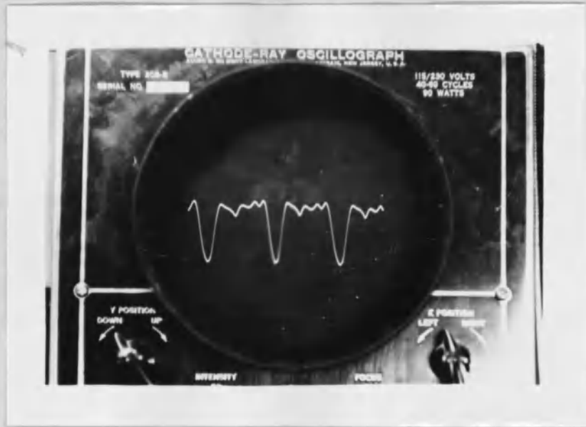
(a) Pulse wave from first three harmonics
