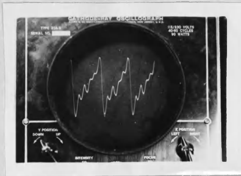
(a) Sawtooth wave from first six harmonics
