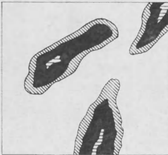
Figure 3 - Polished surfaces of residue particles leached for 30 minutes with acid and oxygen magnified at 100X.
