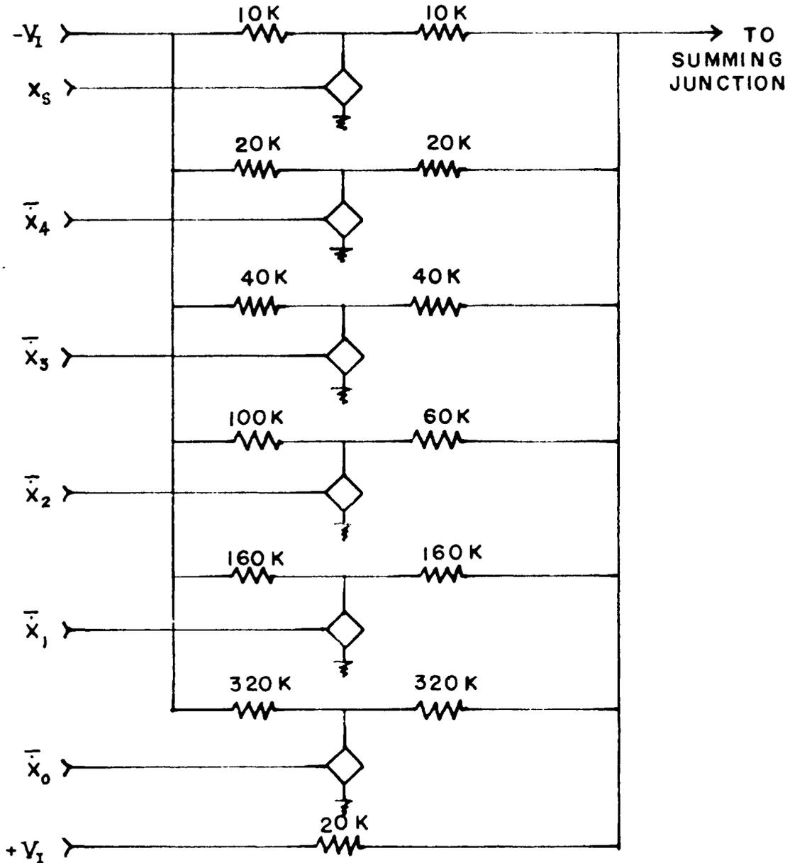
Fig. 5 6-bit D/A multiplier
