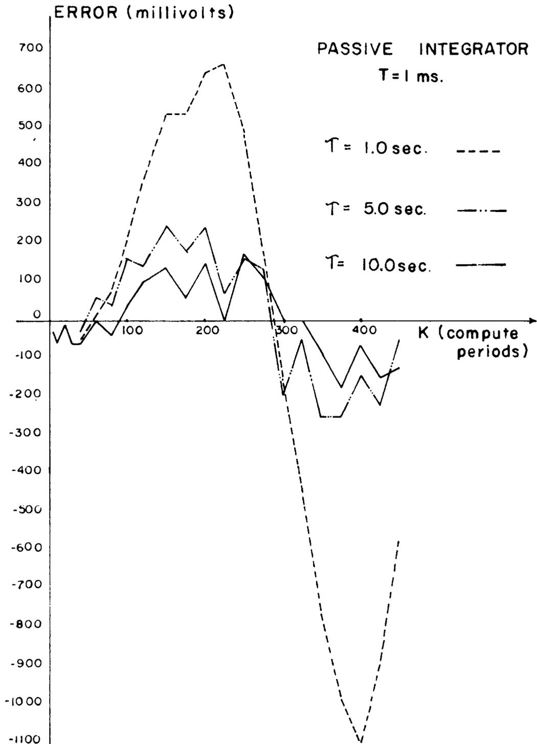
Fig. 9 Results, employing passive analog integrator
