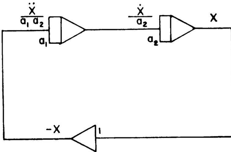
Fig. 7 Sine loop (circle) test
