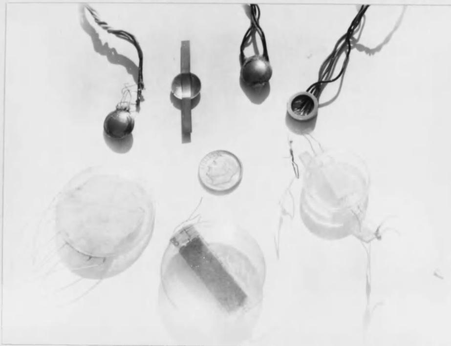
FIGURE 6. Experimental Pressure Cells. The diaphragm type cell is shown in the upper right portion of the figure. The lower cells are made from watch crystals.
