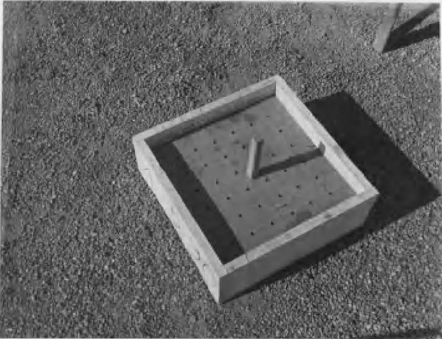
FIGURE 12. Template for Placement of Seed.
