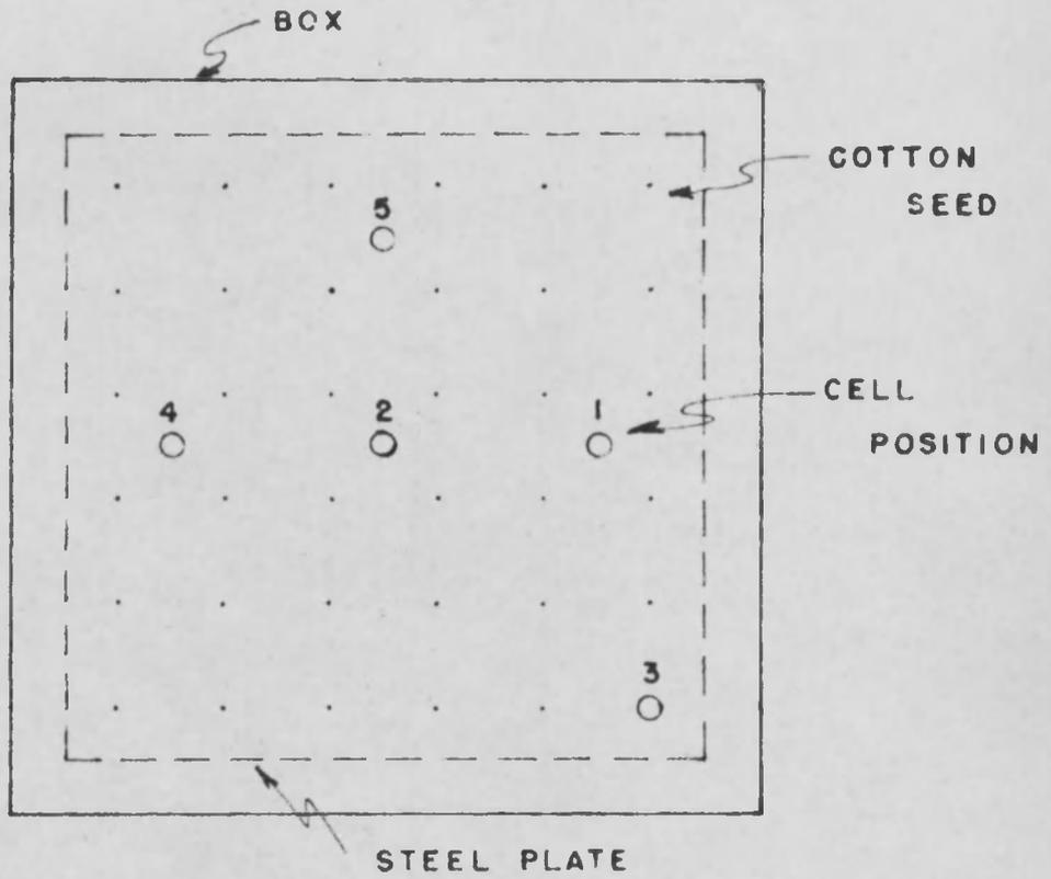
**FIGURE 13.** Pressure Cell Position and Cotton Seed Placement
