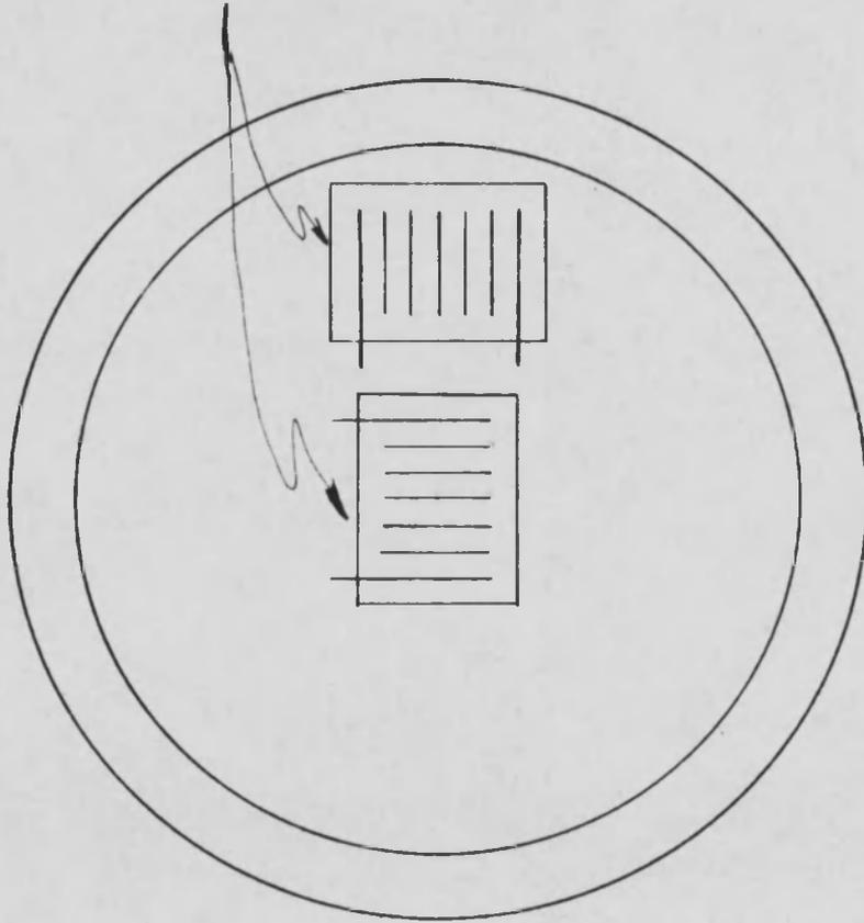
FIGURE 5. Strain Gage Placement on Diaphragm.
