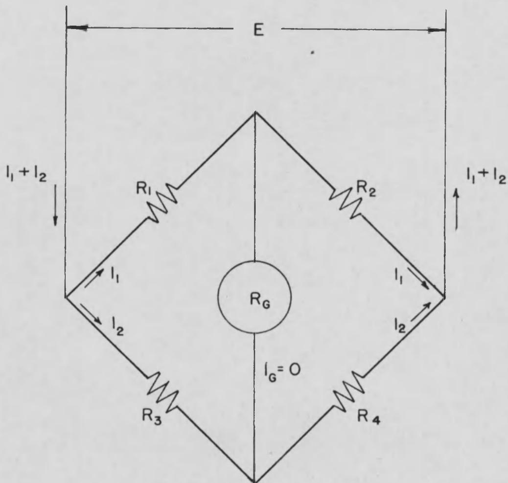
FIGURE 3. Wheatstone-Bridge Circuit
