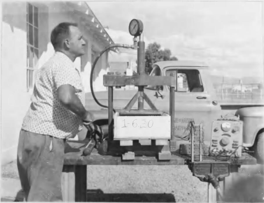
FIGURE 14. Hydraulic Press, Switching Unit, and Indicator. Pressure is being applied to the soil in the box.
