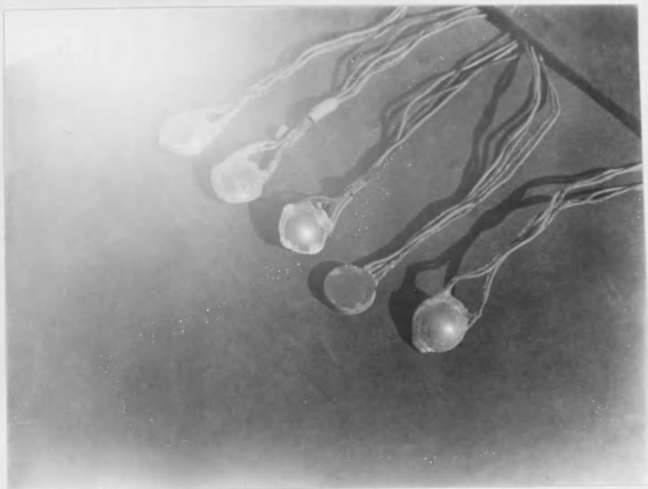
FIGURE 9. Pressure Cells Used in Emergence Study.
