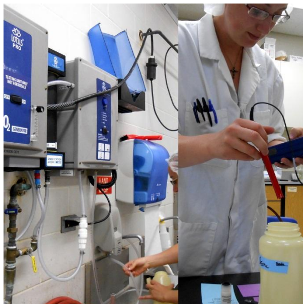
From left to right: The FPSL's ozone machine Testing using Reed's pH/ORP meter to get the mV of the ozonated water
