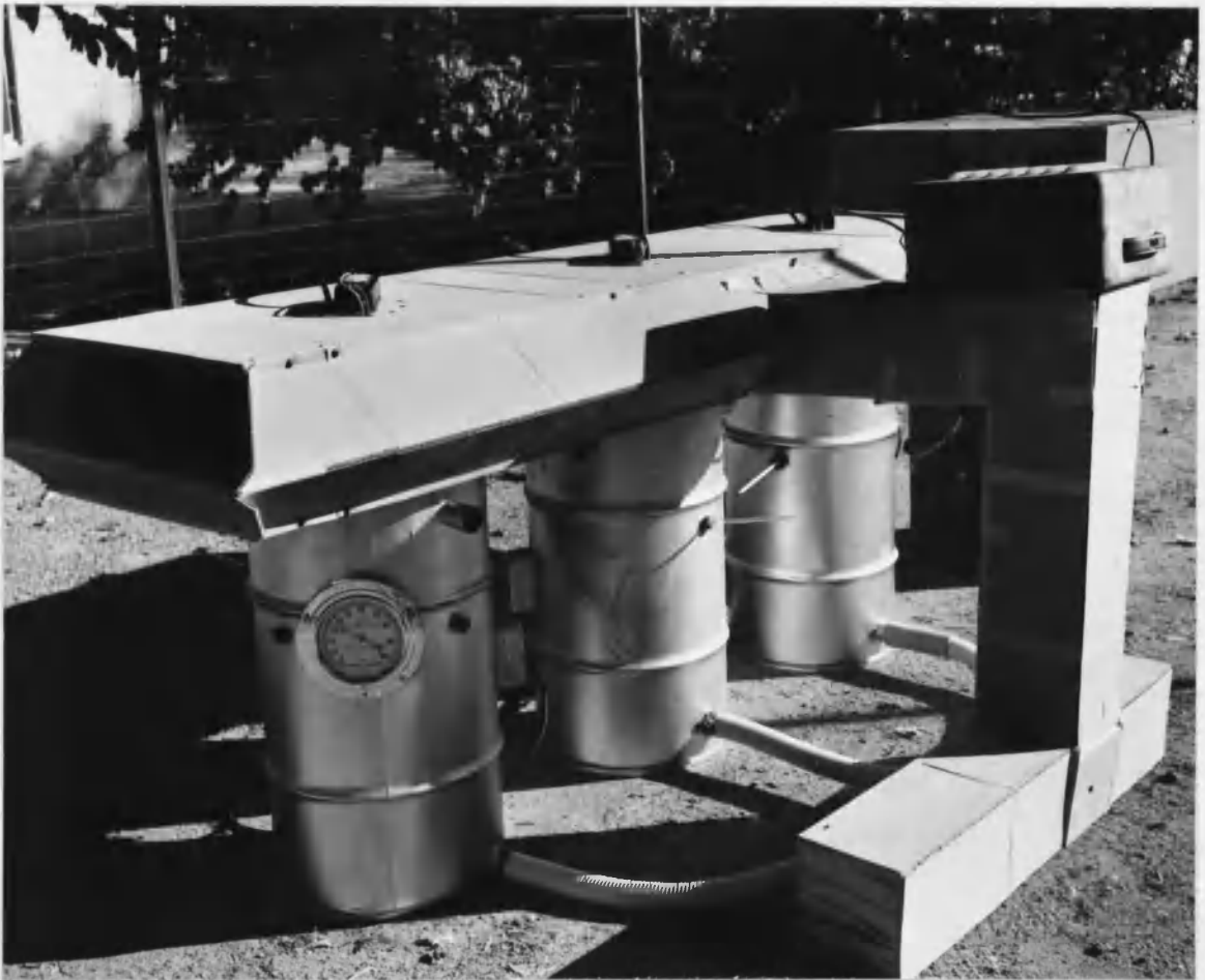
Figure 2. Growth chambers showing plant chambers (lower left) with temperature and humidity gauges, refrigeration unit (far end), light bank (top left) and auxiliary heater (top, right foreground).
