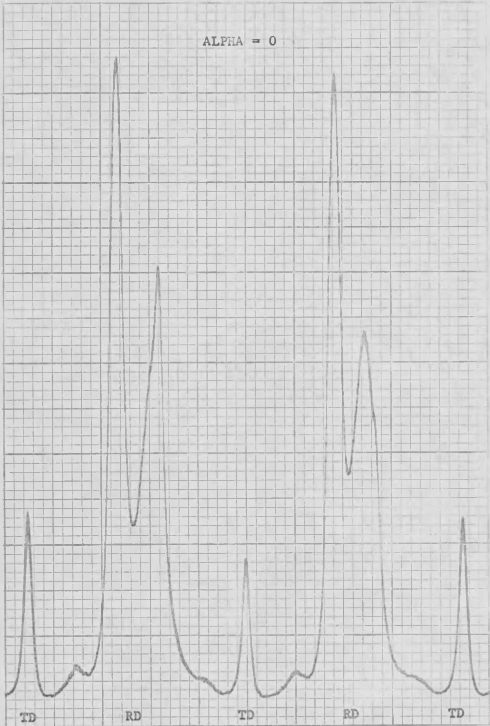
Figure 12. Partial \{111\} pole figure scan of 99.999% copper rolled 98.3%
