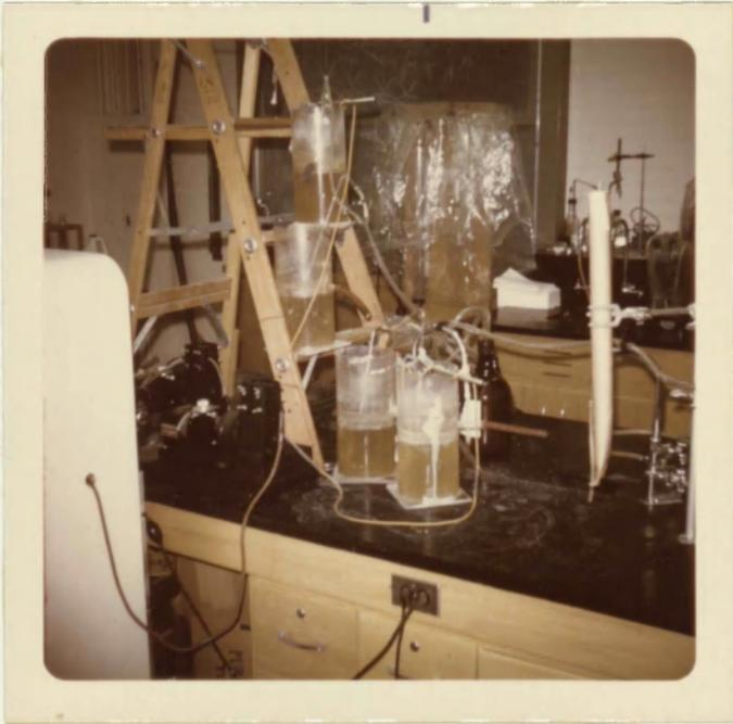
Figure 3.5 Phase two activated sludge reactors
