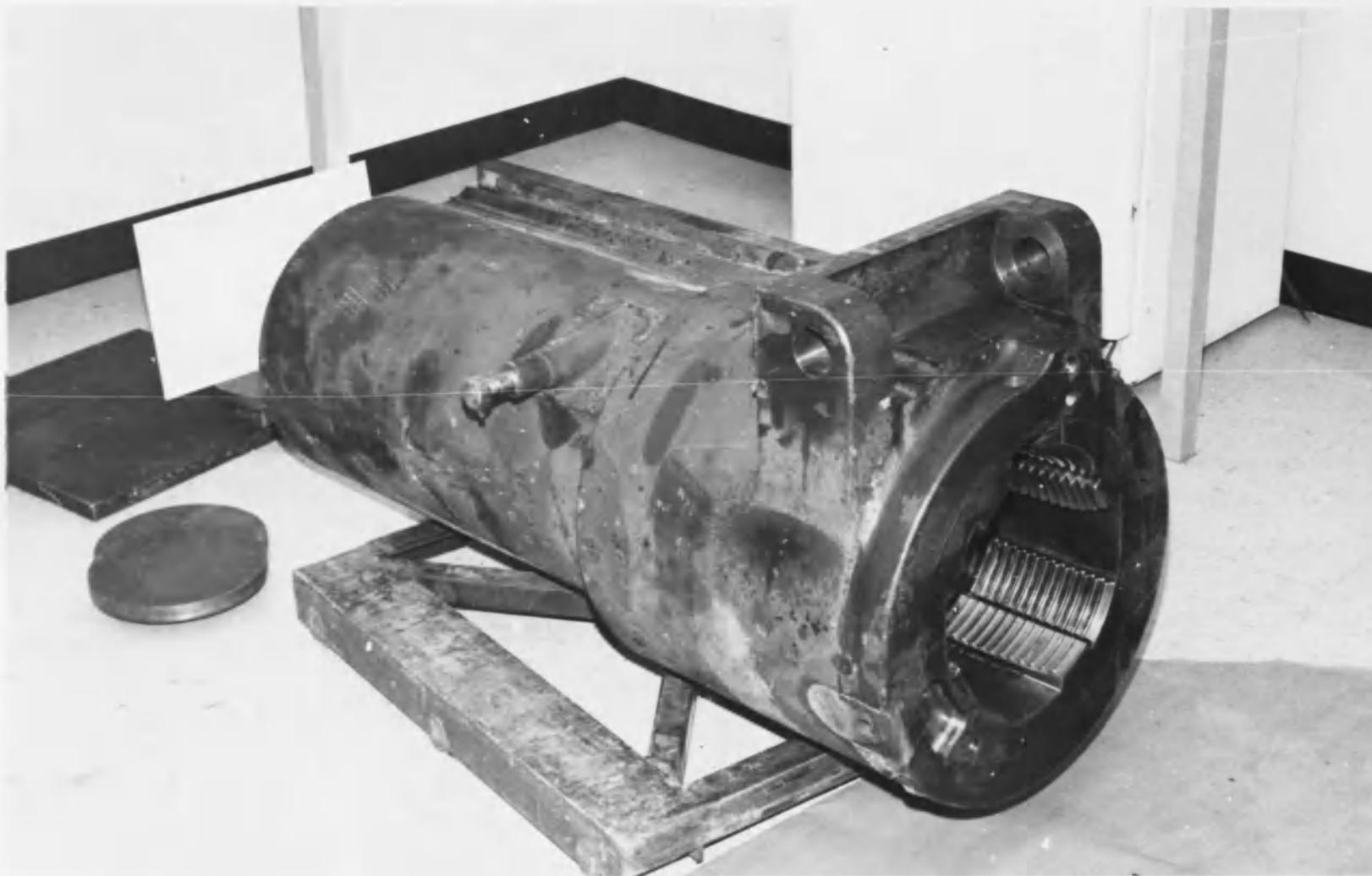
Fig. 15. Four Foot Section of 6-inch Naval Gun Barrel
