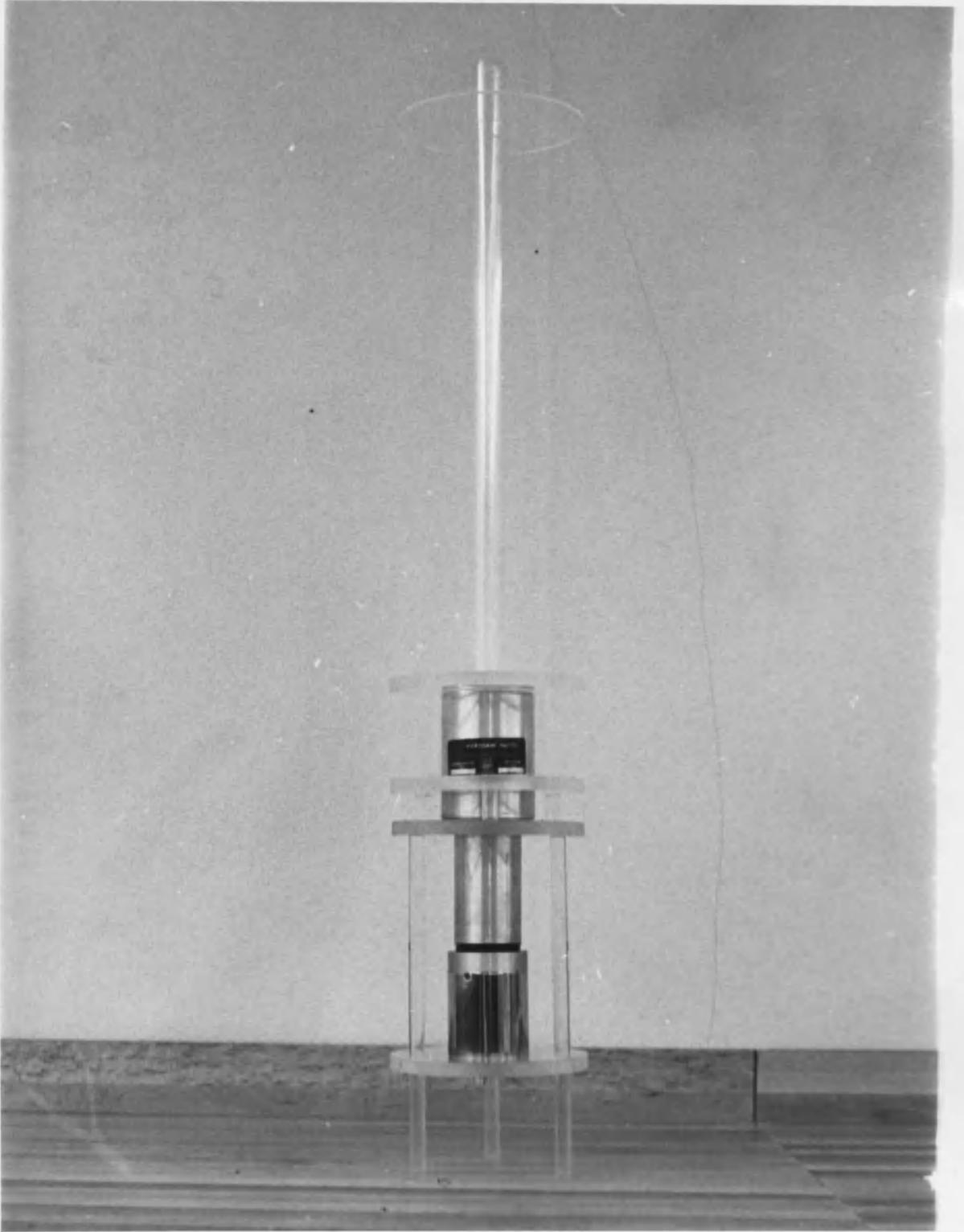
Fig. 18. Detector with Access Tube Assembly for Small Samples
