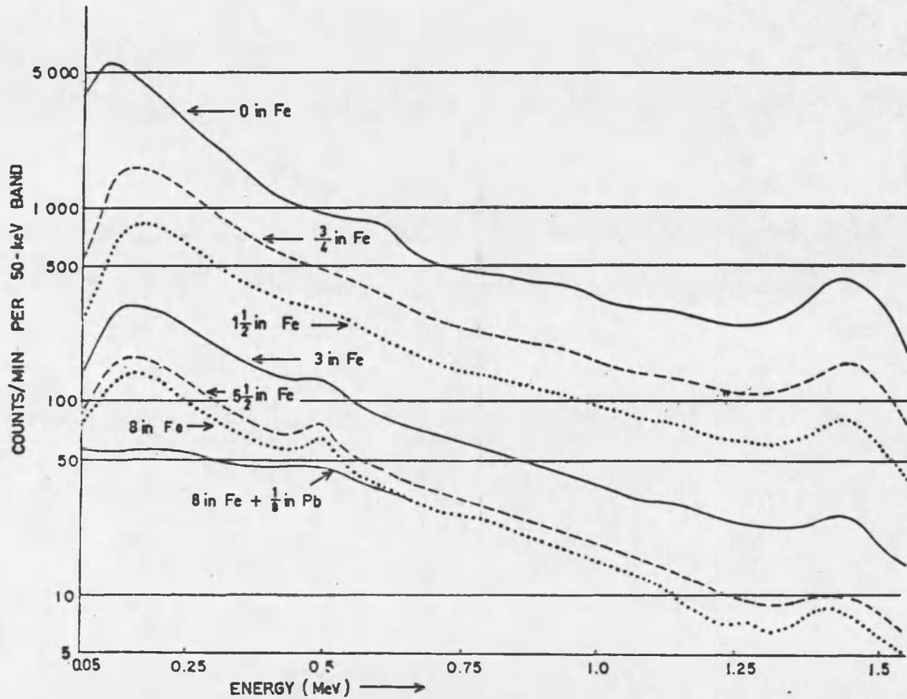
Fig. 14. Reduction in Gamma Ray Background for Various Thicknesses of Iron and Lead. (May and Martinelli 1962)
