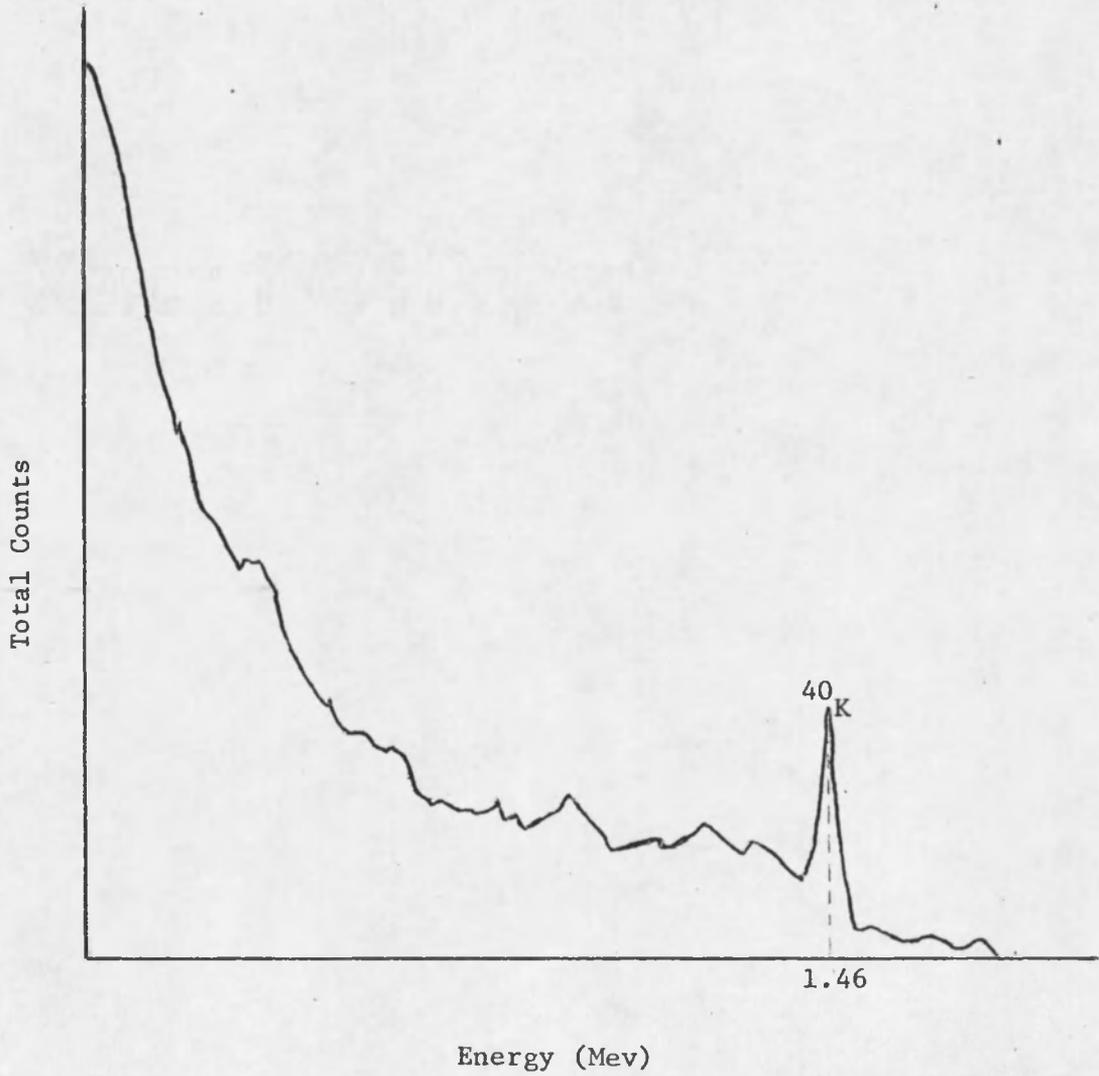
Fig. 12. Background Spectrum in Low Level Counting Laboratory with No Shielding Around Detector
