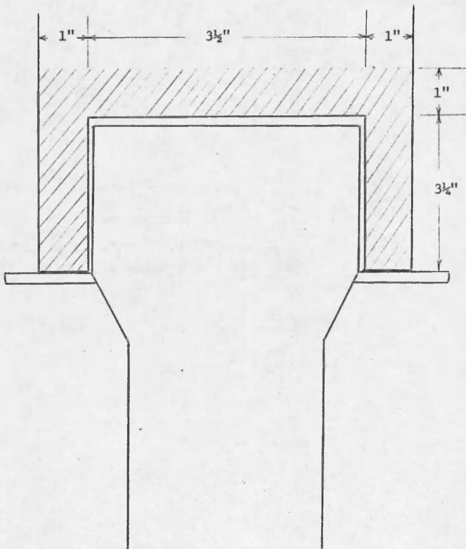
Fig. 20. Reentrant Cup Dimensions
