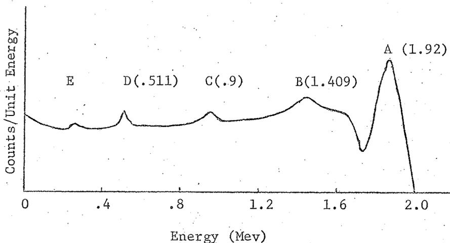
Fig. 8. Pulse Height Distribution for 1.92 Mev Gamma.
