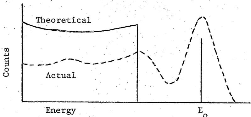
Fig. 7. Theoretical and Actual Energy Distribution for Compton and Photoelectric Interaction in a NaI Detector. (Heath 1964)
