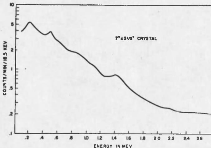
Fig. 13. Background Spectrum in 16-inch Naval Gun Barrel Shield. (May 1962)
