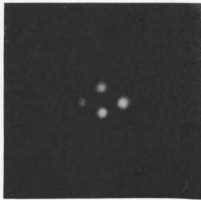
Fig. 5.38. Four-point Axial Object, Distorted FZP on Spherical Surface.
