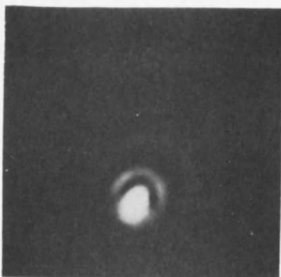
Fig. 5.34. Object Point at x_0 = 0 cm, y_0 = 0.5 cm, Regular FZP on Spherical Surface.
