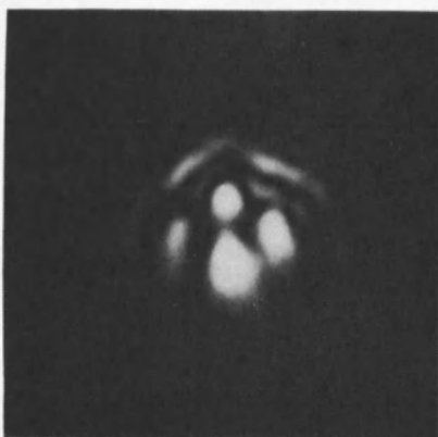
Fig. 5.40. Four-point Object at x_0 = 0 cm, y_0 = 0.5 cm, Distorted FZP on Spherical Surface.
