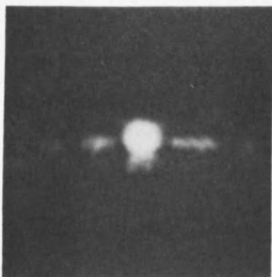
Fig. 5.11. Axial Object Point, Regular FZP on Cylindrical Surface.
