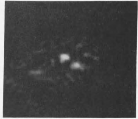
Fig. 5.19. Four-point Object at x_0 = 1.0 cm, y_0 = 0 cm, Distorted FZP #1 on Cylindrical Surface.
