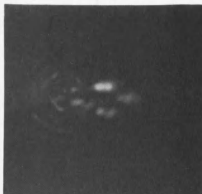
Fig. 5.22. Four-point Object at x_0 = 1.0 cm, y_0 = 0 cm, Distorted FZP #2 on Cylindrical Surface.
