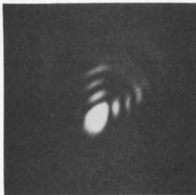
Fig. 5.35. Object Point at x_0 = 0 cm, y_0 = 0.5 cm, Distorted FZP on Spherical Surface.
