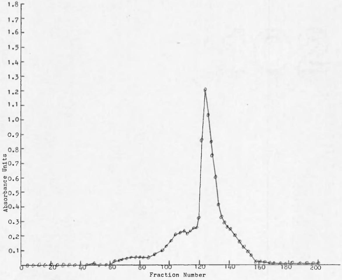
Figure 4. Large Scale SP-Sephadex Ion Exchange Chromatography Using a 0.1 to 0.3 M Sodium Gradient: Optical Density versus Fraction Number.
