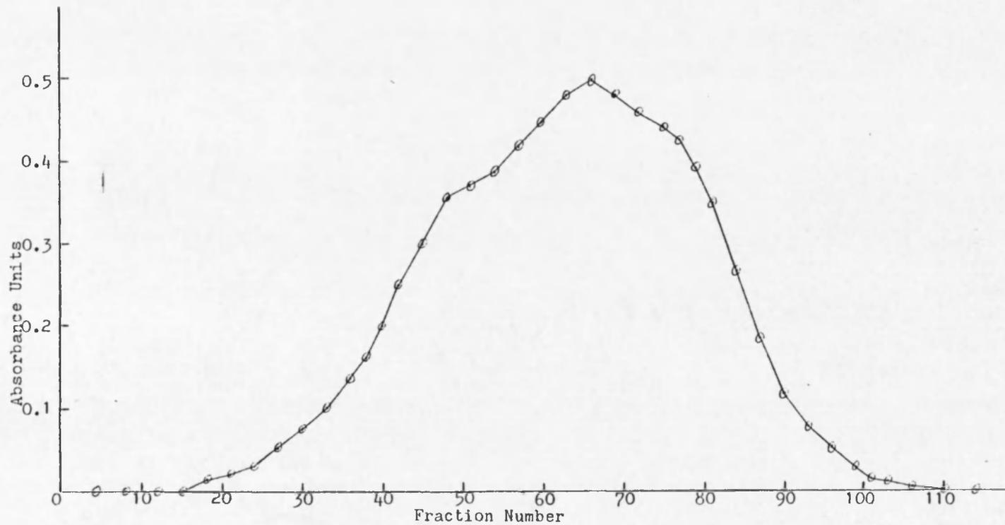
Figure 5. Large Scale SP-Sephadex Ion Exchange Chromatography Using a 0.2 to 0.4 M Sodium Gradient: Optical Density versus Fraction Number.
