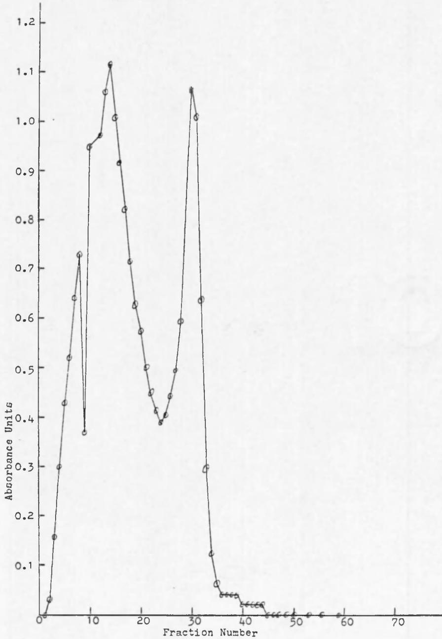
Figure 8. DEAE Sephadex Ion Exchange Chromatography: Optical Density versus Fraction Number.
