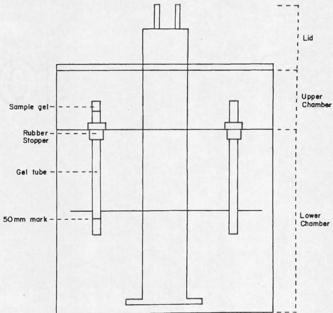
Fig. 3. Electrophoretic Chamber
