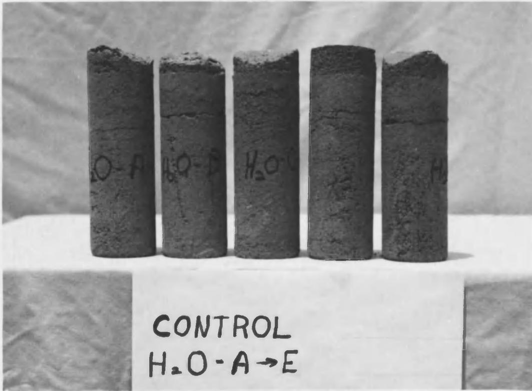
Fig. 2. Cracking patterns in adobe cores after four wetting and drying cycles.
