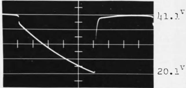
Cathode to Gnd. Voltage of  $V_1$
