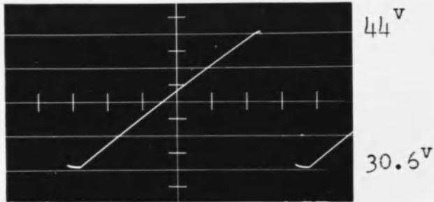
Collector to Gnd. Voltage of  $T_1$
