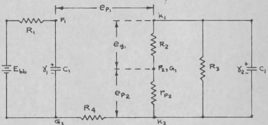
FIG. 2.4 TIMING STATE EQUIVALENT CIRCUIT
