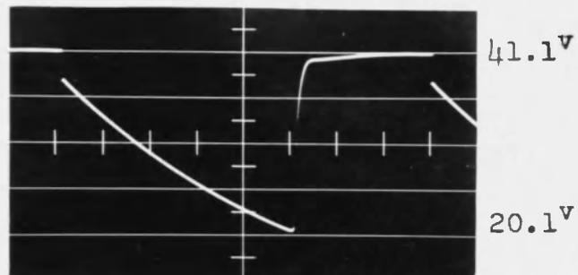
Cathode to Gnd. Voltage of V<sub>1</sub>
