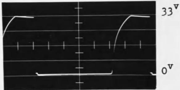
Collector to Gnd. Voltage of  $T_2$
