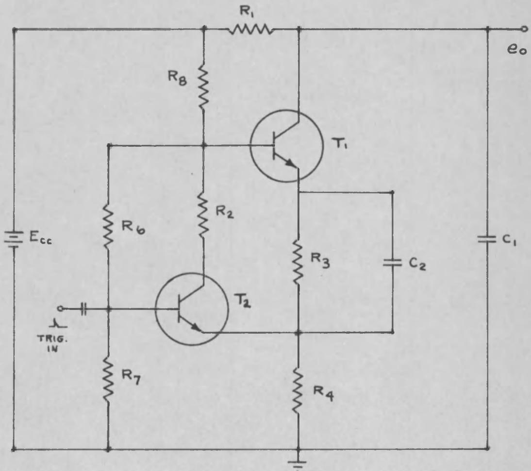
FIG. 3.1 CASCODE SWEEP GENERATOR CIRCUIT
