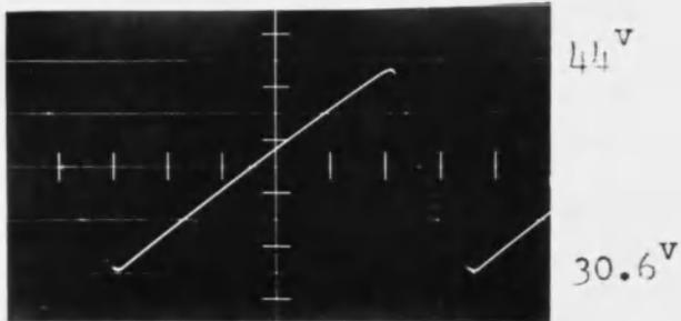
Collector to Gnd. Voltage of  $T_1$
