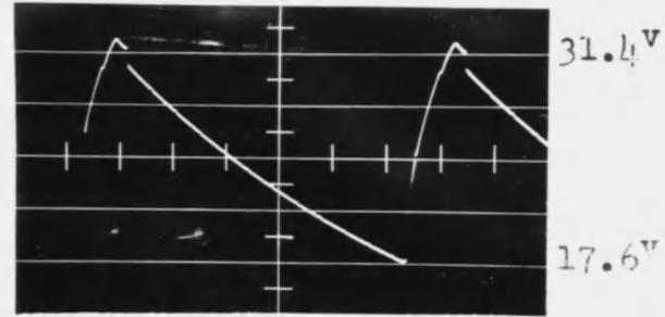
Emitter to Gnd. Voltage of  $T_1$
