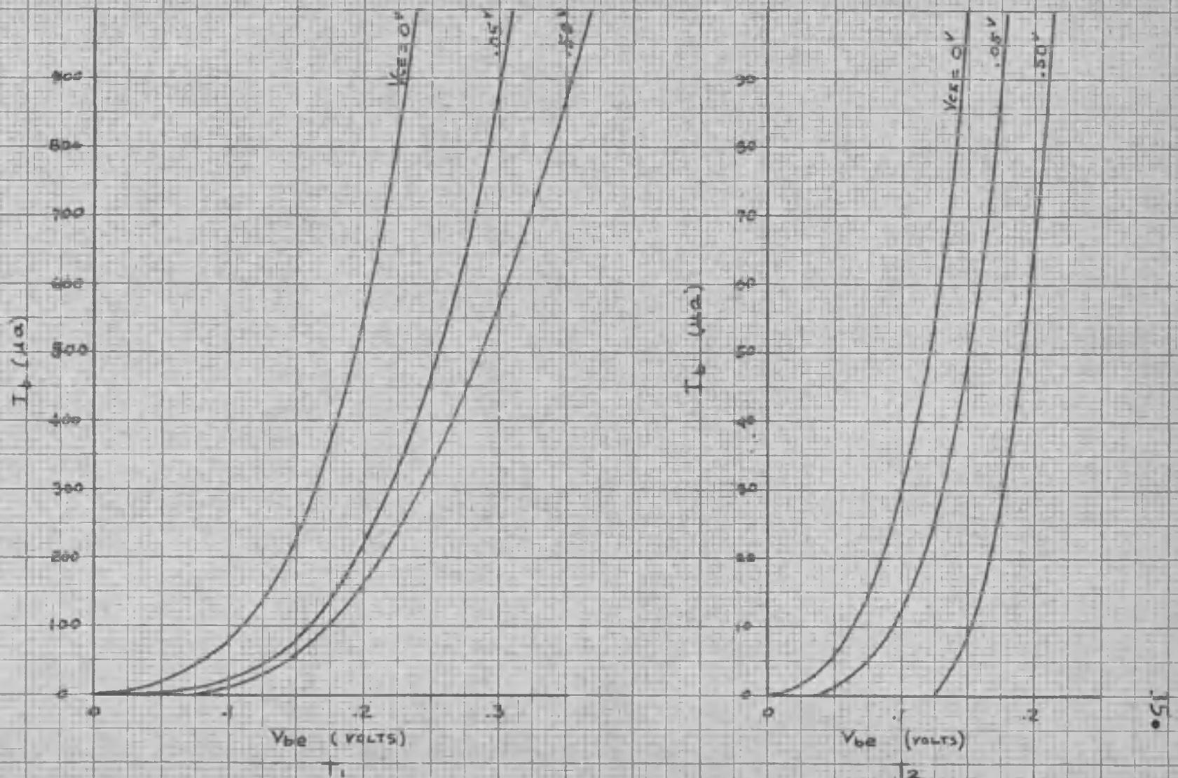
FIG 3 5 INPUT CHARACTERISTICS FOR 2N35 TRANSISTOR
