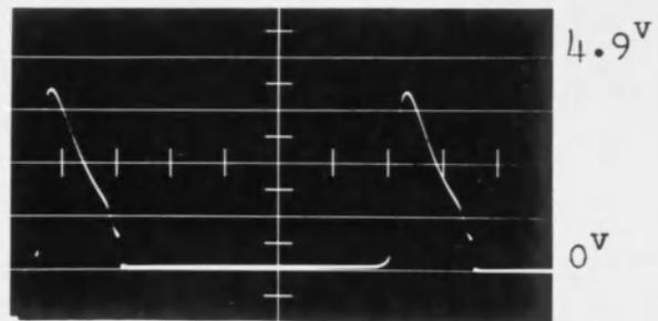
Emitter to Gnd. Voltage of  $T_2$
