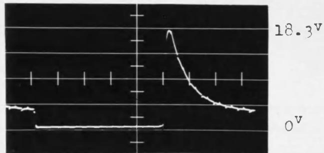
Cathode to Gnd. Voltage of  $V_2$
