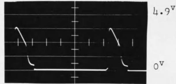
Emitter to Gnd. Voltage of  $T_2$
