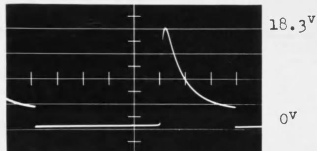
Cathode to Gnd. Voltage of V<sub>2</sub>
