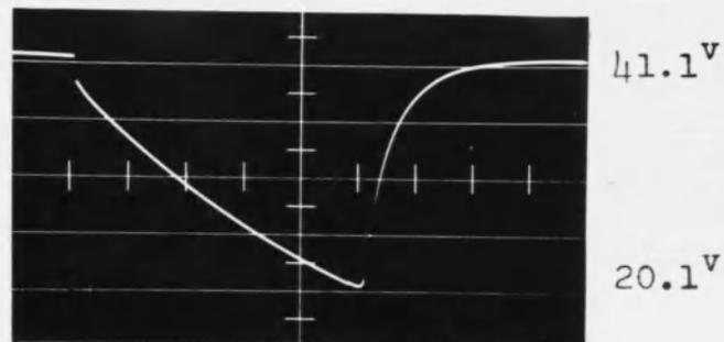
Cathode to Gnd. Voltage of  $V_1$
