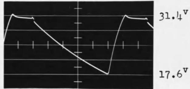
Emitter to Gnd. Voltage of  $T_1$
