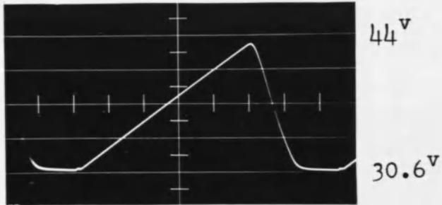
Collector to Gnd. Voltage of  $T_1$
