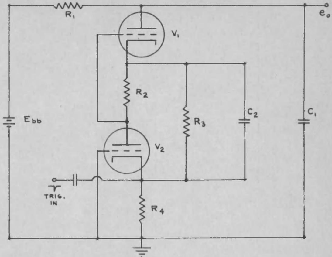
FIG. 2.1 CASCODE SWEEP GENERATOR CIRCUIT
