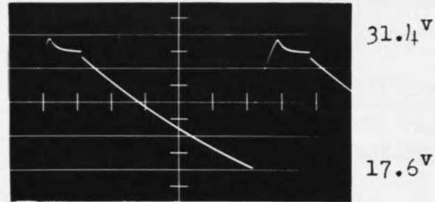
Emitter to Gnd. Voltage of  $T_1$
