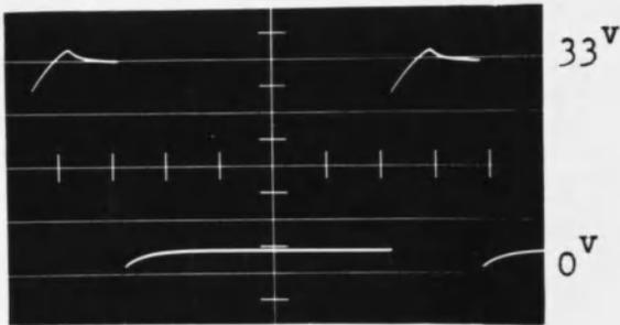
Collector to Gnd. Voltage of  $T_2$
