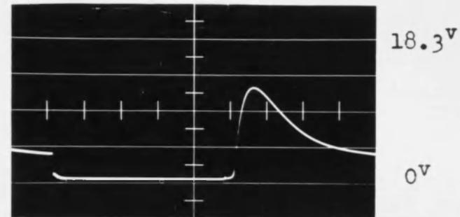
Cathode to Gnd. Voltage of  $V_2$
