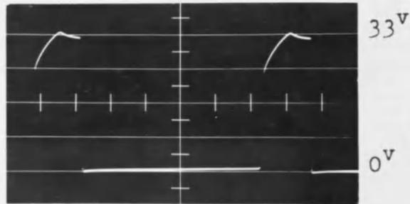
Collector to Gnd. Voltage of  $T_2$
