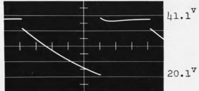
Cathode to Gnd. Voltage of  $V_1$
