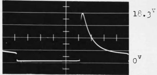
Cathode to Gnd. Voltage of  $V_2$
