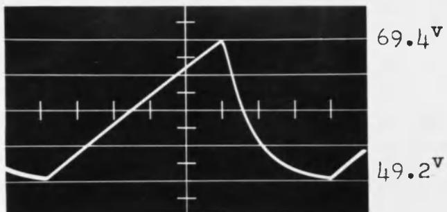
Plate to Gnd. Voltage of V<sub>1</sub>
