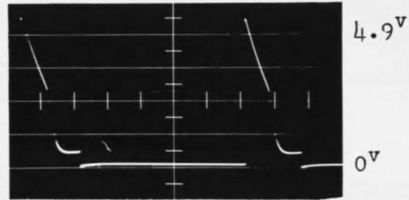
Emitter to Gnd. Voltage of  $T_2$
