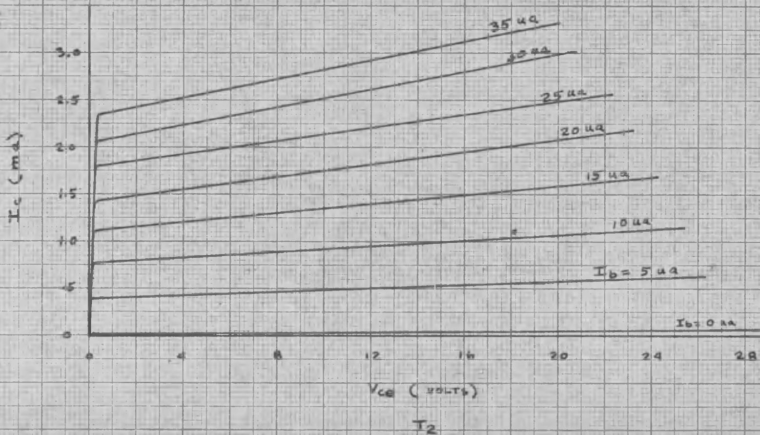
FIG 3.8. OUTPUT CHARACTERISTICS FOR 2N167 TRANSISTOR
