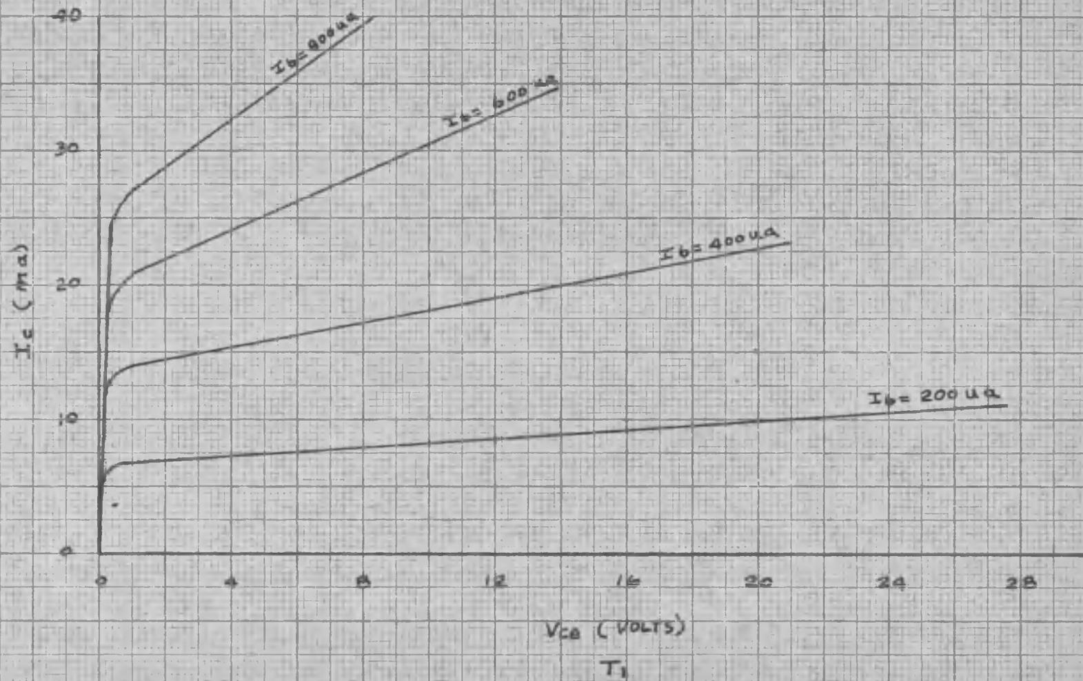
FIG 3.9 OUTPUT CHARACTERISTICS FOR 2N35 TRANSISTOR
