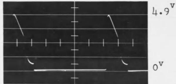
Emitter to Gnd. Voltage of  $T_2$
