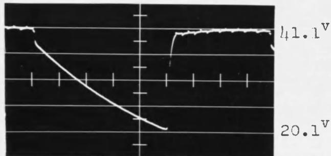
Cathode to Gnd. Voltage of  $V_1$
