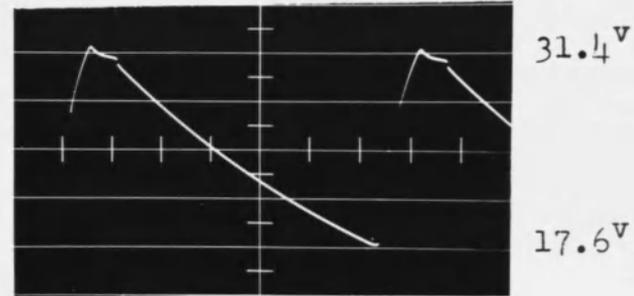
Emitter to Gnd. Voltage of  $T_1$
