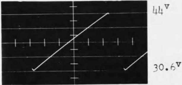
Collector to Gnd. Voltage of  $T_1$
