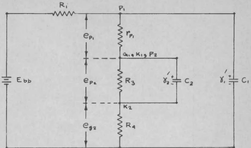
FIG. 2:3 NORMAL STATE EQUIVALENT CIRCUIT
