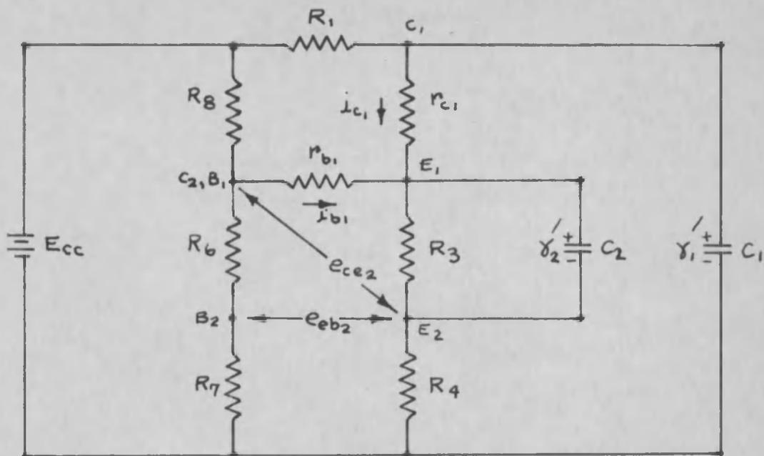
FIG. 3.2 NORMAL STATE EQUIVALENT CIRCUIT
