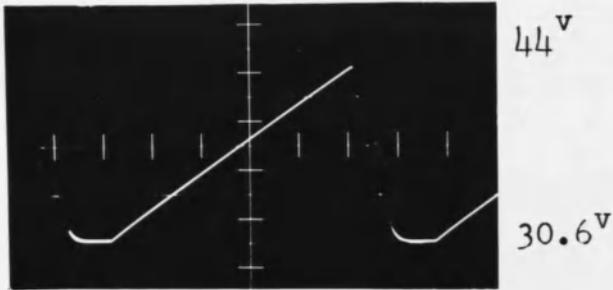
Collector to Gnd. Voltage of  $T_1$
