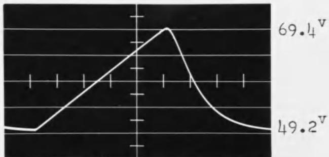
Plate to Gnd. Voltage of  $V_1$
