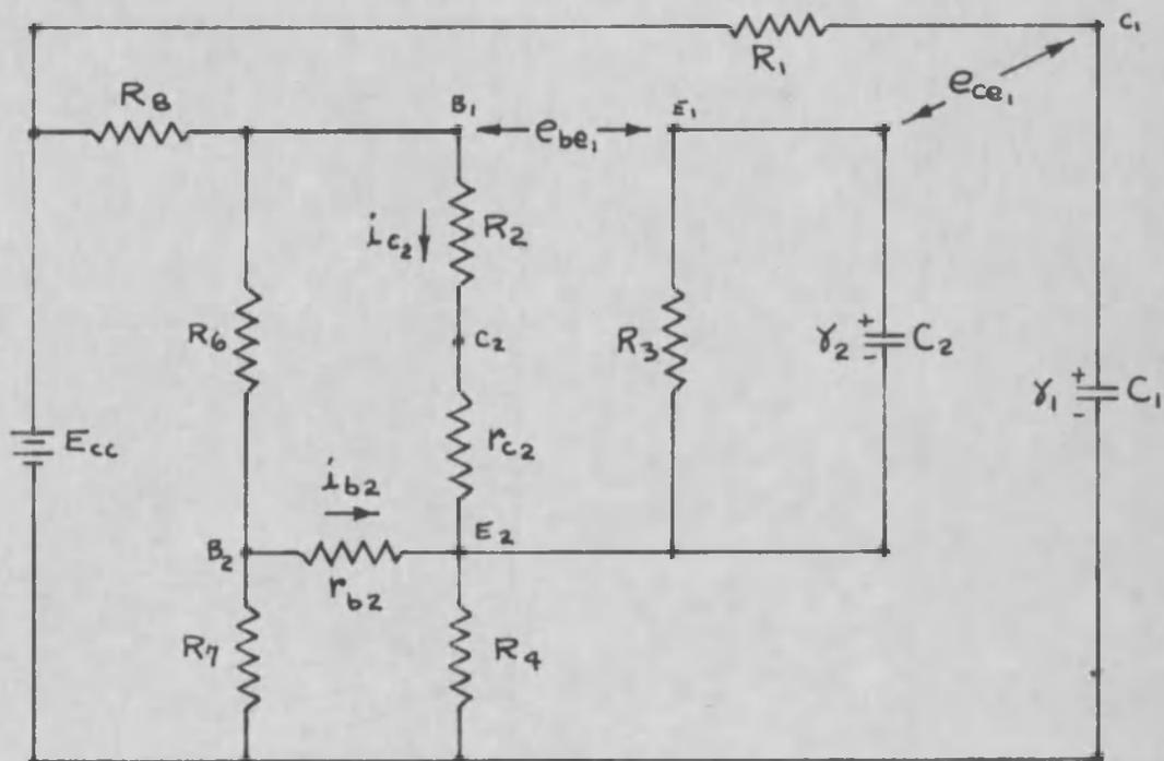
FIG. 3.3 TIMING STATE EQUIVALENT CIRCUIT
