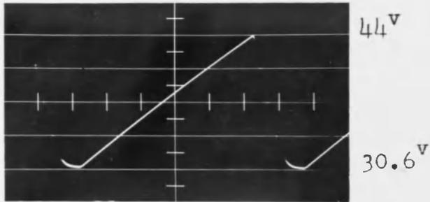
Collector to Gnd. Voltage of  $T_1$
