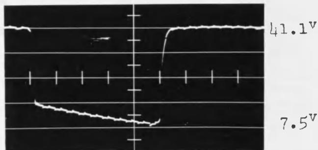
Plate to Gnd. Voltage of  $V_2$
