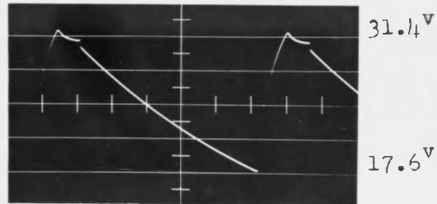
Emitter to Gnd. Voltage of  $T_1$
