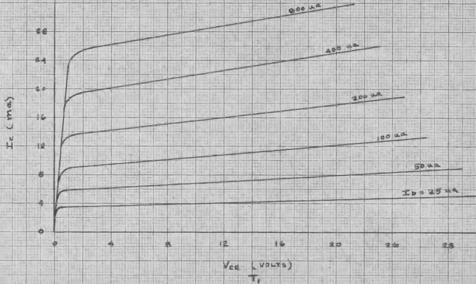
FIG. 3.7 OUTPUT CHARACTERISTICS FOR 2N167 TRANSISTOR
