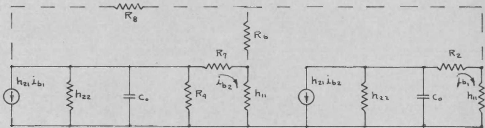
FIG. 3.4 UNSTABLE STATE A.C. EQUIVALENT CIRCUIT
