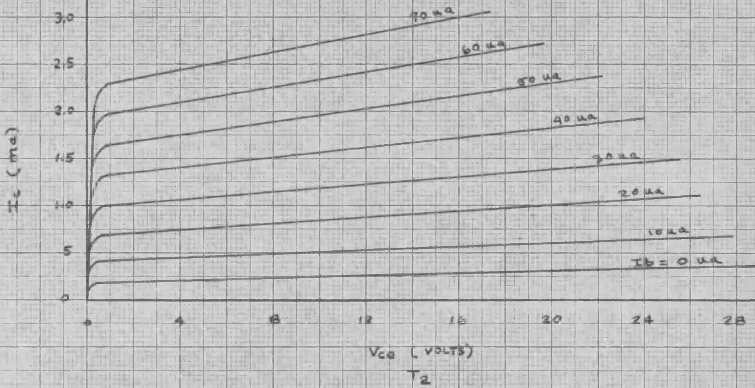
FIG 3.10 OUTPUT CHARACTERISTICS FOR 2N35 TRANSISTOR
