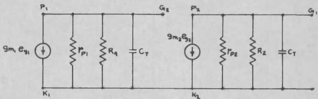
FIG. 2.2 UNSTABLE STATE A.C. EQUIVALENT CIRCUIT
