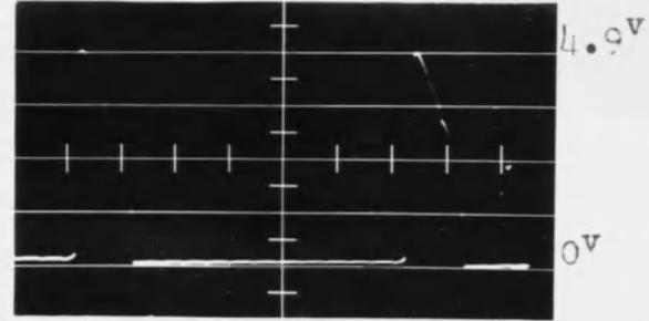
Emitter to Gnd. Voltage of  $T_2$
