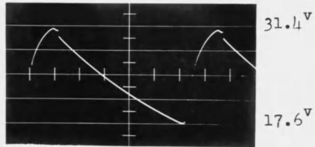
Emitter to Gnd. Voltage of  $T_1$
