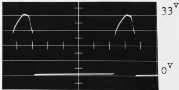
Collector to Gnd. Voltage of  $T_2$
