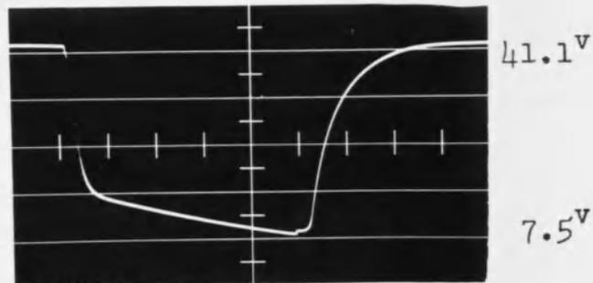
Plate to Gnd. Voltage of  $V_2$
