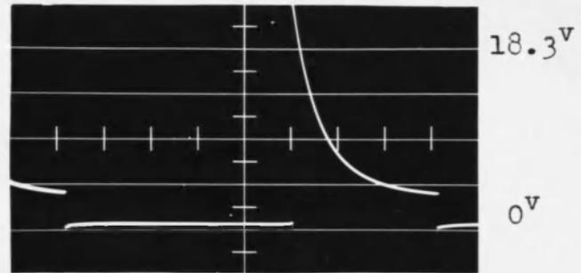
Cathode to Gnd. Voltage of  $V_2$
