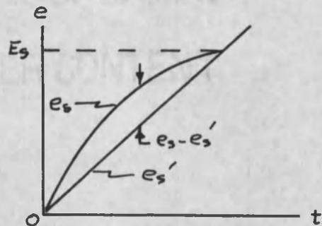
FIG. 2.6 DISPLACEMENT ERROR DEFINITION
