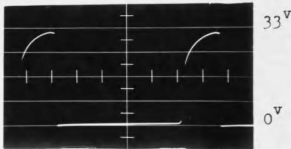
Collector to Gnd. Voltage of  $T_2$
