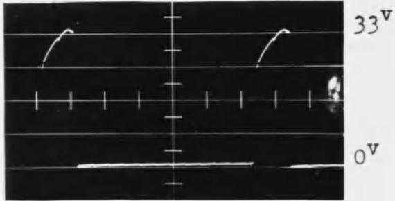
Collector to Gnd. Voltage of  $T_2$
