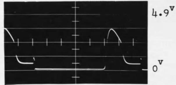
Emitter to Gnd. Voltage of  $T_2$
