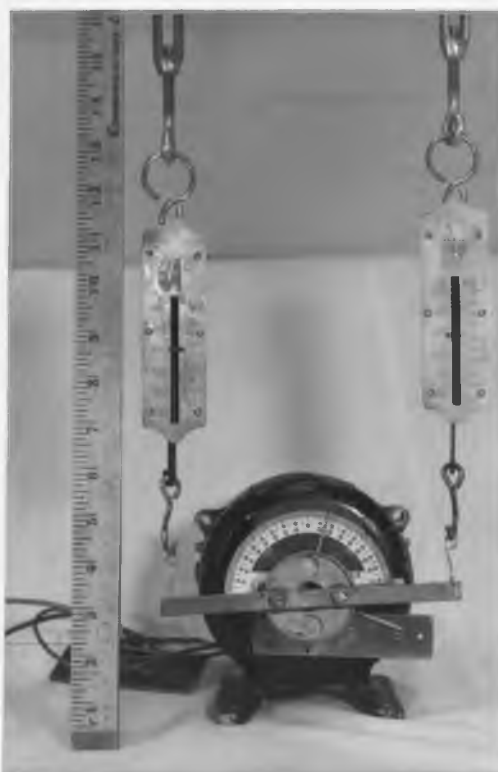
Fig. 3.2 Physical arrangements for measuring torque.
