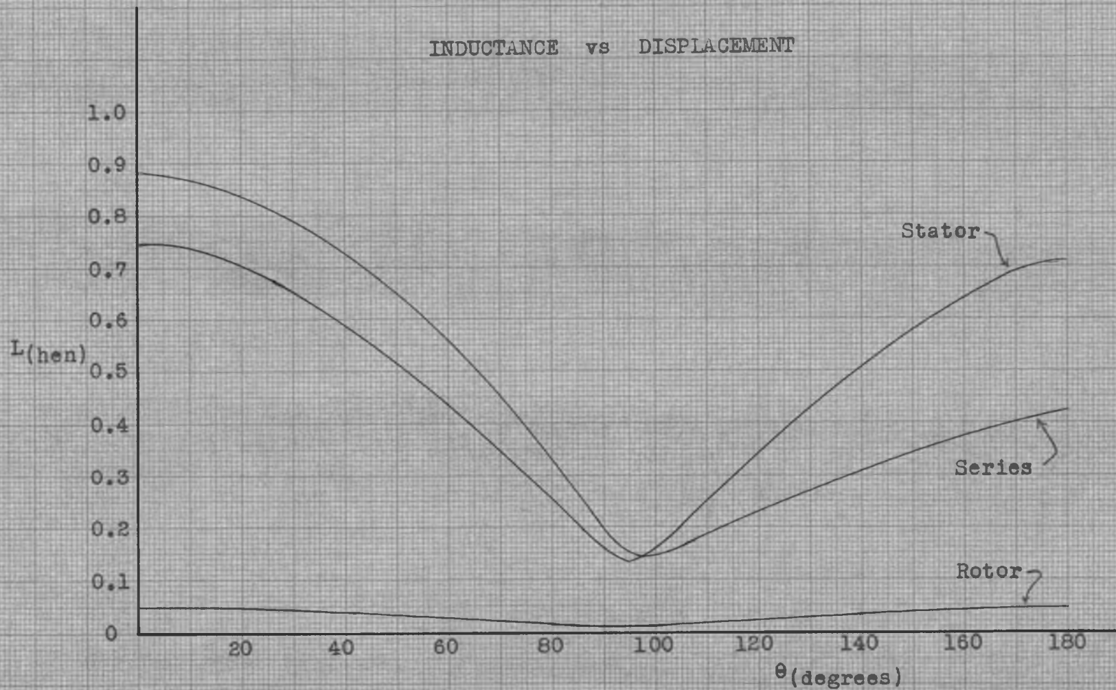
Inductance Curves of Two-Pole-Rotor Electromagnet A-C (60 cycle) Excitation Fig. 3.4
