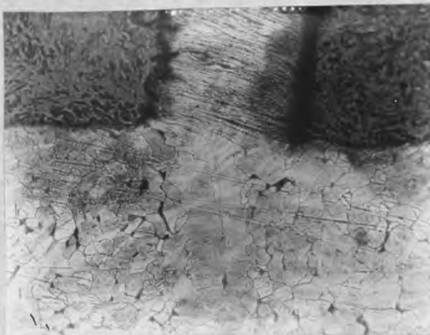
Run 27 - Low Carbon Steel - "As Received" (100x)
