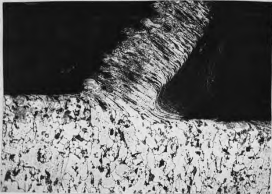
Figure 4.1 Crosssection through chip and work piece (100x)
