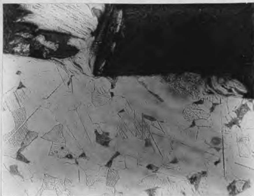
Run 28 - Low Carbon Steel - 1900°F - 4 hr. (100x)
