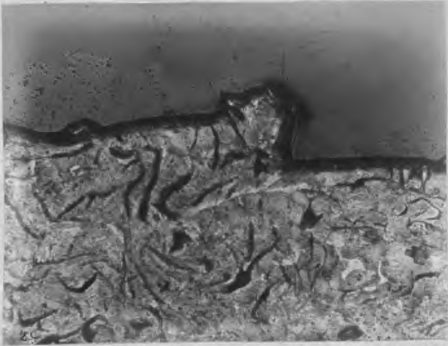
Run 25 - Cast Iron - "As Received" (100x)
