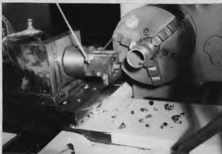
Figure 4.3 Photograph of special tool holder
