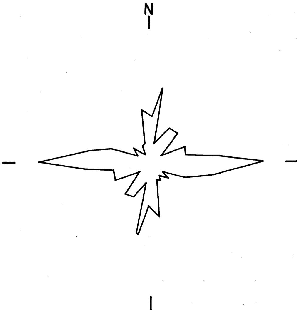
Figure 4.3--Rose diagram showing the orientation of joints in the area studied based on 250 measurements of strike
