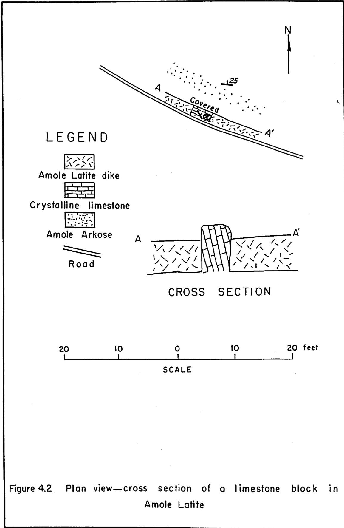
Figure 4.2. Plan view—cross section of a limestone block in Amole Latite
