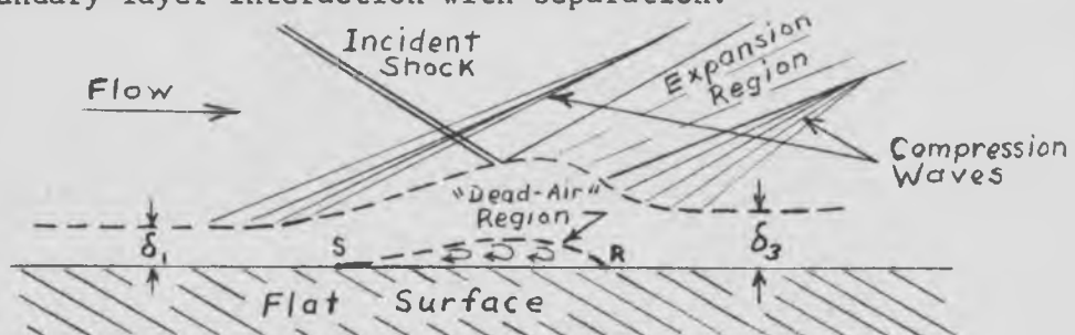
Figure 2.01 Shock Wave-Boundary Layer Interaction With Separation.
