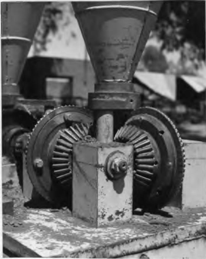
Figure 2. View of compression-type pelleting machine.
