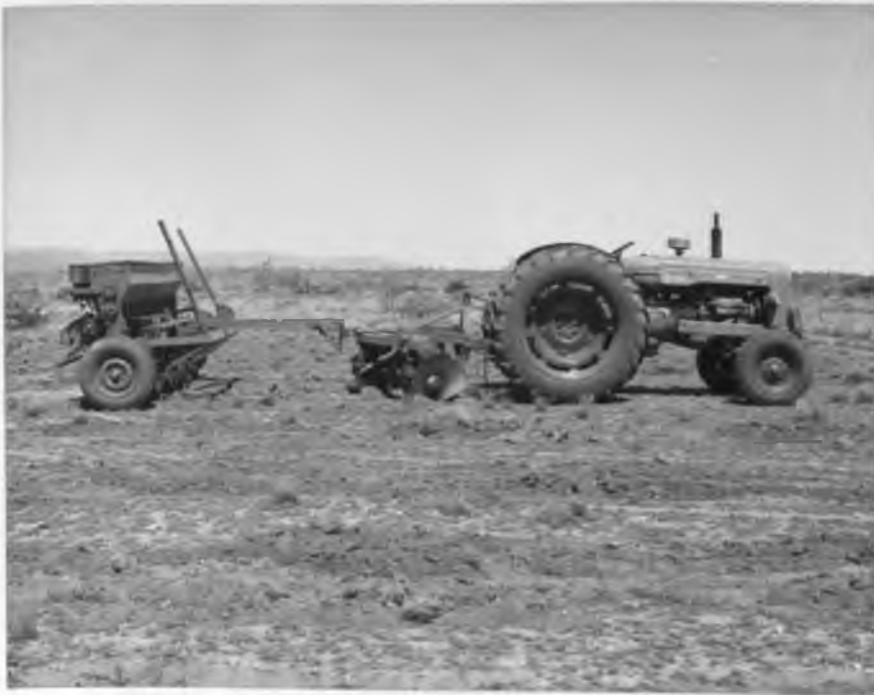
Figure 4. View of cut-away pitting disc (center) and Nisbet grass-seeder (left) used in seedbed preparation and planting.
