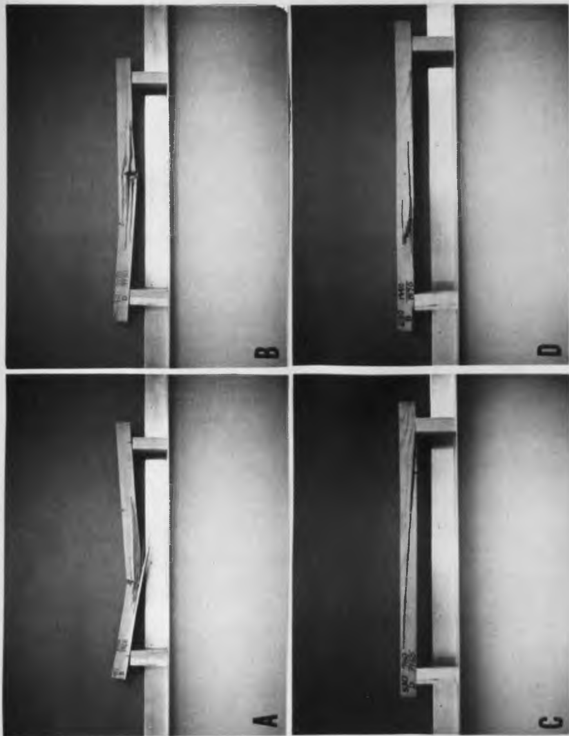
Figure 6. Typical Douglas Fir Failures.
