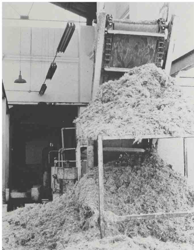
Figure 5. After milling to mechanically break up the heated cabezas, a press separates syrup from waste fiber, bagazo. Here a conveyor belt deposits the bagazo away from the press.
