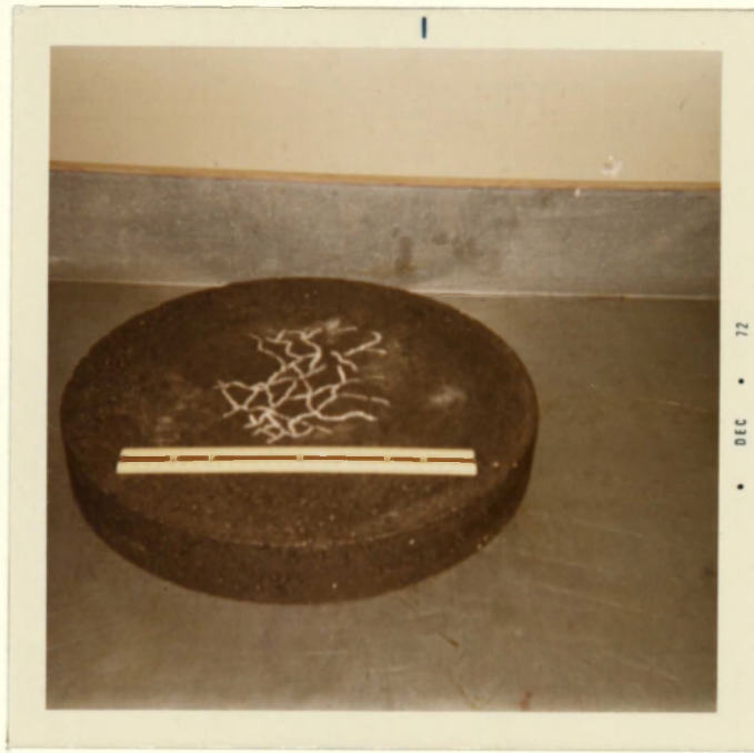
Figure 6. Typical Crack Pattern of a Failed Specimen
