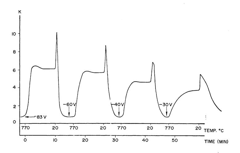
Figure 11. Effect of Various Filament Voltages on Catalytic Oxidation of CO
