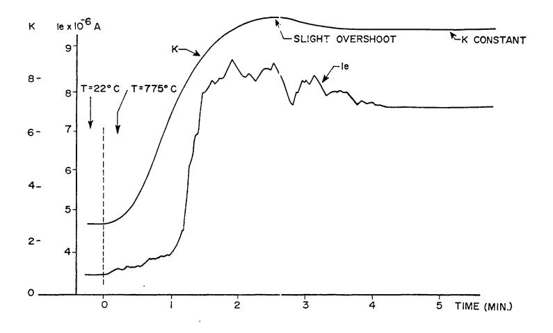
Figure 5. Rate of Reaction and Exo-Electron Emission Versus Time-Oxidation of  ${\rm H_2}$
