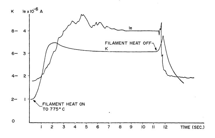
Figure 6. Rate of Reaction and Exo-Electron Emission Versus Time-Oxidation of CO
