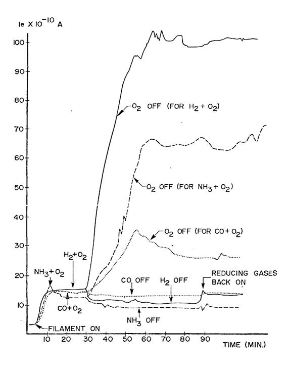
Figure 13. Effect of Removing One of the Reactants on Exo-Electron Emission
