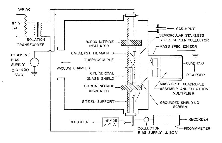
Figure 3. The Reaction Chamber
