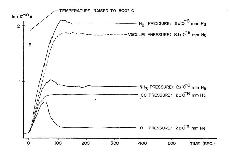
Figure 4. Effect of Various Gases on Exo-Electron Emission from Platinum
