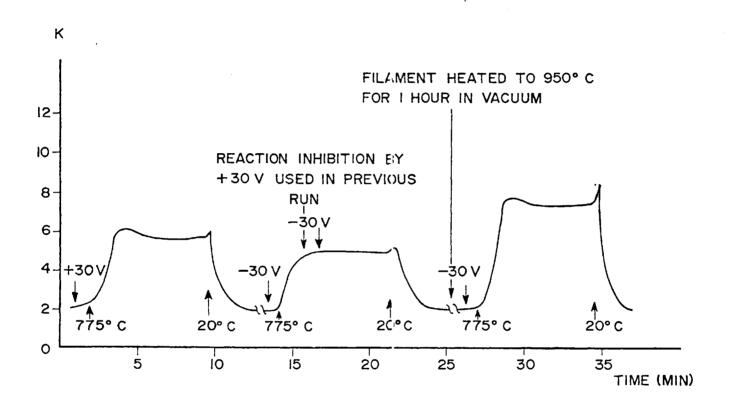
Figure 12. Effect of Previous Exposure to Positive Voltage on Catalysis of CO Oxidation
