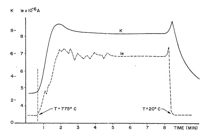
Figure 7. Rate of Reaction and Exo-Electron Emission in Time-Oxidation of  $^{\mathrm{NH}}_{3}$
