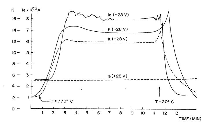
Figure 10. Effect of an External Electric Field on Catalysis of CO Oxidation
