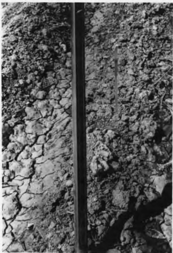
Figure 1. Soil core taken with a "Bull Soil Corer".
