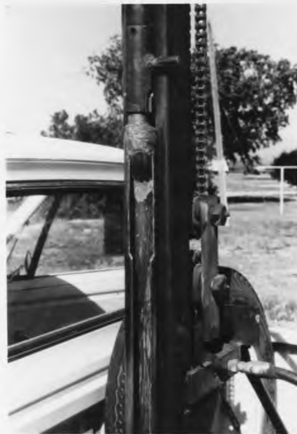
Figure 2. Truck mounted with a "Bull Soil Corer".
