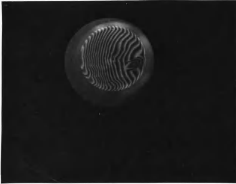
Fig. A.7. Diamond-turned substrate 004, interferogram; two-fringe removal at 3 o'clock; the scallop in the fringes between 6 and 10 o'clock are local dynamic removal areas with voltage change from 2 to 7 volts at 6 o'clock.
