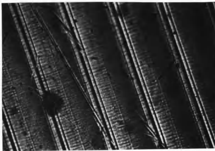
Fig. A.12. Diamond-turned substrate 018, 2.2 \mu material removal, some attack and burn spots, 40 X objective.
