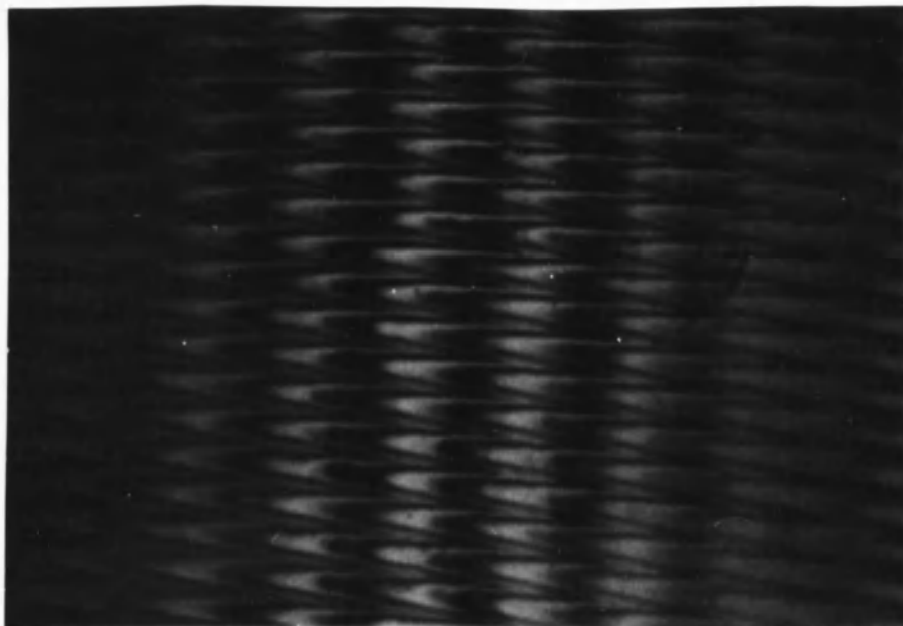
Fig. A.14. Diamond-turned substrate 018, microinterferogram 2.2 \mu material removal, large unique turnings are evident, 10 X objective.
