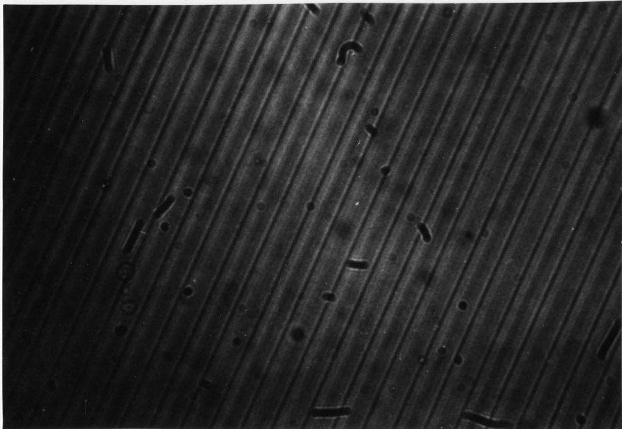
Fig. A.4. Diamond-turned substrate 004, untouched area, 40 X objective.
