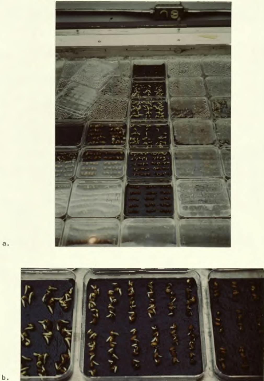
Fig. 4. Thermogradient plate shown with cover removed. -- (a) Seeds shown in the center column are Macroptilium atropurpureum ; (b) Closeup of center of Fig. 4a.
