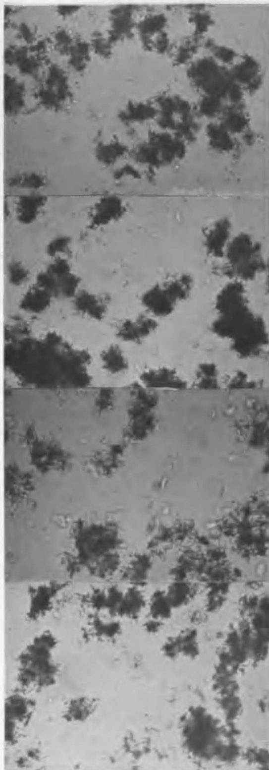
Figure 28. Crystals grown in high citric acid concentrations ((50 ppm to 250 ppm)).
