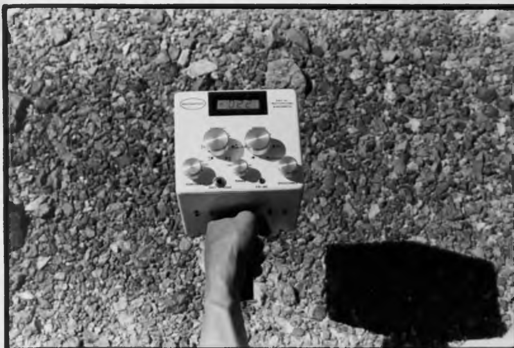
Figure 36. Radiometrics RMR-10 multispectral radiometer shown in field operation.
