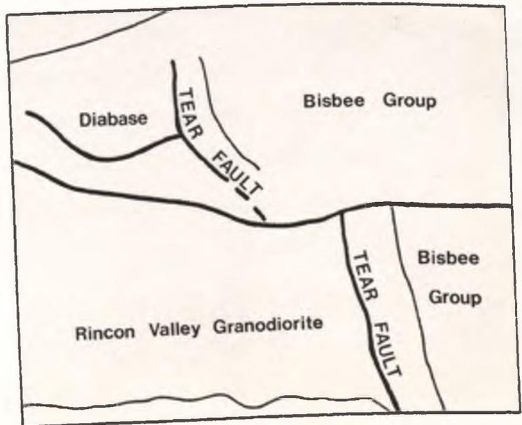
North of Bolsa Hill, the Tear Fault is truncated by a northwest striking, southwest side down normal fault. Any further northeast extension of the Tear Fault was not visible, and may lie under the upper detachment.
