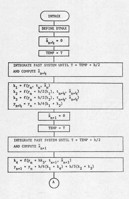
Figure 4. Flow chart of general nonlinear algorithm with averaging
