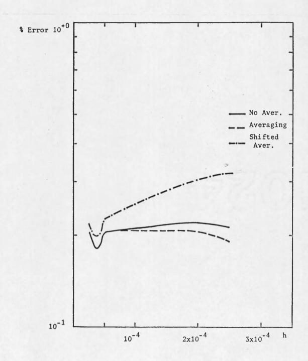
Figure 25. Peak error in  $X_2$  vs. h. Autopilot (partition 2)
