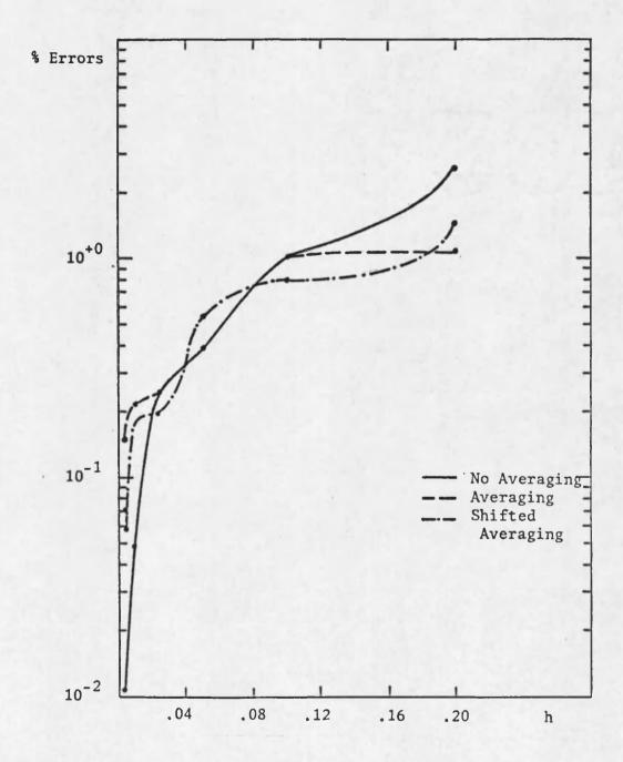
Figure 18. Peak error in  $X_2$  vs. h. Oscillator (partition B)
