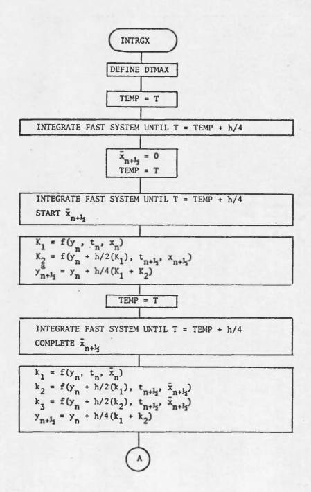
Figure 5. Flow chart of subroutine INTRGX of general nonlinear algorithm with shifted averaging
