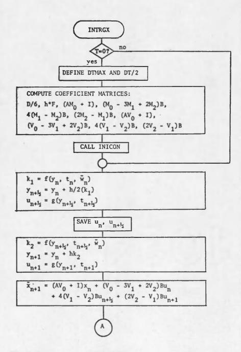
Figure 3. Flow chart of INTRGX for Modified Euler method
