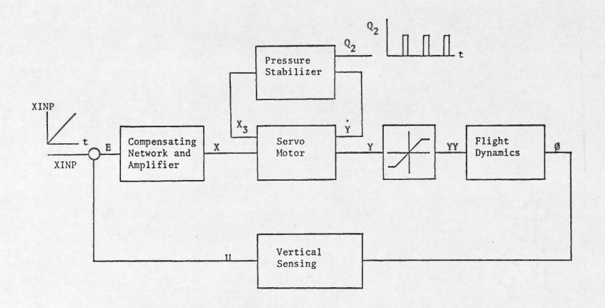
Figure 6. Block diagram of autopilot system
