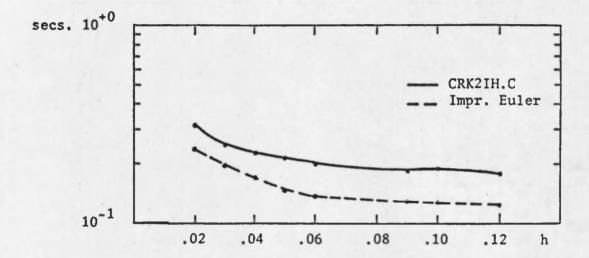
Figure 13. Execution times vs. h. Mine-shaft
