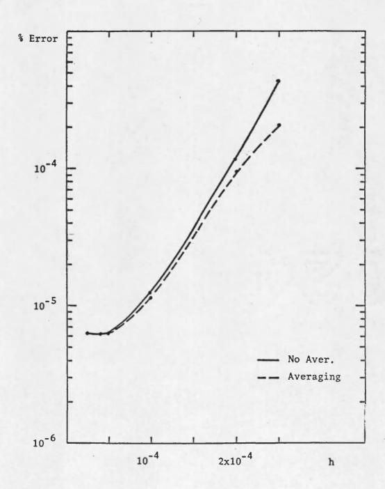
Figure 21. Peak error in  $X_2$  vs. h. Autopilot (partition 1)
