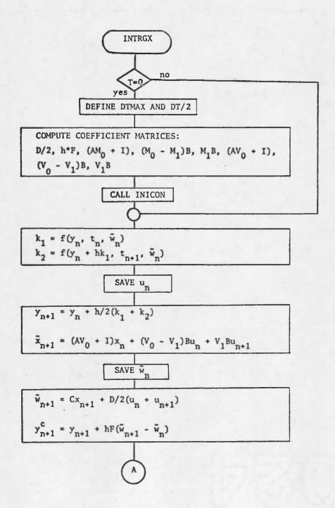
Figure 2. Flow chart of subroutine INTRGX for Improved Euler method
