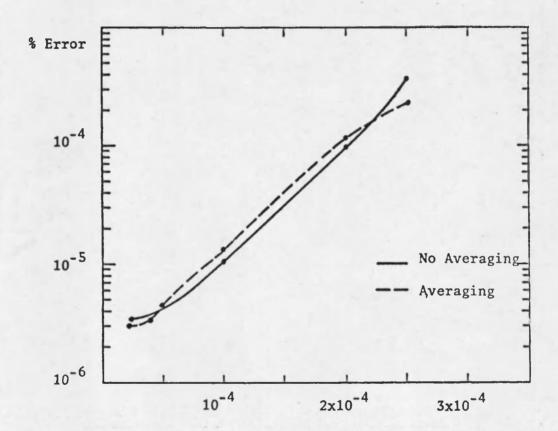
Figure 20. Mean peak error vs. h. Autopilot (partition 1)
