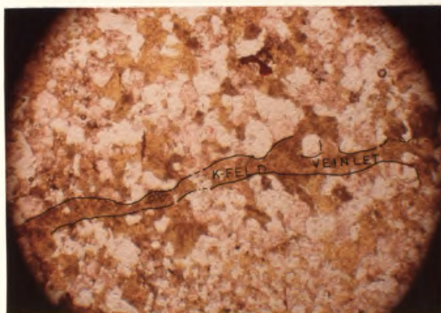
Figure 16. Photomicrograph showing a veinlet of secondary orthoclase in aplite, southern part of Sierrita intrusion, Arizona
