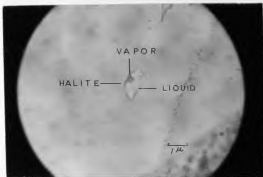
Figure 38. Fluid inclusion with a halite daughter mineral Boulder batholith, Montana, thin section 21.
