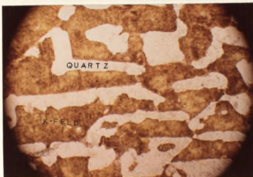
Figure 15. Photomicrograph showing graphic texture in a pegmatite dike, southern part of Sierrita intrusion, Arizona
