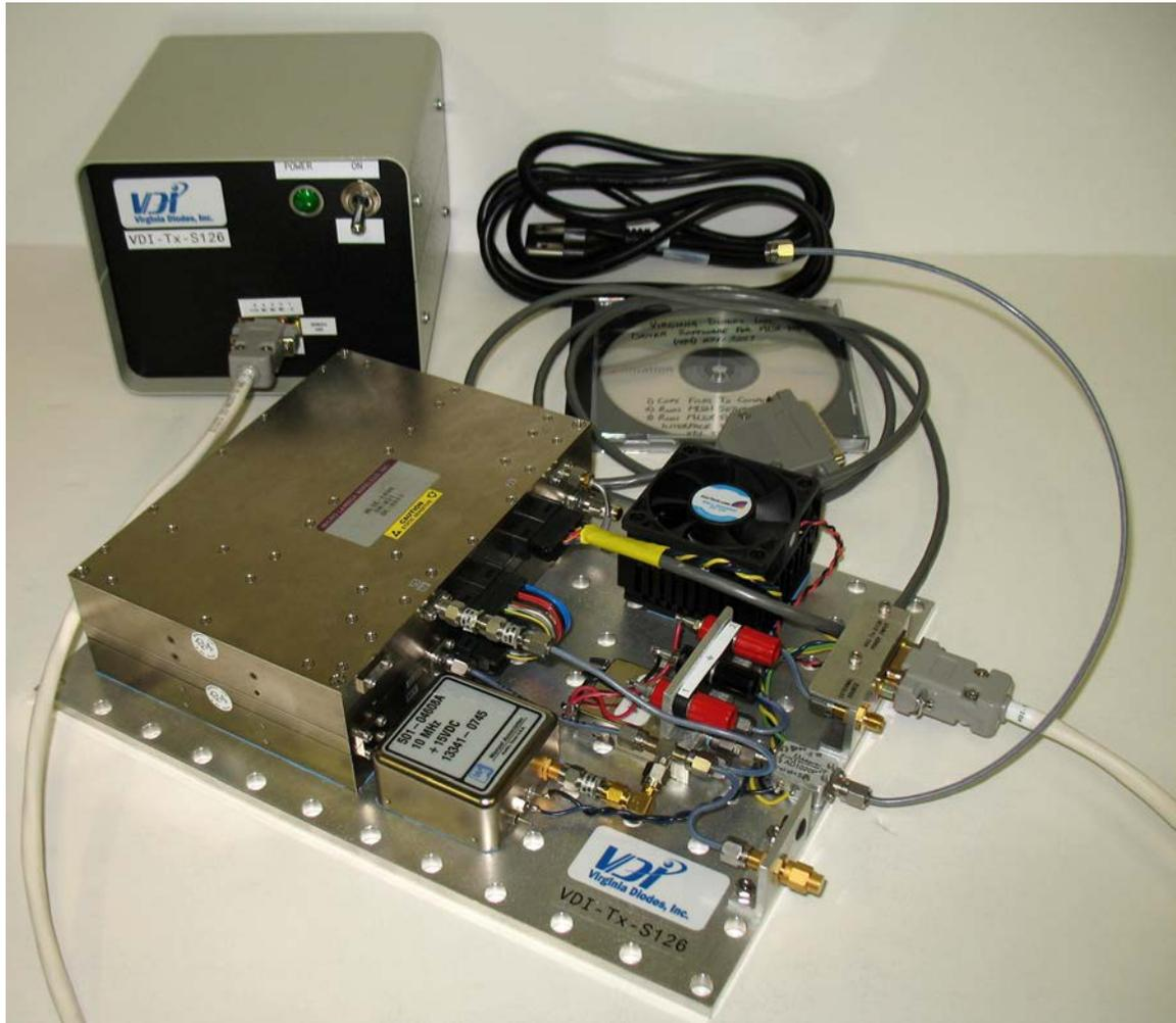
**Figure 7: The 20-40 GHz Synthesizer-Driver-Transmitter (courtesy of Virginia Diodes, Inc.)**
