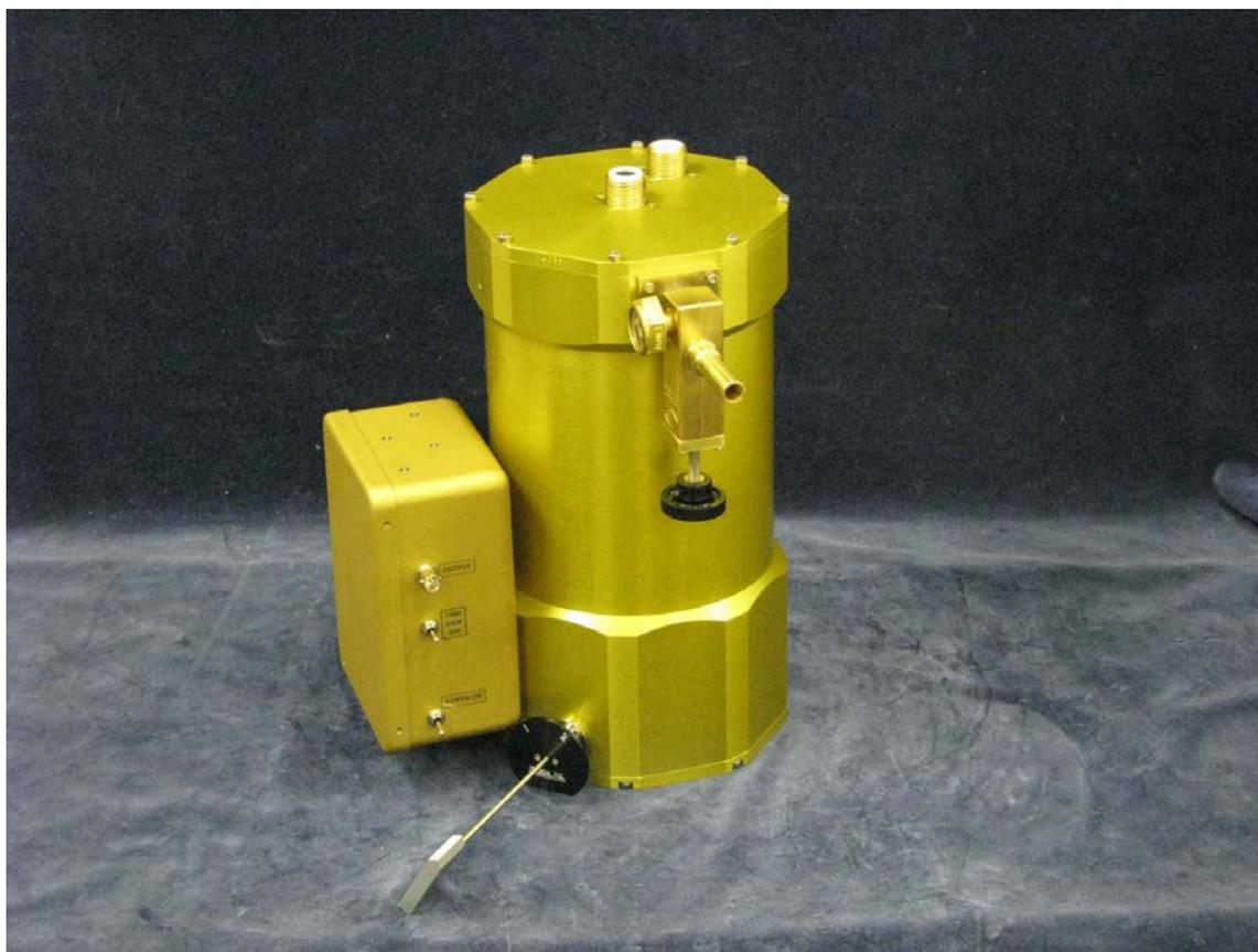
External view of IR Labs Silicon Bolometer Dewar Assembly (Courtesy IR Labs, Tucson, AZ)
