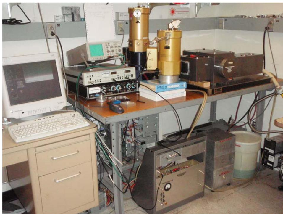
**Figure 32 FTS System Photo with Cooled Silicon Bolometer Detector**
