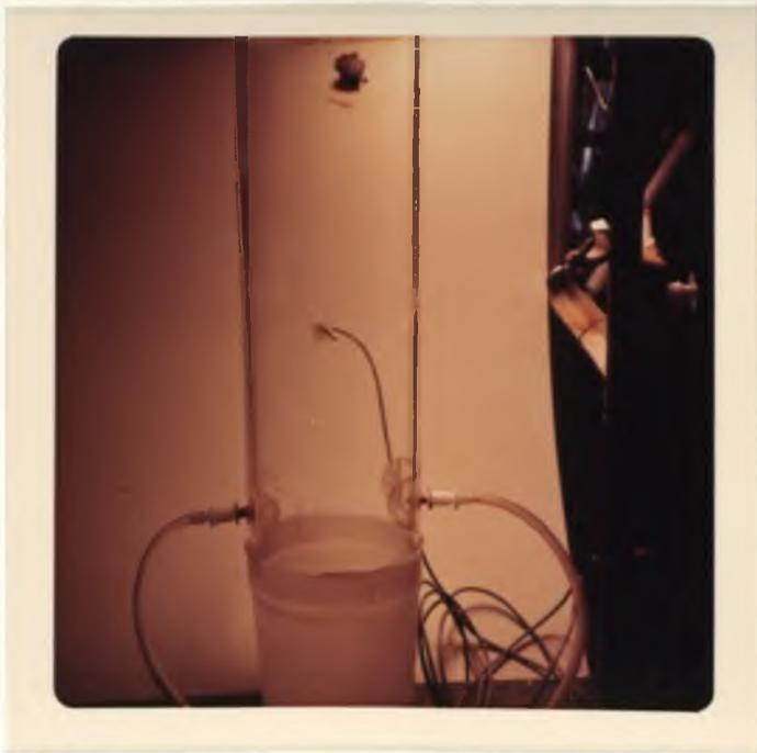
Figure 1. Plexiglass chamber used to measure photosynthesis in Experiments 1 and 2.
